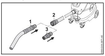
► Push hand tube (1) or adapter (3) into the sleeve (2). The hand tube (1) or adapter (3) engages audibly.
