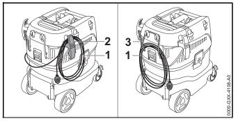
► Roll up the connecting cord (1) and hang it on the holder (2) or secure with rubber strap (3).
