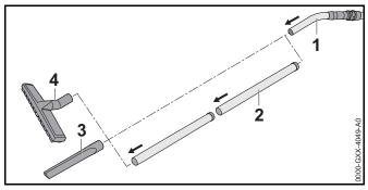
► Push the hand tube (1) into the suction tube (2), floor tool (4), crevice tool (3) or other accessory.
