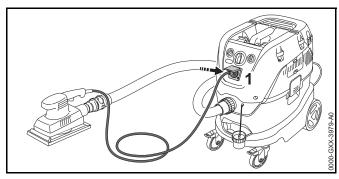
Plug mains plug (1) of the electric power tool into the socket.
