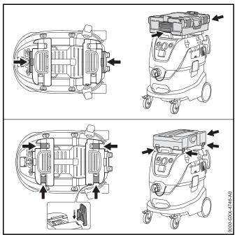
► Put the tool box on top and lock it in place.
