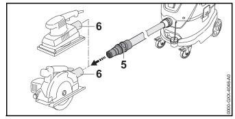
► If connecting an electric power tool: Push adapter (5) onto suction connector of electric power tool (6).
