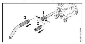
Squeeze sleeve (1) and pull off hand tube (3) or adapter (2).
