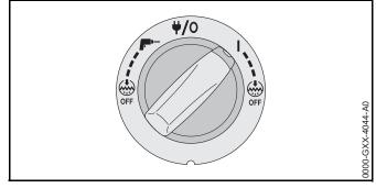
► Turn the rotary switch to the I position.
