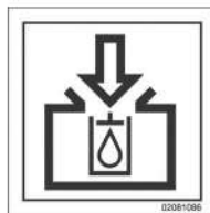
Hydraulic oil reservoir inlet
