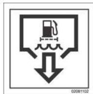
Water sump fuel filter outlet
