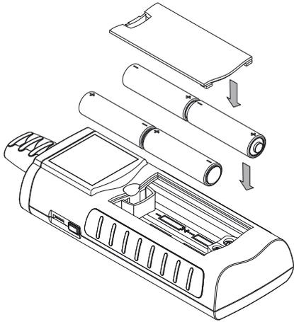
1. Open the cover of the battery compartment (3).
