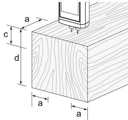
2. Insert the measuring tips transverse to the fibre direction with a 30 cm distance to one of the two ends of the sawn timber.
