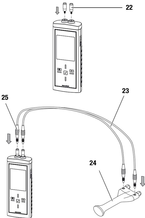
1. Detach the nuts and remove the measuring tips, if applicable.
