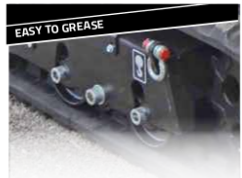
EASY TO GREASE Greasing the undercarriage is easy and fast: nothing has to be taken apart.
