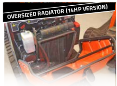
OVERSIZED RADIATOR (14HP VERSION) The air/water cooling system allows the machine to operate in extreme conditions
