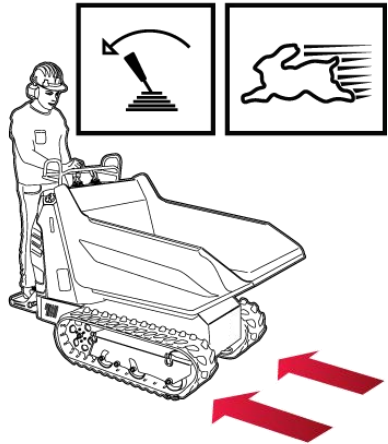
fig. 23 – Forward (top) - Reverse (bottom) "speed"
