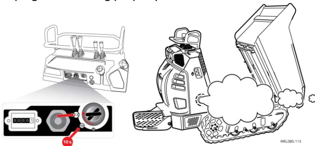
fig. 41 – Verification of plugs preheating system
