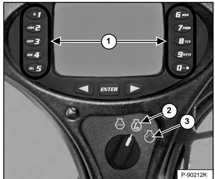
Turn the key switch to RUN (Item 2) [Figure 125]. The indicator lights on the left instrument panel will come ON briefly and the instrument panel / monitoring system will perform a self test.
