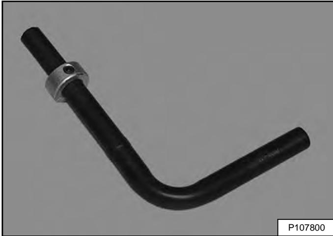
A bleed tool [Figure 253] is available and recommended to decrease track tension. The bleed tool will direct the flow of grease to aid in cleanup. See your Bobcat dealer to order a bleed tool.
