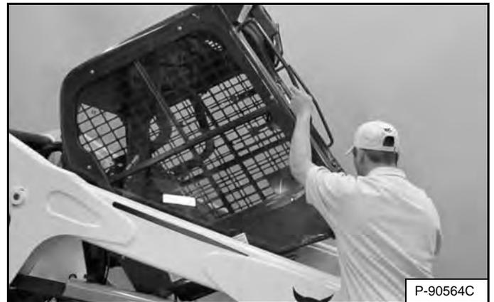
Lift on the grab handles and bottom of the operator cab [Figure 182] slowly until the operator cab is all the way up and the latching mechanism engages.
