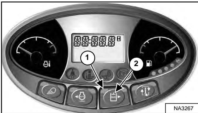
Press the Auxiliary Hydraulics button (Item 2) [Figure 85] once to activate the auxiliary hydraulics.
