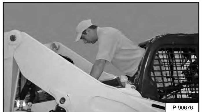
Exit through the rear of the operator cab [Figure 44].
