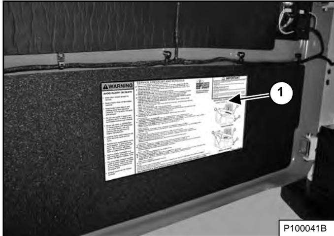
The Service Checklist And Schedule (Item 1) [Figure 103] is located inside the rear door of the loader.
