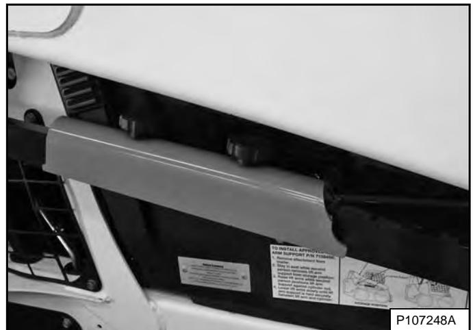
Return the lift arm support device to the storage position and secure with clamping knobs **[Figure 173]**.
