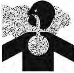
Cutting or drilling concrete containing sand or rock containing quartz may result in exposure to silica dust. Use a respirator, water spray or other means to control dust.
