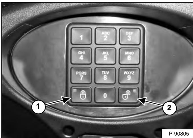
Press and hold the lock (Item 1) and unlock (Item 2) [Figure 313] keys for 2 seconds.
