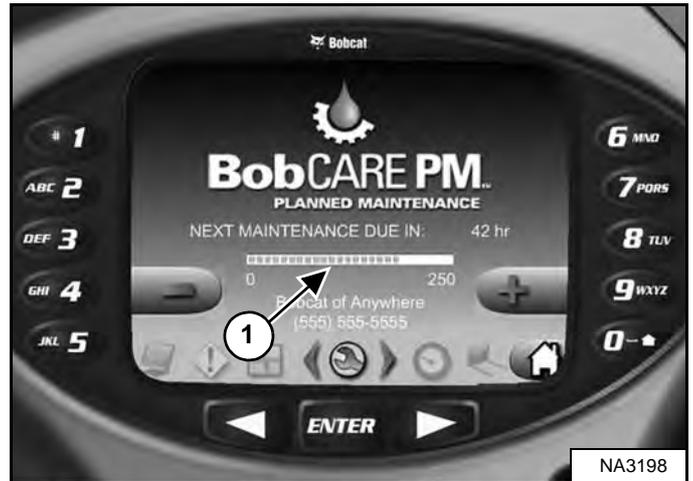
The Deluxe Instrumentation Panel (if equipped) will display a bar (Item 1) [Figure 316] showing the time remaining until next service. This bar will turn red when service is past due. [NEXT MAINTENANCE DUE] will change to [MAINTENANCE PAST DUE] and display the number of hours past due.
