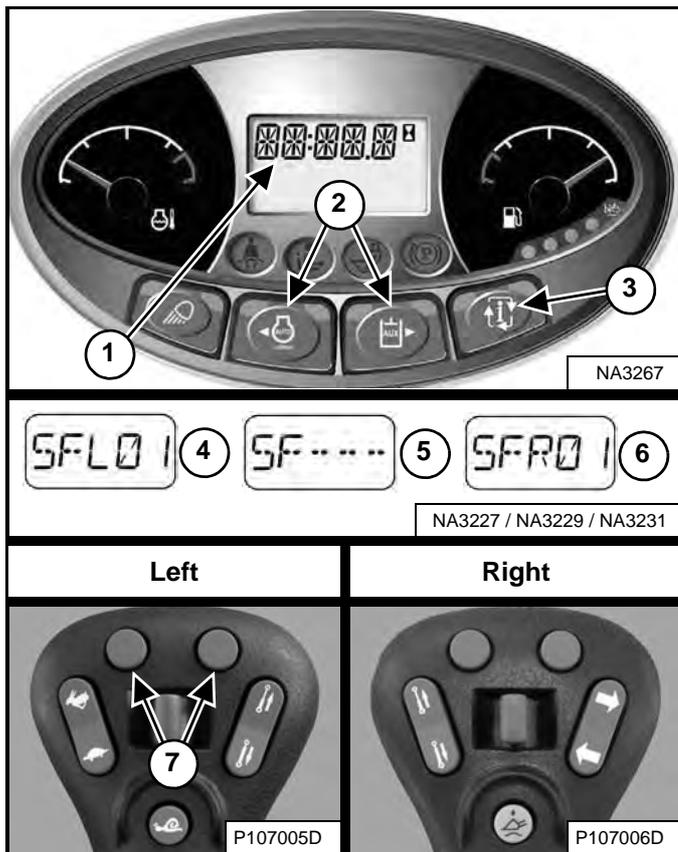
Press the Information button (Item 3) to cycle the data display until the steering drift compensation menu is displayed. The current steering drift compensation setting will appear in the data display (Item 1) [Figure 71].
