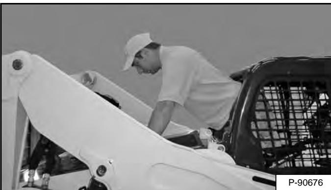
Exit through the rear of the operator cab [Figure 42].
