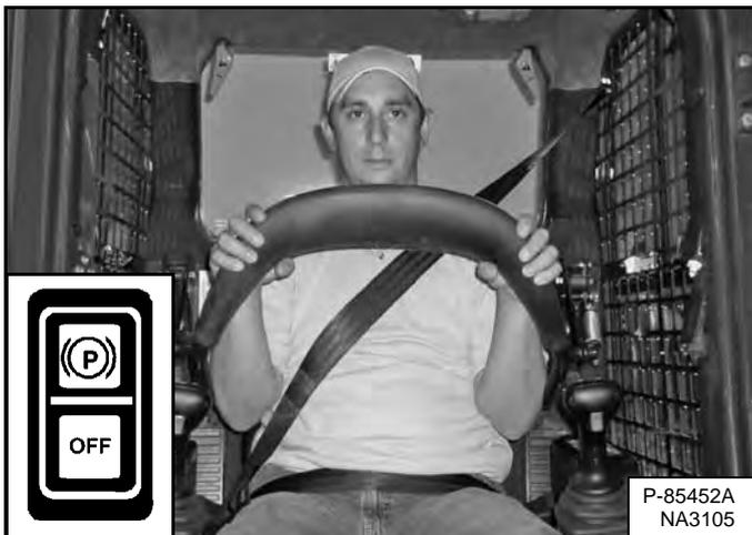
Lower the seat bar and engage the parking brake [Figure 112].
