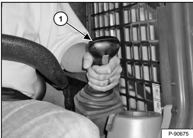
The joystick that controls drive and steering is on the left side in front of the seat (Item 1) [Figure 57].
