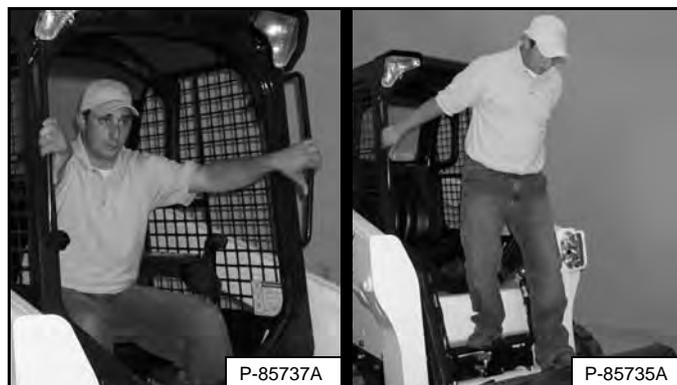
Exit the loader using grab handles, safety tread, and steps (maintaining a three-point contact) [Figure 132].
