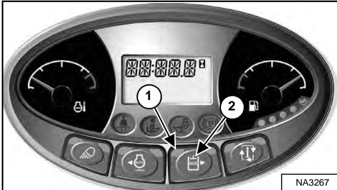
Press the Auxiliary Hydraulics button (Item 2) [Figure 90] once to activate the auxiliary hydraulics.
