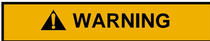
The signal word **WARNING** on the machine and in the manuals indicates a potentially hazardous situation which, if not avoided, could result in death or serious injury.
