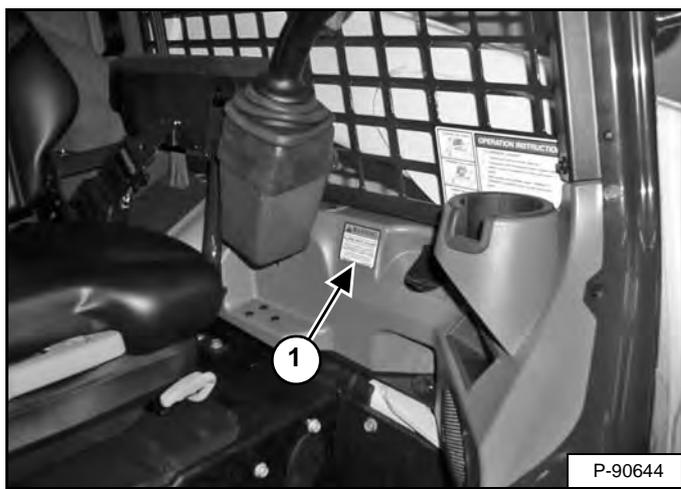
Inspect for damaged or missing back-up alarm decal (Item 1) [Figure 174]. Replace if required.
