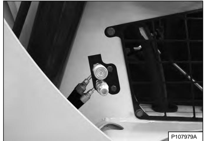
Move the Rear Auxiliary Hydraulic switch (Item 1) [Figure 91] or [Figure 92] to the right or left to change direction of the auxiliary hydraulic fluid flow to the rear quick couplers [Figure 93]. (EXAMPLE: Raise and lower rear stabilisers.) Release the switch to stop fluid flow.
