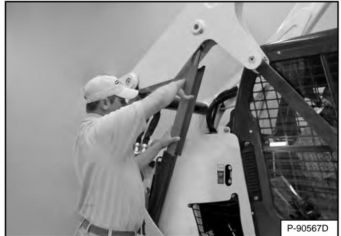
Have a second person install the lift arm support device over the rod of one of the lift cylinders [Figure 170].
