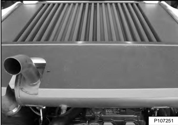
Lift and pull the rear grille backward to remove from the loader **[Figure 188]**.
