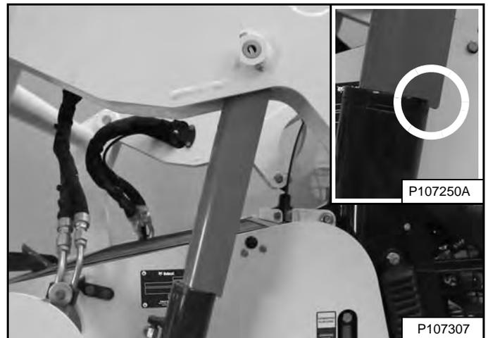
Lower the lift arms slowly until the lift arm support device is held between the lift arms and the lift cylinder. The tabs of the lift arm support device must go past the end of the cylinder (Inset) [Figure 171].
