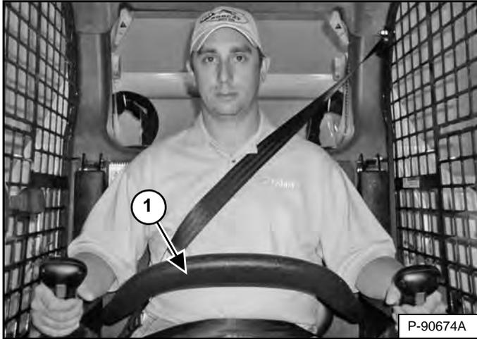
The seat bar restraint system has a pivoting seat bar with armrests (Item 1) [Figure 34].
