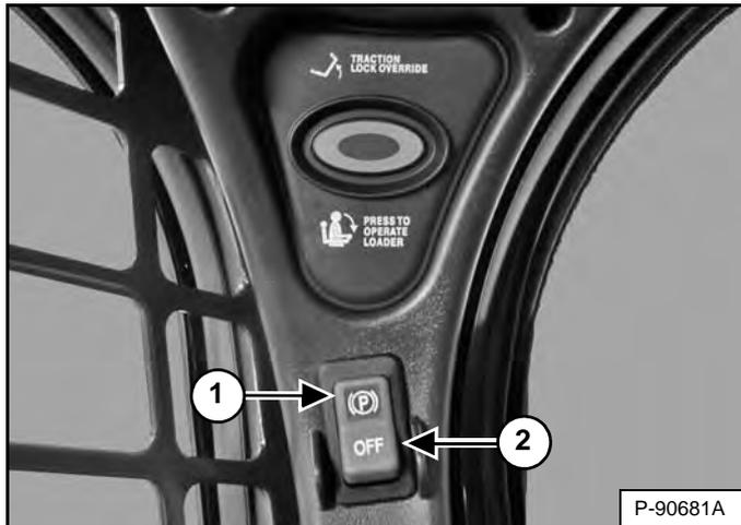
Press the top of the switch (Item 1) [Figure 35] to engage the parking brake. The red light in the switch will turn on. The traction drive system is locked.
