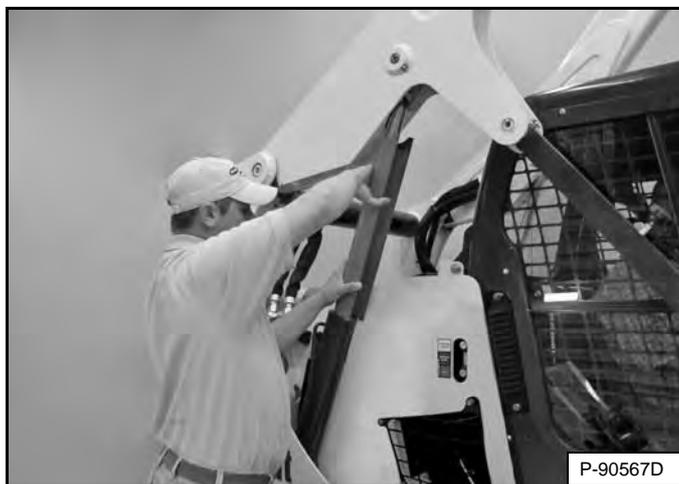
Have a second person remove the lift arm support device **[Figure 172]**.
