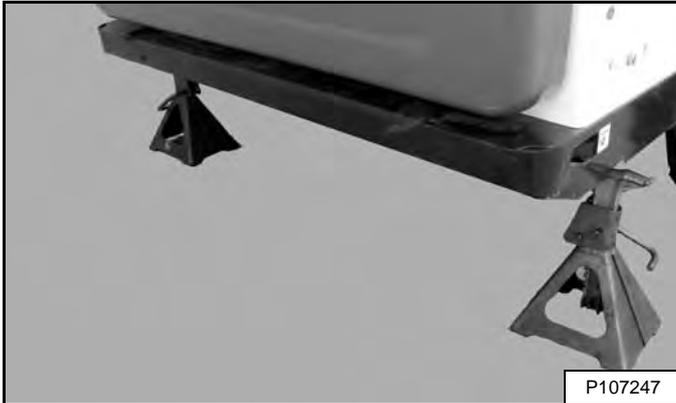
Install jackstands under the rear of the loader frame [Figure 180].
