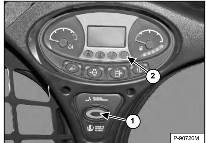
*(Functions Only When The Seat Bar Is Raised And The Engine Is Running)* There is a TRACTION LOCK OVERRIDE button (Item 1) [Figure 36] on the left instrument panel that will allow you to use the steering controls to move the loader forward and backward when using the backhoe attachment.
