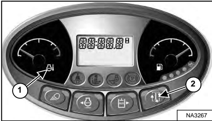
Frequently monitor the temperature and fuel gauges and BICS™ lights (all BICS™ lights must be OFF to operate loader) [Figure 129].
