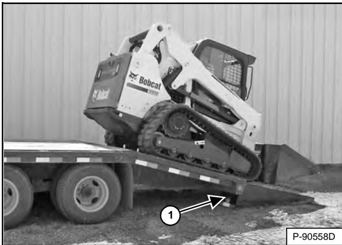
A loader with an empty bucket or no attachment must be loaded backward onto the transport vehicle [Figure 162].
