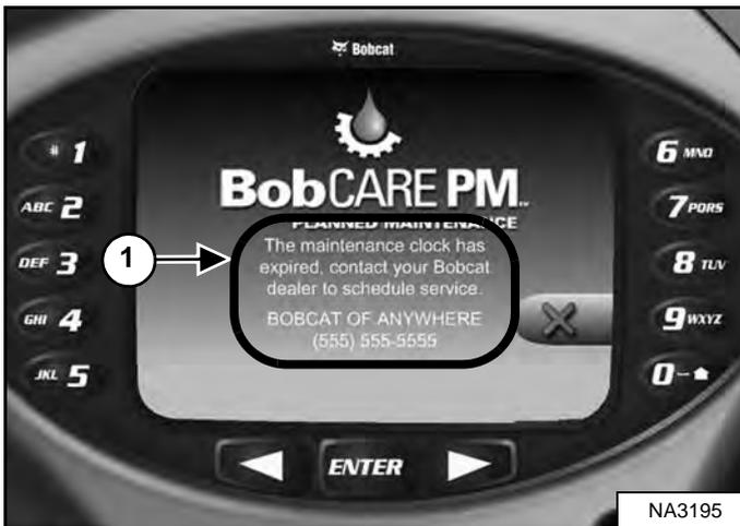
The Deluxe Instrumentation Panel (if equipped) will display a message (Item 1) [Figure 315] alerting the operator to service the machine.
