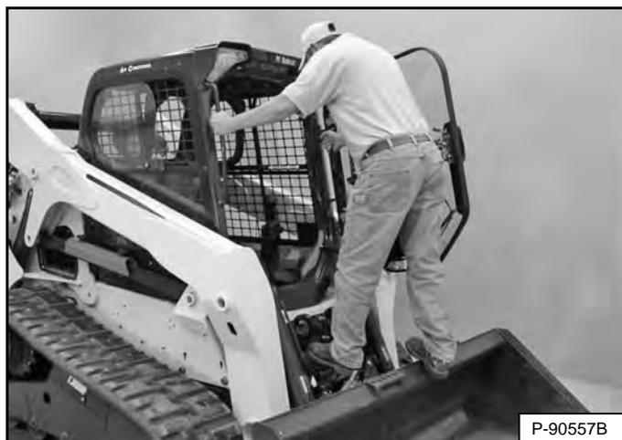
Use the bucket or attachment steps, grab handles, and safety treads (on the loader lift arms and frame) to get on and off the loader, maintaining a three-point contact at all times [Figure 104]. Do not jump.
