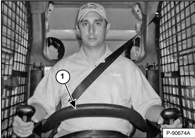
The seat bar restraint system has a pivoting seat bar with armrests (Item 1) [Figure 165].
