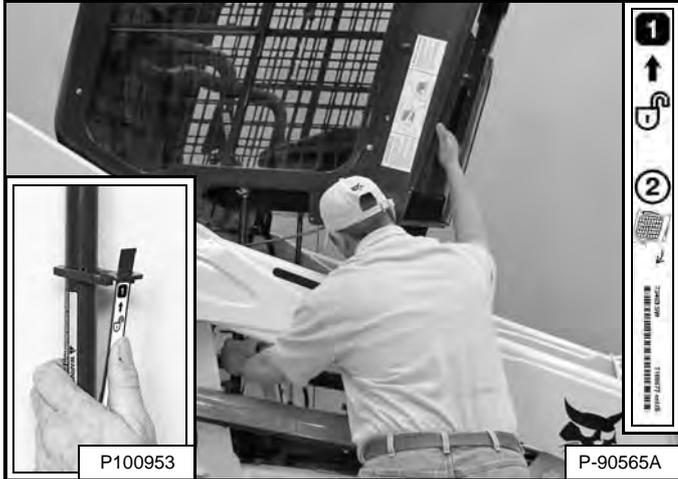
Pull down on the bottom of the operator cab until stopped by the latching mechanism [Figure 183].
