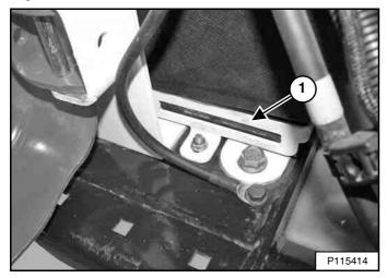
Earlier models use a clamp (Item 1) **[Figure 242]** at the base of the battery. (See Removing (Earlier Models) on Page 167.)
