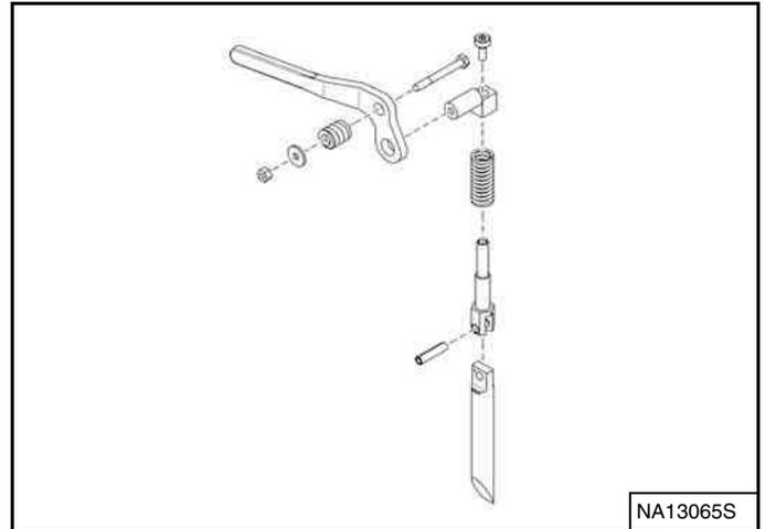
Inspect the mounting frame on the attachment and Bob-Tach, linkages, and wedges for excessive wear or damage [Figure 312]. Replace any parts that are damaged, bent, or missing. Keep all fasteners tight.
