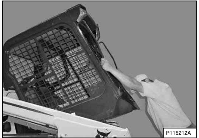
Lift on the grab handles and bottom of the operator cab [Figure 187] slowly until the operator cab is all the way up and the latching mechanism engages.
