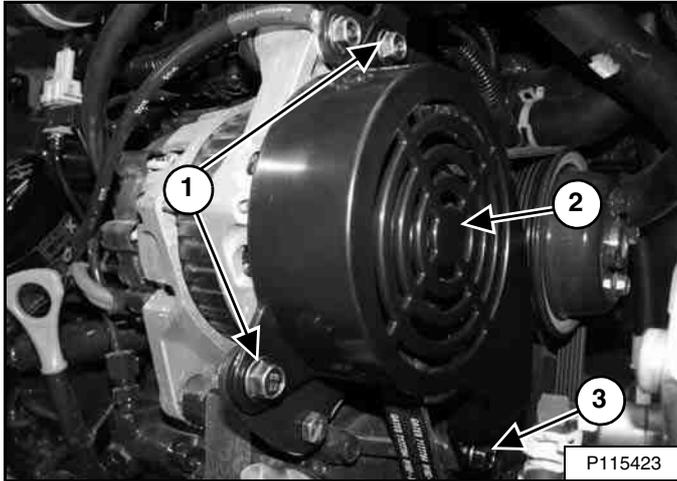
Remove the alternator belt shield mounting nuts and bolts (Item 1). Remove the mounting bolt (Item 3) [Figure 287].
