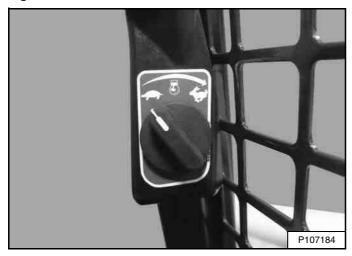
Set the engine speed control to the low idle position [Figure 127].
