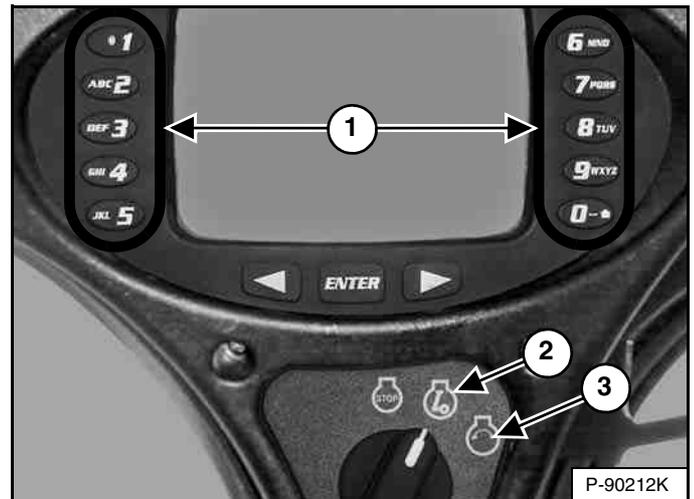
Turn the key switch to RUN (Item 2). The indicator lights on the left instrument panel will come ON briefly and the instrument panel / monitoring system will perform a self test. Use the numeric keypad (Item 1) [Figure 128] to enter the password.
