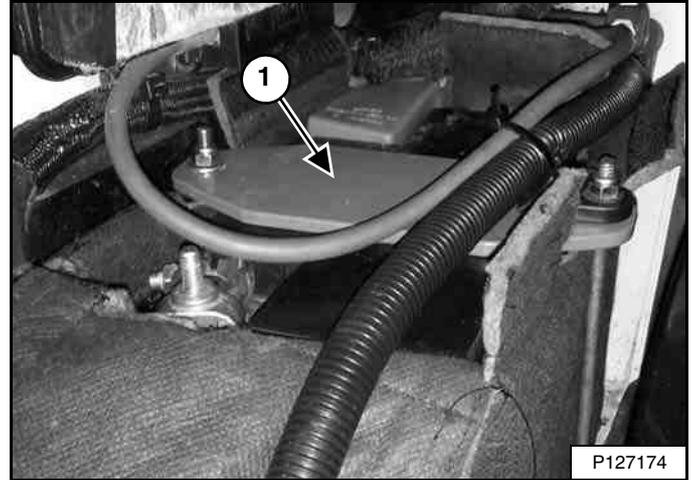
Later models use a bracket (Item 1) [Figure 243] over the top of the battery. (See Removing (Later Models) on Page 169.)
