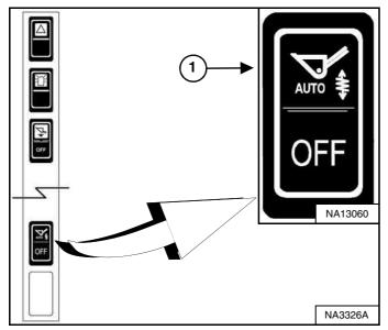
Press the top of the Automatic Ride Control switch (Item 1) **[Figure 86]** on the left switch panel to engage the automatic ride control function.
