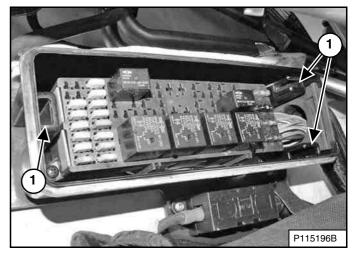
Line up the clips on the back of the fuse panel cover with the slots (Item 1) **[Figure 235]** in the fuse panel and push the cover into position when finished.
