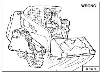
*Turning:* Use a gradual turn (one lever farther forward than the other) instead of a fast turn (one lever forward and one lever backward) on asphalt or concrete surfaces to prevent reduced track life or derailing of the tracks **[Figure 154]**.
