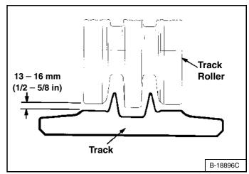
DO NOT put your fingers into the pinch points between the track and the roller. Use a 13 - 16 mm (1/2 - 5/8 in) bolt, dowel or block to check the gap **[Figure 275]** and **[Figure 276]**.
