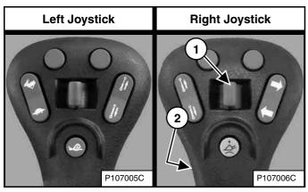
After activating the auxiliary hydraulics, press the Continuous Flow Control switch (Item 2) [Figure 92] or [Figure 93] to allow constant auxiliary hydraulic fluid flow to the front female coupler (female coupler is pressurised). (EXAMPLE: Operate a backhoe.)
