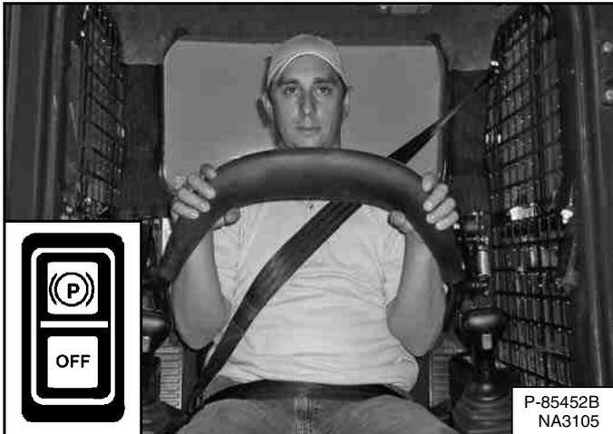
Lower the seat bar and engage the parking brake [Figure 115].
