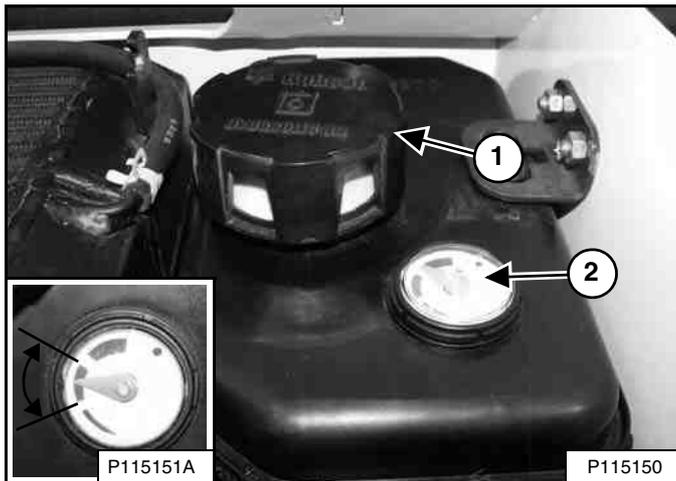
Check the fluid level in the sight gauge (Item 2). Keep the fluid level within the operating range (Inset) [Figure 256].
