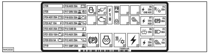
The table below is for later models with decal part number 7308513. Fuse location and amperage ratings are shown in the table below and on the decal [Figure 238]. Relays are identified by the letter "R" in the AMP column.
