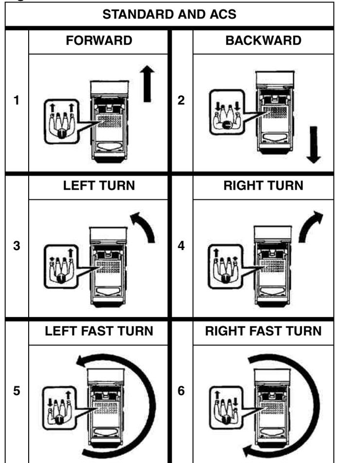
*Steering Lever Functions (Drive And Steering)* [Figure 59]:
