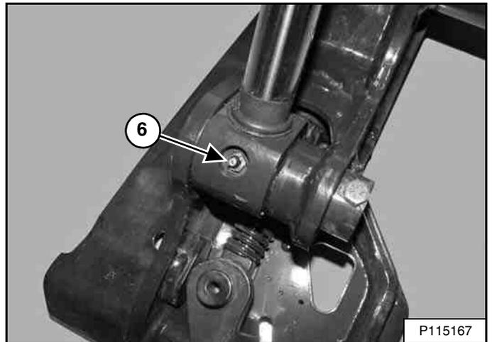
6. Rod End Tilt Cylinder (Both Sides) (2) [Figure 306].
