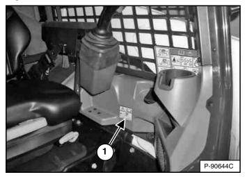
Inspect for damaged or missing back-up alarm decal (Item 1) [Figure 179]. Replace if required.
