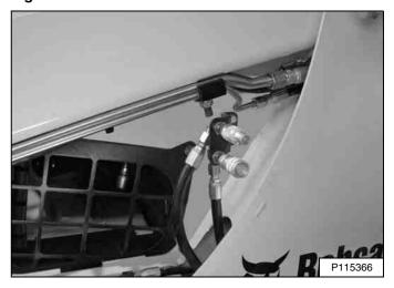
Move the Rear Auxiliary Hydraulic switch (Item 1) [Figure 95] or [Figure 96] to the right or left to change direction of the auxiliary hydraulic fluid flow to the rear quick couplers [Figure 97]. (Left side shown.) (EXAMPLE: Raise and lower rear stabilisers.) Release the switch to stop fluid flow.
