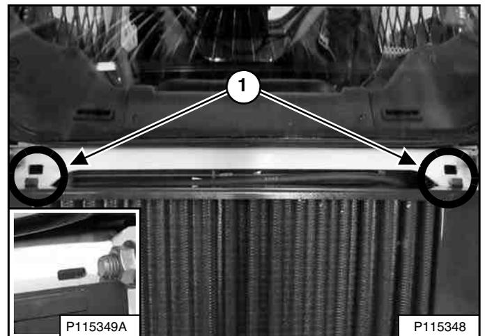
The front edge of the rear grille has two tabs that fit into slots in the loader frame (Item 1) [**Figure 194**]. Insert the tabs into the slots and lower the rear grille.
