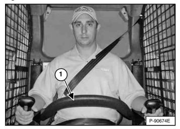
The Bobcat Interlock Control System (BICS<sup>TM</sup>) has a pivoting seat bar with armrests (Item 1) [Figure 35]. The operator controls the use of the seat bar.
