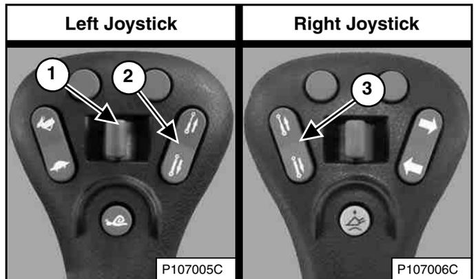
Additional switches (Items 1, 2, and 3) [Figure 104] or [Figure 105] are used to control some attachment functions through the attachment control device.
