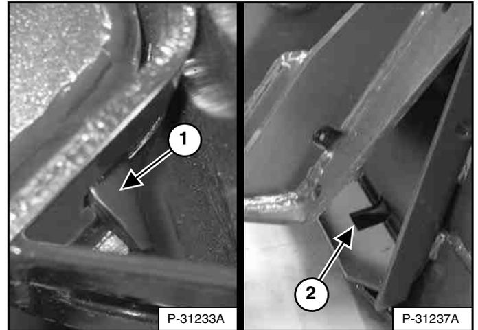
The wedges (Item 1) must extend through the holes (Item 2) **[Figure 142]** in the mounting frame of the bucket (or other attachment), securely fastening the bucket to the Bob-Tach.
