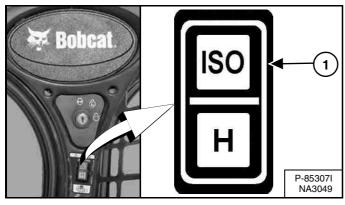
Select the 'ISO' control pattern by pressing the top of the switch (Item 1) [Figure 60].
