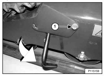
Tighten the access cover bolt (Item 1) [Figure 280] to secure the tool.
