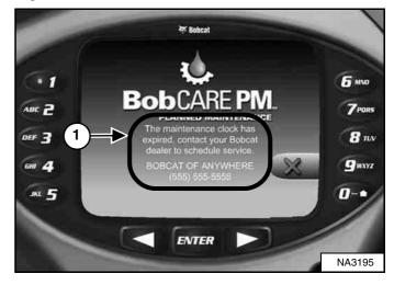
The Deluxe Instrumentation Panel (if equipped) will display a message (Item 1) [Figure 321] alerting the operator to service the machine.
