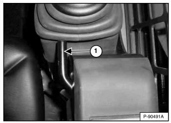
Pull the joystick adjustment lever (Item 1) [Figure 116] up to slide the loader joystick forward or backward to adjust for comfortable operation. (Right side shown.)
