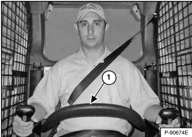
The seat bar restraint system has a pivoting seat bar with armrests (Item 1) [Figure 169].
