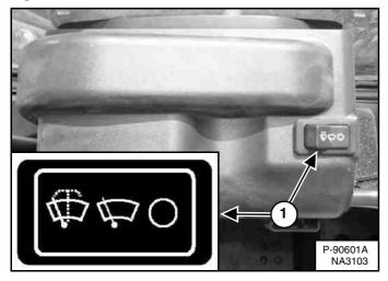
Press the left side of the switch (Item 1) **[Figure 32]** to start the front wiper (press and hold for washer fluid). Press the right side of the switch to stop the wiper.
