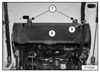
Remove the nut (Item 3) holding the operator cab electrical harness clamp and move the harness toward the front of the loader. Remove the bolts (Item 1) and remove the lower fan duct (Item 2) [Figure 291].
