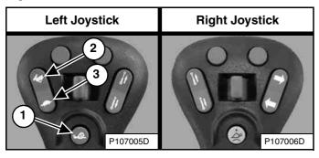
Press the button (Item 1) [Figure 68] on the left joystick once to engage Speed Management.
