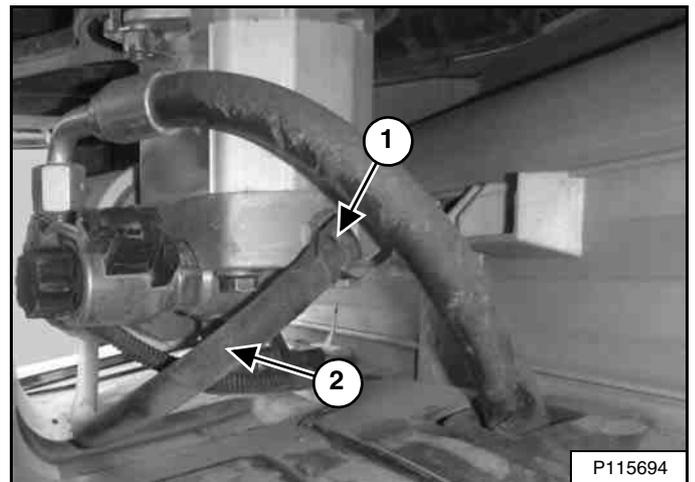
Remove the clamp (Item 1). Pinch off the hose (Item 2) [Figure 262] near the fitting and disconnect hose from the fitting.
