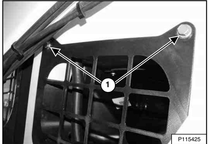
Remove the left side access cover bolts (Item 1) [Figure 292] and remove the access cover.
