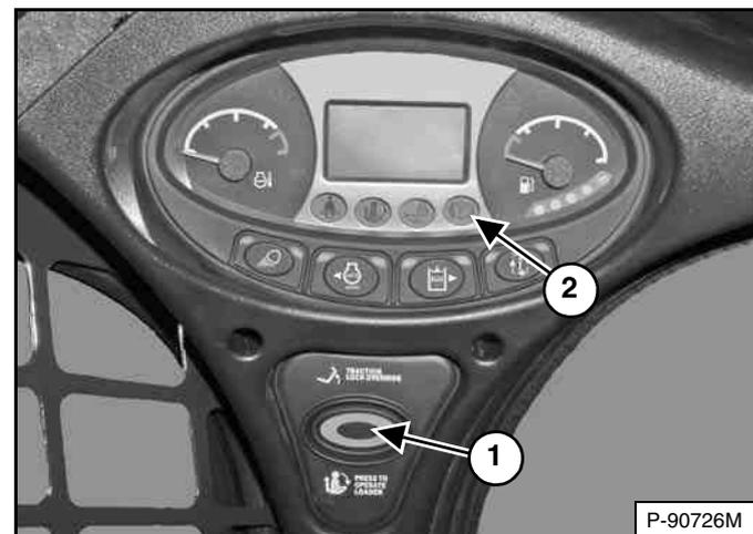
*(Functions Only When The Seat Bar Is Raised And The Engine Is Running)* There is a TRACTION LOCK OVERRIDE button (Item 1) [Figure 39] on the left instrument panel that will allow you to use the steering controls to move the loader forward and backward when using the backhoe attachment.
