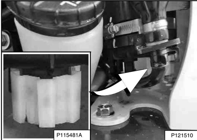
Loosen the drain (Inset) [Figure 211] at the bottom of the filter to remove trapped water from the filter.
