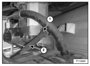
Remove the clamp (Item 1). Pinch off the hose (Item 2) **[Figure 262]** near the fitting and disconnect hose from the fitting.
