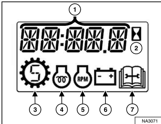
The display screen is shown in **[Figure 12]**. The data display will show operating hours upon startup.
