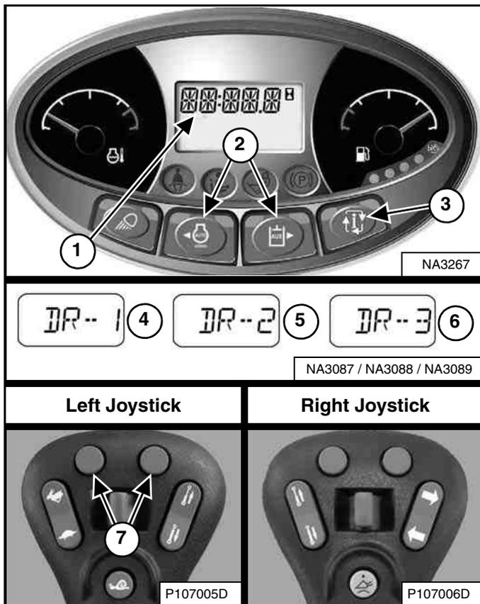
Press the Information button (Item 3) to cycle the data display until the drive response menu is displayed. The current drive response setting will appear in the data display (Item 1) [Figure 72].
