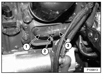
Remove the clamp (Item 2) and disconnect the hose (Item 3) from the engine oil cooler fitting (Item 1) **[Figure 230]**.
