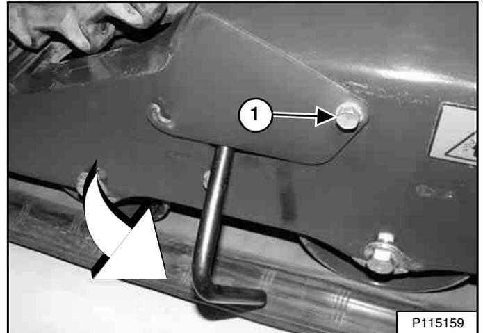
Tighten the access cover bolt (Item 1) [Figure 280] to secure the tool.
