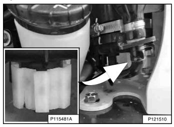
Loosen the drain (Inset) **[Figure 211]** at the bottom of the filter to remove trapped water from the filter.
