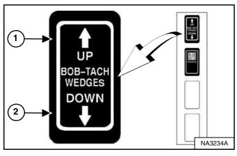
Push and hold the BOB-TACH WEDGES "UP" switch (Item 1) until wedges are fully raised. Push and hold the BOB-TACH WEDGES "DOWN" switch (Item 2) [Figure 313] until the wedges are fully down.
