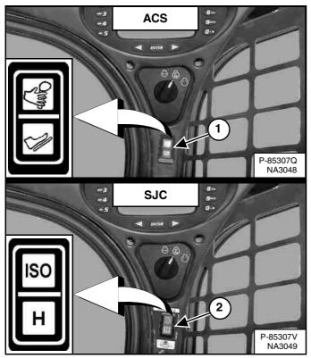
(ACS) Select hand control or foot pedal operation (Item 1) [Figure 130] if equipped with ACS.
