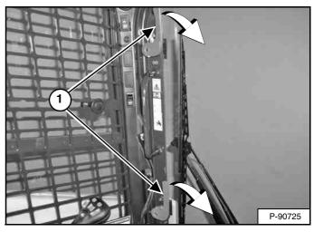
Turn both latches (Item 1) [Figure 52] down until they disengage from the door frame.
