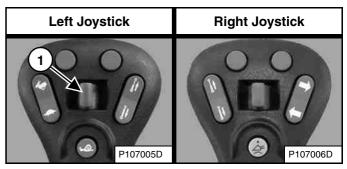
Move the Rear Auxiliary Hydraulic switch (Item 1) **[Figure 100]** or **[Figure 101]** to the left and right several times. Turn the key switch to STOP.
