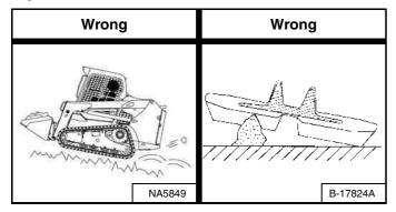
Avoid operating or turning on sharp objects such as jagged rocks, broken concrete, quarry materials, or scrap applications. This can cause cuts on the lug surface of the tracks [Figure 158].
