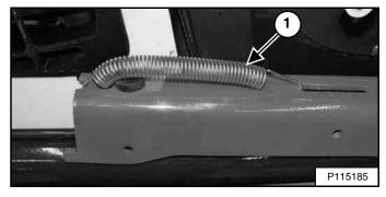
Lower the lift arm support device to the top of the lift cylinder. Hook the free end of the spring (Item 1) [Figure 174] to the lift arm support device to prevent interference with lift arm support device engagement.
