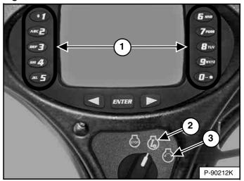
Turn the key switch to RUN (Item 2). The indicator lights on the left instrument panel will come ON briefly and the instrument panel / monitoring system will perform a self test. Use the numeric keypad (Item 1) [Figure 128] to enter the password.
