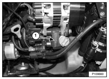
The engine serial number (Item 1) [Figure 2] is located on the side of the engine next to the oil fill cap.
