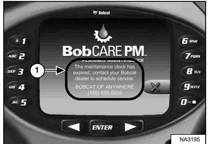
The Deluxe Instrumentation Panel (if equipped) will display a message (Item 1) [Figure 321] alerting the operator to service the machine.
