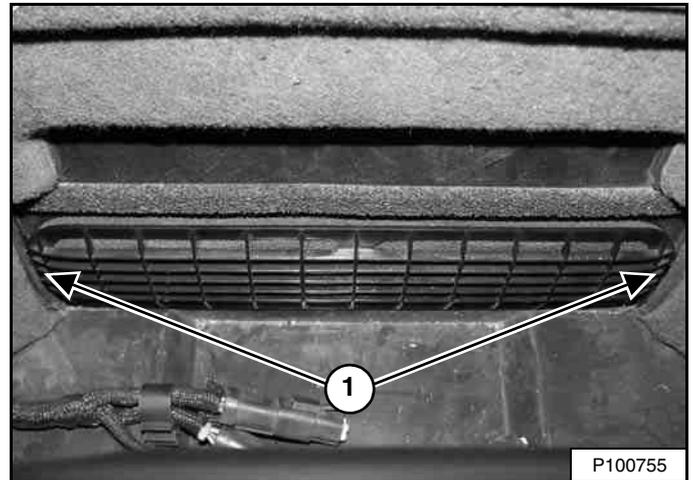
The recirculation filter is located behind the operator's seat inside the operator cab. The filter cover is held in position with three clips. Pull the cover at each end (Item 1) [Figure 196] to remove.
