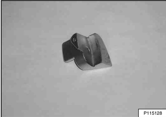
A belt tool [Figure 290] is required to install the new air conditioning belt. See your Bobcat dealer.
