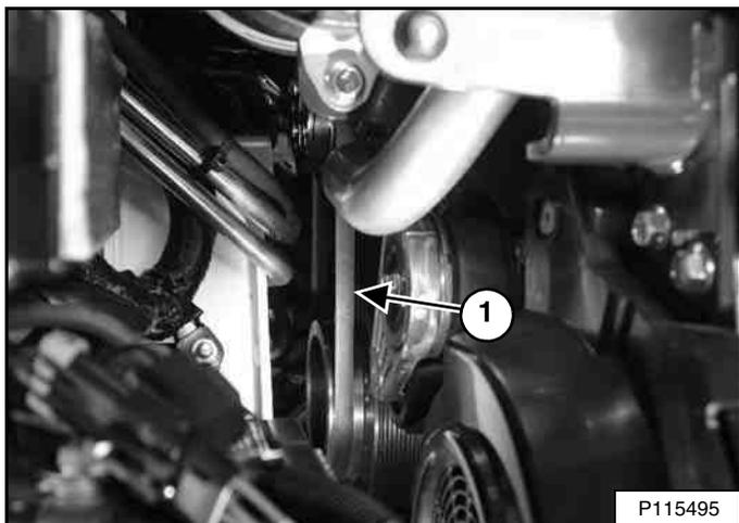
Cut the old belt (Item 1) [Figure 294] and remove the belt from the pulleys. Inspect the pulleys for wear.
