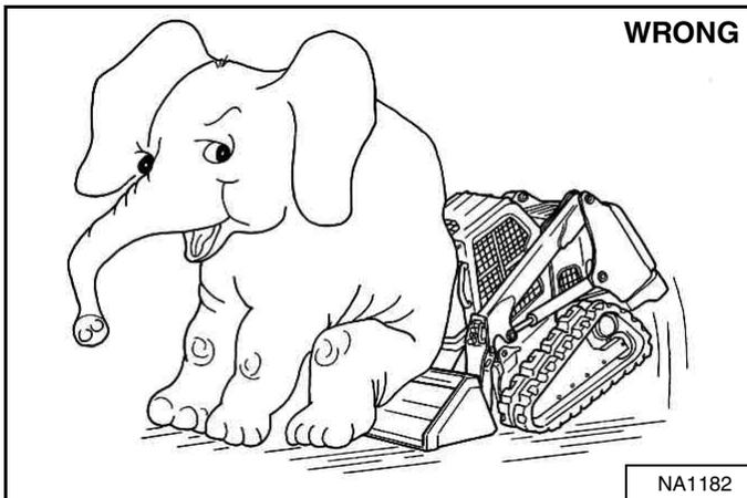
Exceeding the ROC [Figure 137] can cause the following problems:
