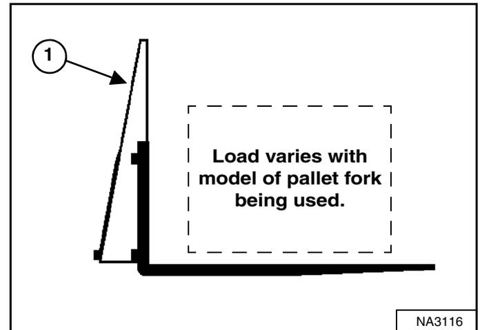
The maximum load to be carried when using a pallet fork is shown on a decal located on the pallet fork frame (Item 1) [Figure 138].
