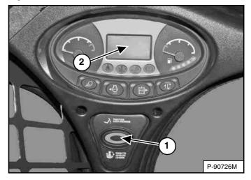
Press the PRESS TO OPERATE LOADER button (Item 1) **[Figure 121]** to activate the BICS<sup>™</sup> and to perform hydraulic and loader functions.
