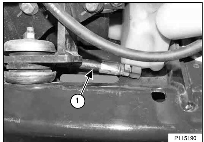
The oil drain hose (Item 1) [Figure 217] storage location is near the fuel tank fill. Route the oil drain hose through the opening.
