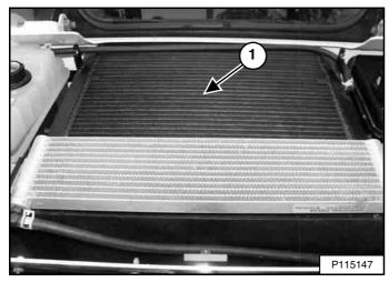
Use low air pressure or water pressure to clean the top of the hydraulic fluid cooler and radiator assembly (Item 1) **[Figure 225]**.
