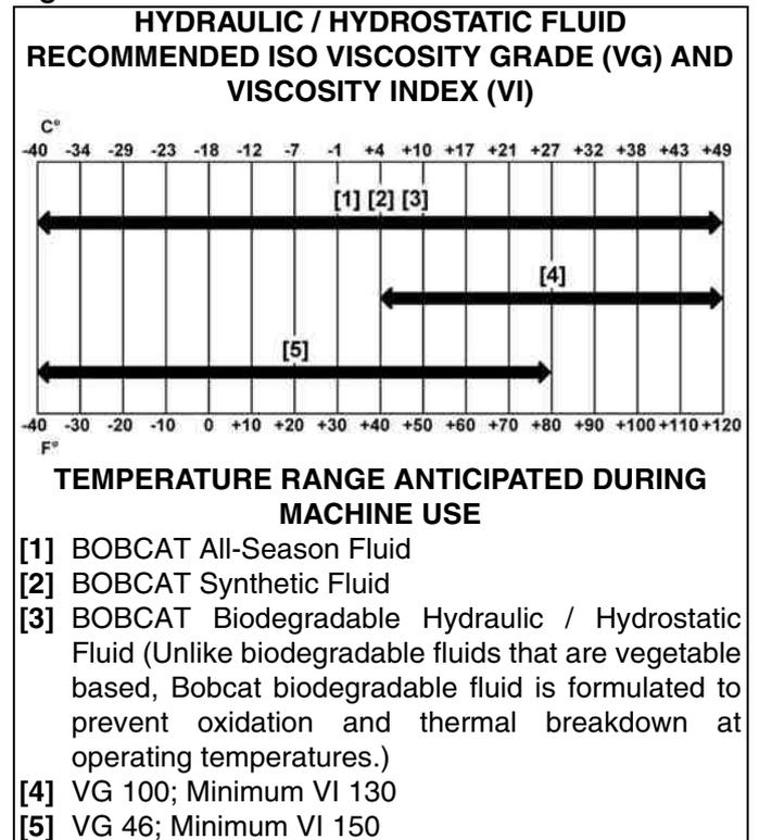
Bobcat hydraulic fluids are recommended for use in this machine. If Bobcat hydraulic fluid is not available, use a good quality hydraulic fluid meeting the viscosity grade and viscosity index shown in the chart [Figure 257].
