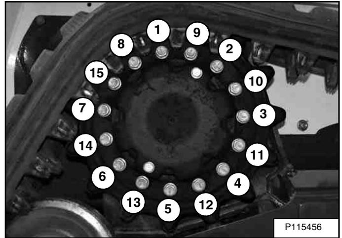
Check the torque of the fifteen track sprocket bolts (Items 1 – 15) [Figure 286]. Use an alternating tightening sequence and then repeat to tighten the bolts to 122,0 – 135,6 N•m (90 – 100 ft-lb) torque.
