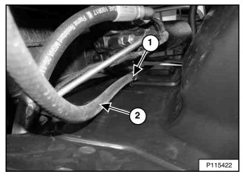
Remove the clamp (Item 1). Pinch off the hose (Item 2) **[Figure 260]** near the fitting and disconnect hose from the fitting.
