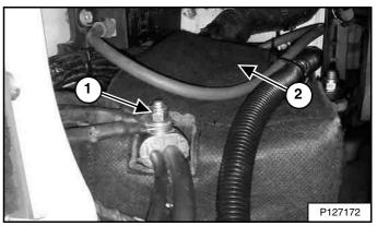
Close and securely fasten the top flap of the battery wrap (Item 2) [Figure 255].
