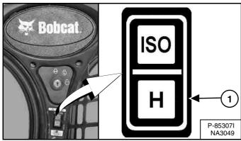
Select the 'H' control pattern by pressing the bottom of the switch (Item 1) [Figure 63].
