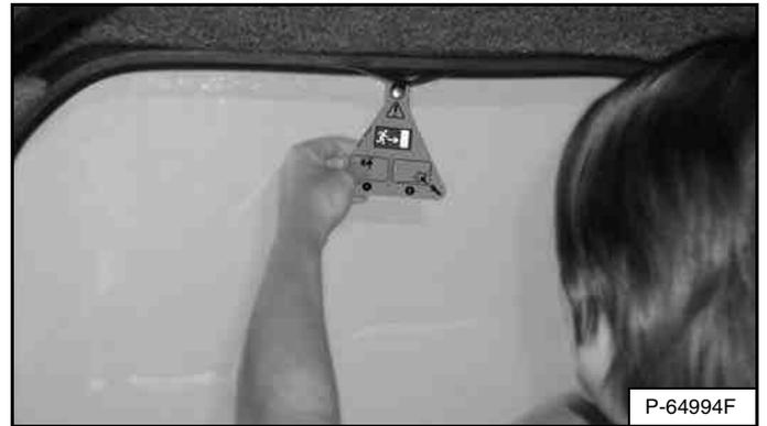
Pull on the tag on the top of the rear window to remove the rubber cord [Figure 47].
