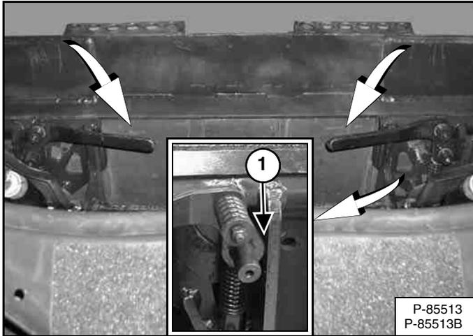
Push down on the Bob-Tach levers until they are fully engaged in the locked position **[Figure 141]** (wedges fully extended through the attachment mounting frame holes).
