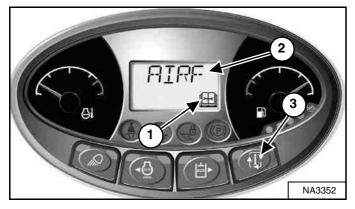
Replace the air filters only when necessary. The service indicator (Item 1) will FLASH. Press the Information button (Item 3) until the display screen shows the service codes. Service code **[AIRF]** (Replace Engine Air Filter) or **[M0117]** (Air Filter Plugged) will show in the display screen (Item 2) **[Figure 204]** when air filter replacement is necessary.
