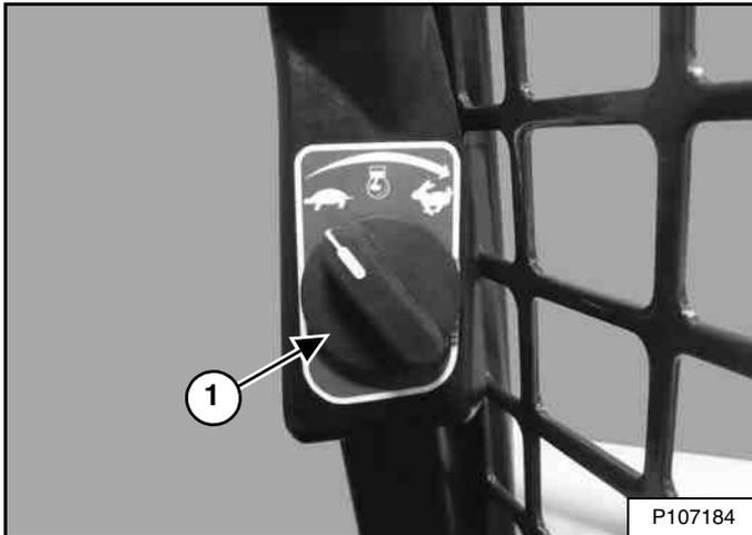
The engine speed control (Item 1) [Figure 40] is located alongside the door frame below the right panel.
