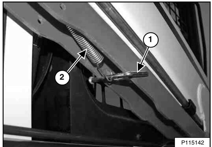
Raise the lift arm support device into the storage position and insert the retaining pin (Item 1) through the lift arm support device and the bracket. Hook the spring (Item 2) [Figure 178] to the retaining pin.
