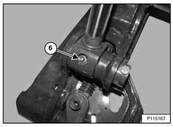
6. Rod End Tilt Cylinder (Both Sides) (2) [Figure 306].
