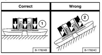
The track carriage components will wear faster when operated on a slope. When the machine is operated on a level surface, the weight of the machine is distributed throughout the entire surface of the rollers to the tracks (Item 1). When operated on a slope, the weight is directed to the edge of the rollers and against the lugs of the track (Item 2) **[Figure 156]** which causes increased wear.
