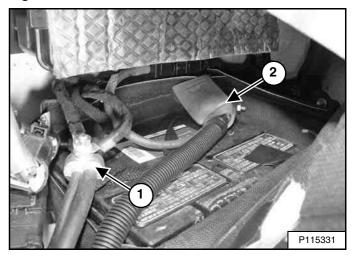
Connect and tighten the positive (+) cable (Item 2). Connect and tighten the negative (-) cable (Item 1) [Figure 249] last to prevent sparks. Tighten the nuts to 5,4 - 6,8 N-m (4 - 5 ft-lb) torque.
