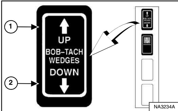
Push and hold the BOB-TACH WEDGES “UP” switch (Item 1) until wedges are fully raised. Push and hold the BOB-TACH WEDGES “DOWN” switch (Item 2) [Figure 313] until the wedges are fully down.
