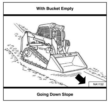
With an empty bucket, go up or down the slope with the heavy end toward the top of the slope [Figure 161] and [Figure 162].
