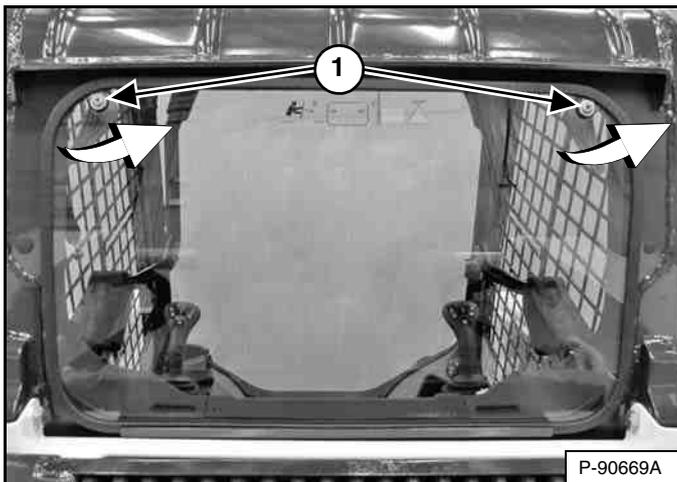
The rear window can be removed from outside the loader using a T40 TORX® Drive tool. Turn both screws (Item 1) [Figure 49] anticlockwise until the latches disengage from the window frame. Pull the top of the window away from the cab and lift up to remove.
