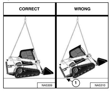
Attach cables or chains to lift eyes [Figure 165].
