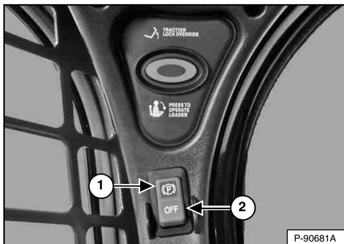
Press the top of the switch (Item 1) [Figure 38] to engage the parking brake. The red light in the switch will turn ON. The traction drive system is locked.
