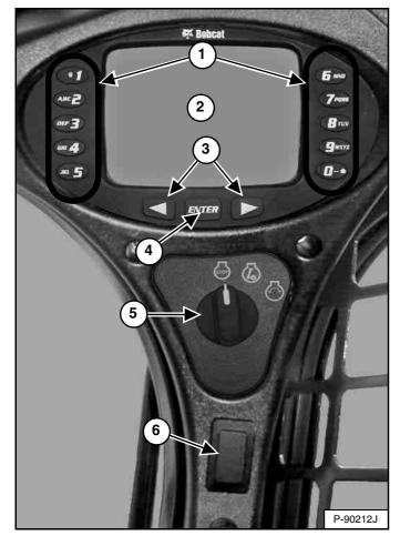
This machine may be equipped with a Deluxe Instrumentation Panel [Figure 15].
