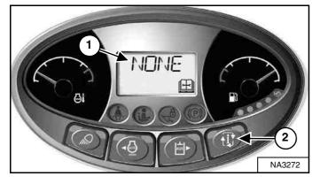
Press the Information button (Item 2) to cycle the data display (Item 1) **[Figure 316]** until the service code screen is displayed. If more than one service code is present, the codes will scroll on the data display.
