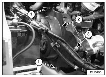
Remove the drive belt shield bolt (Item 3) [Figure 296].
