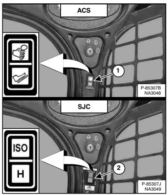
(ACS) Select hand control or foot pedal operation (Item 1) [Figure 120] if equipped with ACS.
