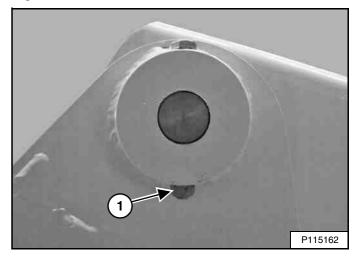
All lift arm and cylinder pivots have a large pin held in position with a retainer bolt and locknut (Item 1) [Figure 309].
