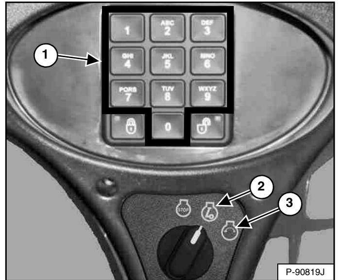
Turn the key switch to RUN (Item 2). The indicator lights on the left instrument panel will come ON briefly and the instrument panel / monitoring system will perform a self test. Use the numeric keypad (Item 1) [Figure 123] to enter the password.
