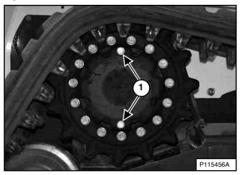
Park the loader so that the plugs (Item 1) [Figure 285] in the hydrostatic drive motor are at the top and the bottom.
