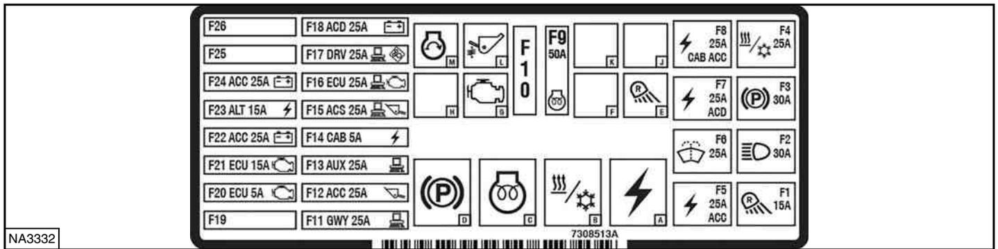
The table below is for later models with decal part number 7308513. Fuse location and amperage ratings are shown in the table below and on the decal [Figure 238]. Relays are identified by the letter "R" in the AMP column.
