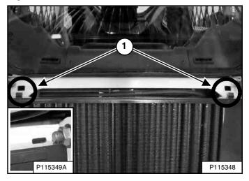
The front edge of the rear grille has two tabs that fit into slots in the loader frame (Item 1) **[Figure 194]**. Insert the tabs into the slots and lower the rear grille.
