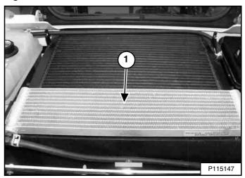
Use low air pressure or water pressure to clean the top of the fuel cooler (Item 1) [Figure 221].
