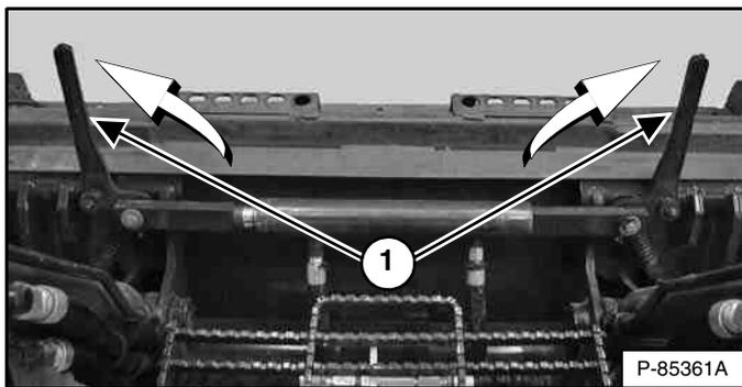
Push and hold BOB-TACH WEDGES "UP" switch (Right Switch Panel) [Figure 145] until levers (Item 1) [Figure 146] are fully raised (wedges fully raised).
