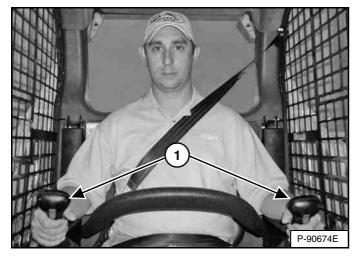
Both joysticks control drive and steering and are located on the left and right side in front of the seat (Item 1) [Figure 64].
