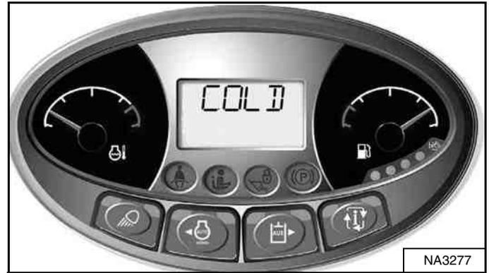
The engine controller will not allow full engine speed and torque when the engine temperature is too low. The following indications and actions are performed automatically by the engine controller:
