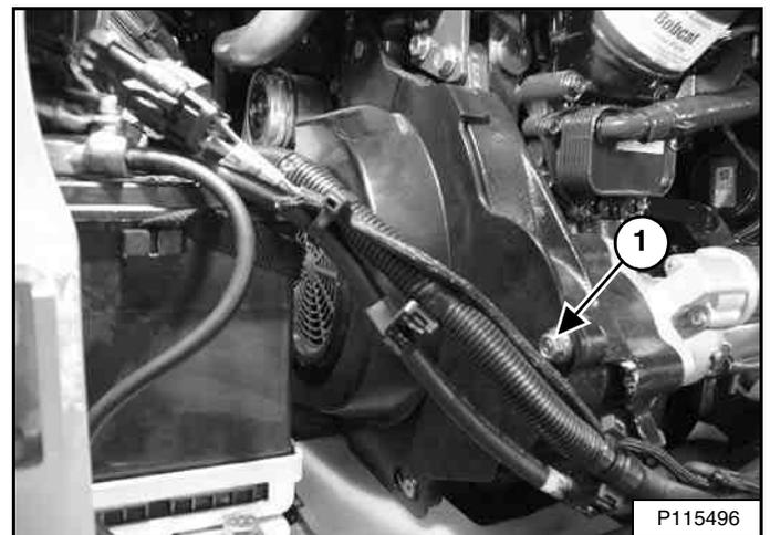
Install the drive belt shield bolt (Item 1) [Figure 299].
