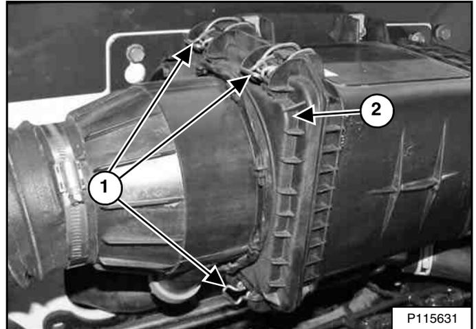
Install the cover (Item 2) and secure four latches (Item 1) **[Figure 208]**. (One latch is not visible in the photo.)
