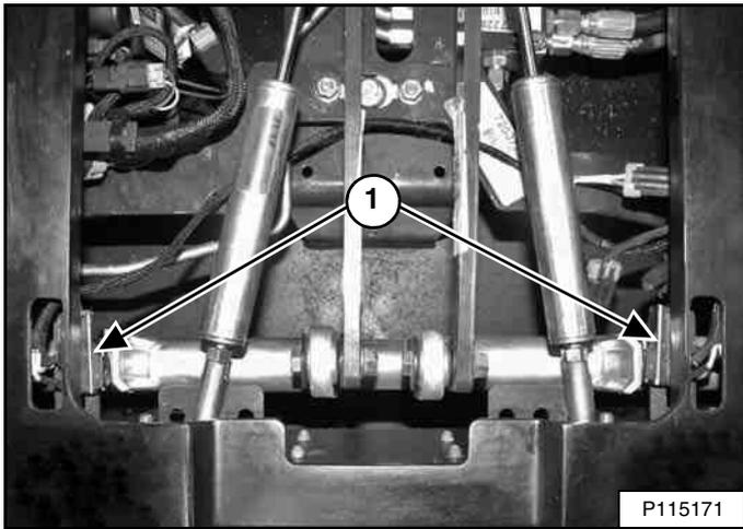
The back-up alarm switches (Item 1) [Figure 181] are located alongside the steering bellcranks. Both switches must be adjusted properly for the back-up alarm to operate correctly.
