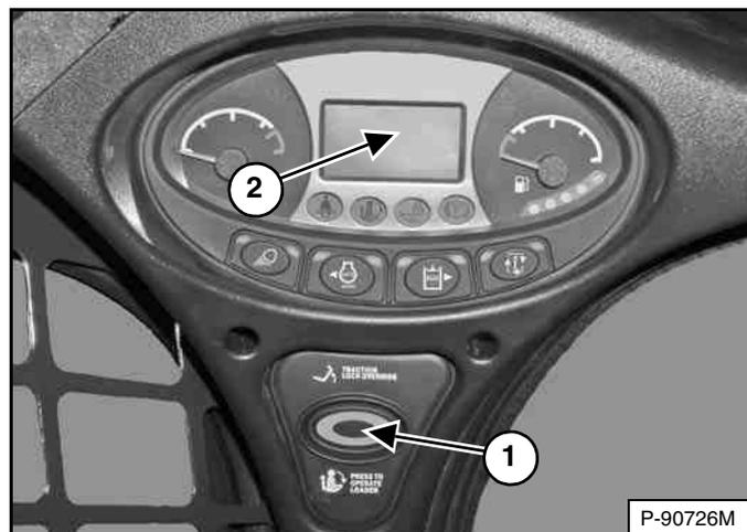
Press the PRESS TO OPERATE LOADER button (Item 1) [Figure 131] to activate the BICST™ and to perform hydraulic and loader functions.
