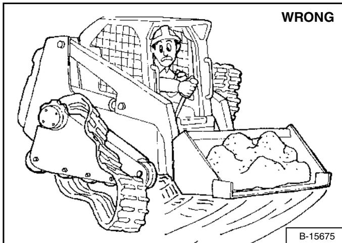
**Turning:** Use a gradual turn (one lever farther forward than the other) instead of a fast turn (one lever forward and one lever backward) on asphalt or concrete surfaces to prevent reduced track life or derailing of the tracks [Figure 154].
