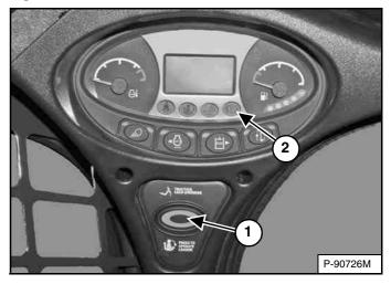
(Functions Only When The Seat Bar Is Raised And The Engine Is Running) There is a TRACTION LOCK OVERRIDE button (Item 1) [Figure 39] on the left instrument panel that will allow you to use the steering controls to move the loader forward and backward when using the backhoe attachment.
