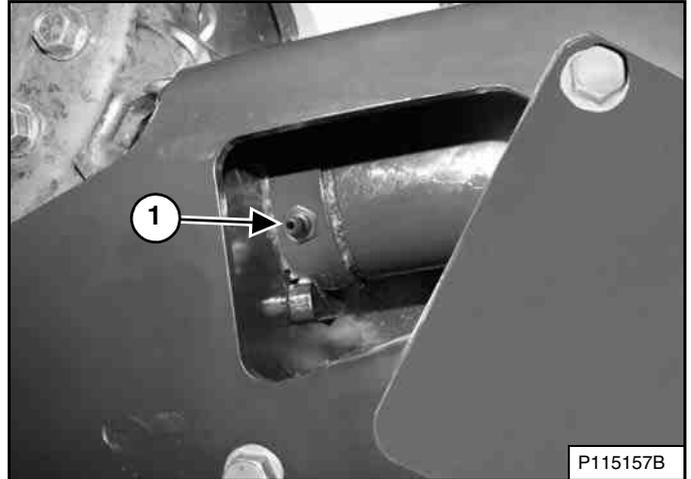
Add grease to the track tension fitting (Item 1) [Figure 282] until the track adjustment is correct [Figure 275] and [Figure 276].
