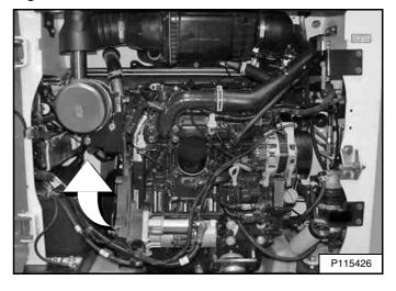
The air conditioning compressor is located behind the engine on the left side of the loader [Figure 293].
