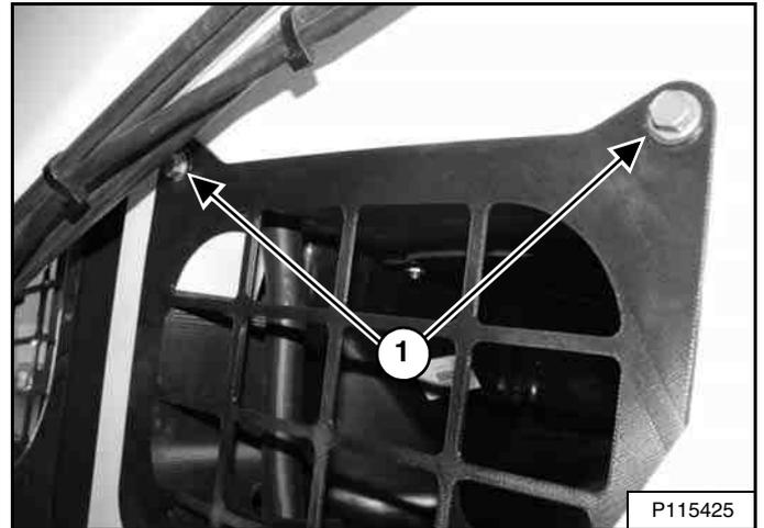
Remove the left side access cover bolts (Item 1) [Figure 261] and remove the access cover.
