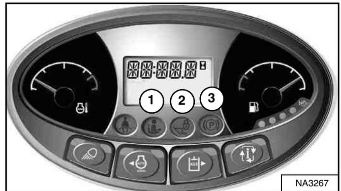
There are three display lights (Items 1, 2, and 3) [Figure 36] located on the left instrument panel that must be OFF to fully operate the machine.
