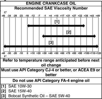
Bobcat engine oils are recommended for use in this machine. If Bobcat engine oil is not available, use a good quality engine oil that meets API Service Category of CJ-4 or better, or ACEA E9 or better [Figure 215].
