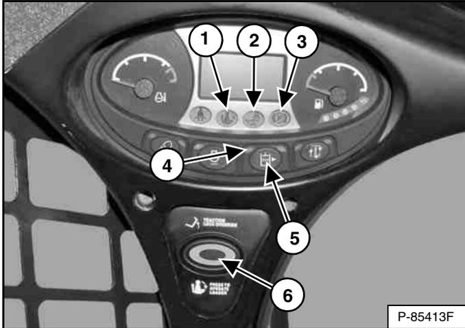
1. Sit in operator's seat. Turn key switch to RUN. Lower seat bar and disengage parking brake. Press the PRESS TO OPERATE LOADER button (Item 6). Two BICS™ lights (Items 1 and 2) [Figure 168] [SEAT BAR and LIFT AND TILT VALVE] on left instrument panel must be OFF. The PRESS TO OPERATE LOADER button will light.
