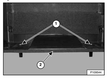
Clean the plenum drains (Item 1) [Figure 199] to ensure they are not plugged by debris.
