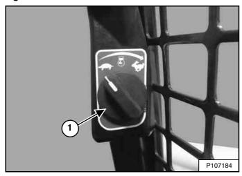
The engine speed control (Item 1) [Figure 40] is located alongside the door frame below the right panel.
