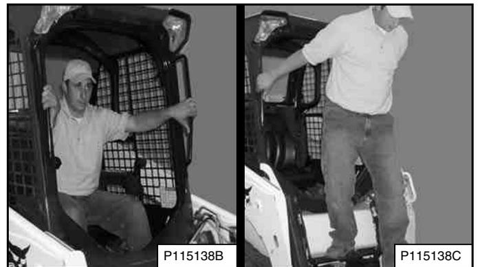
Exit the loader using grab handles, safety tread, and steps (maintaining a three-point contact) [Figure 136].
