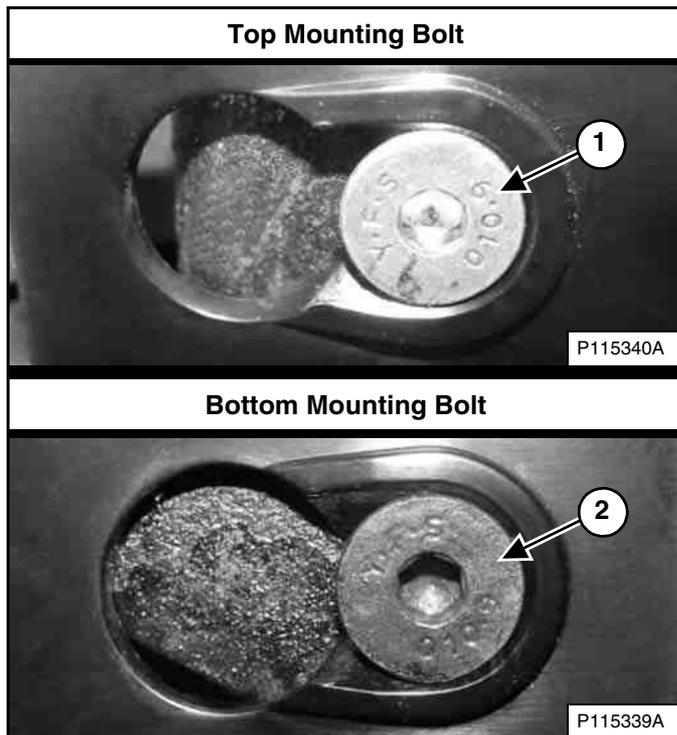
Position the drive belt shield over the drive belt shield mounting bolts. Slide the drive belt shield toward the front of the loader to fully seat the shield onto the top and bottom mounting bolts (Items 1 and 2) [Figure 298].
