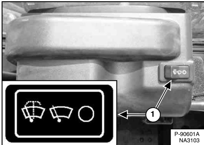
Press the left side of the switch (Item 1) [Figure 32] to start the front wiper (press and hold for washer fluid). Press the right side of the switch to stop the wiper.
