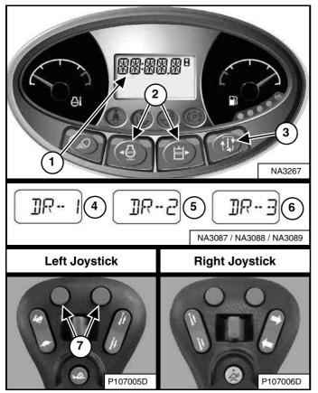
Press the Information button (Item 3) to cycle the data display until the drive response menu is displayed. The current drive response setting will appear in the data display (Item 1) [Figure 72].
