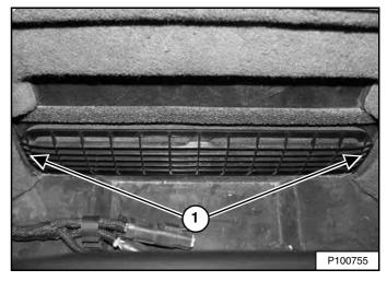
The recirculation filter is located behind the operator's seat inside the operator cab. The filter cover is held in position with three clips. Pull the cover at each end (Item 1) [Figure 196] to remove.
