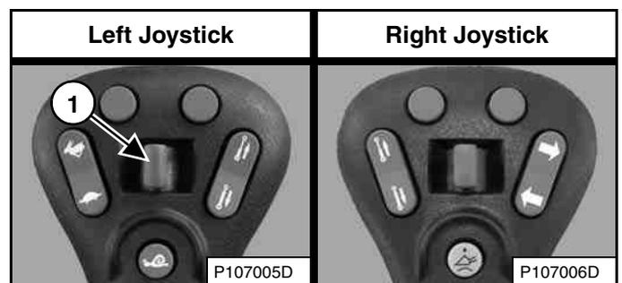
Move the Rear Auxiliary Hydraulic switch (Item 1) [Figure 100] or [Figure 101] to the left and right several times. Turn the key switch to STOP.
