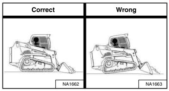
*Digging And Levelling:* Keep the full length of the tracks in contact with the ground [Figure 155] for best traction.
