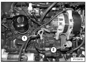
Park the loader on a level surface. Stop the engine. Open the rear door and remove the dipstick (Item 1) **[Figure 214]**.
