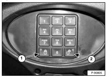
Press and hold the lock (Item 1) and unlock (Item 2) [Figure 319] keys for 2 seconds.
