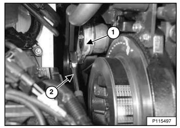
Insert a breaker bar (Item 2) into the square hole provided in the idler assembly (Item 1) [Figure 297] as shown and push the breaker bar down to release tension on the drive belt.
