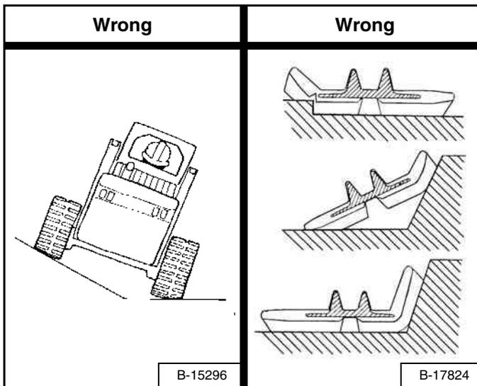
**Operating Conditions:** Avoid operating the loader with one track on a slope and the other on flat ground or with the end of the track turned up against a curb or mound [Figure 157]. This can cause the tracks to derail, cracks in the edge of the tracks, or cracks at the edges of the embedded metal.
