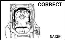
Always use the seat bar and fasten seat belt snugly. Always keep feet on the foot pedals or
