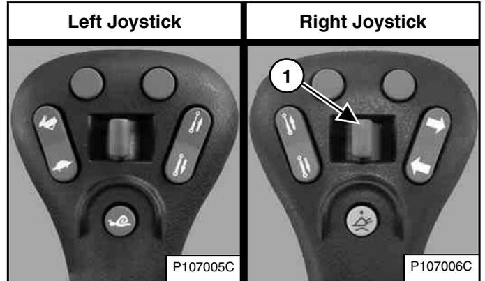
Move the Front Auxiliary Hydraulic switch (Item 1) [Figure 90] or [Figure 91] to the right or left to change direction of the auxiliary hydraulic fluid flow to the front quick couplers. If you move the switch halfway, the auxiliary functions move at approximately one-half speed. (EXAMPLE: Open and close grapple teeth.)
