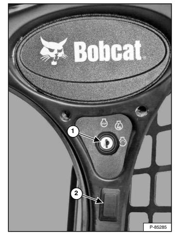
This machine may be equipped with a Standard Key Panel **[Figure 13]**.
