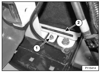
Slightly raise the battery wrap to gain access to the battery clamp.
