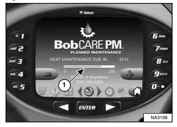
The Deluxe Instrumentation Panel (if equipped) will display a bar (Item 1) [Figure 322] showing the time remaining until next service. This bar will turn red when service is past due. [NEXT MAINTENANCE DUE] will change to [MAINTENANCE PAST DUE] and display the number of hours past due.
