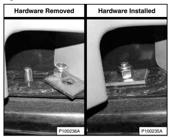
Install the washers and nuts (both sides) [Figure 189]. Tighten the nuts to 54 - 61 N•m (40 - 45 ft-lb) torque.
