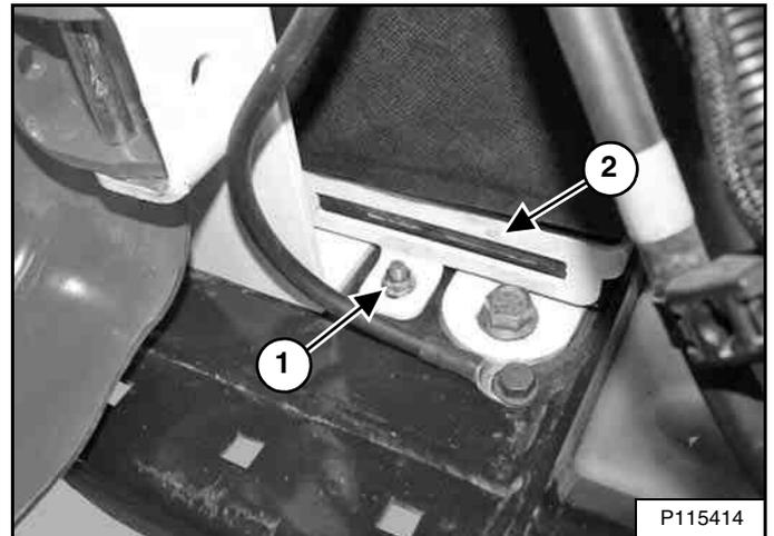
Slightly raise the battery wrap to gain access to the battery clamp.
