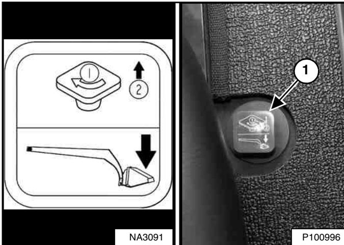
The lift arm bypass control (Item 1) [Figure 43], located to the right of the operator's seat, is used to lower the lift arms if the lift arms cannot be lowered during normal operations.
