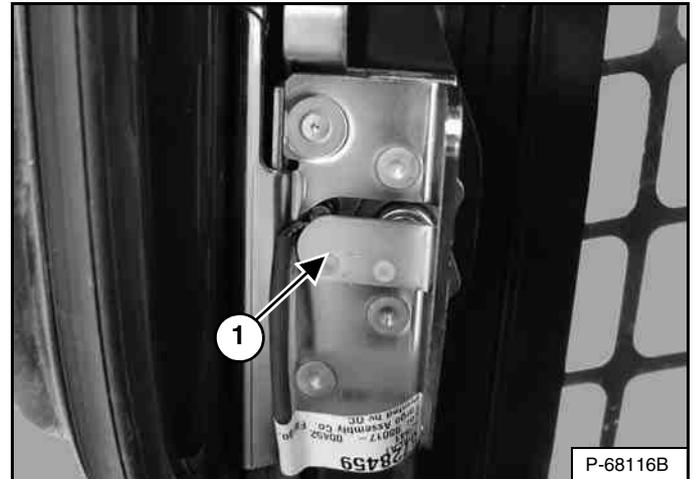
The cab door has a sensor (Item 1) [Figure 183] installed that deactivates the lift and tilt valves when the door is open.
