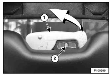
The lever (Item 1) is used to adjust the suspension response of the seat depending on the operator's weight. The optimum setting is achieved with the needle (Item 2) **[Figure 110]** centred in the gauge with the operator normally seated.
