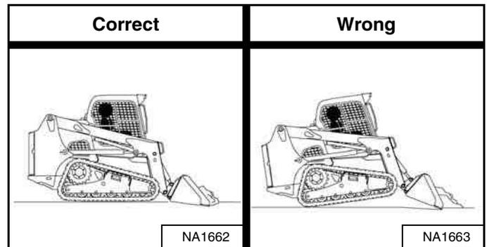
**Digging And Levelling:** Keep the full length of the tracks in contact with the ground [Figure 155] for best traction.
