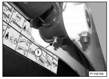
3. Rod End Lift Cylinder (Both Sides) (2) [Figure 303].
