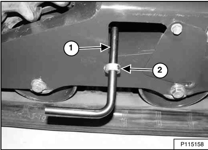
Install the bleed tool (7277225) (Item 1) on the track tension fitting, adjust and tighten the collar (Item 2) [Figure 283] to fit behind the edge of the access cover. (Right side shown.)
