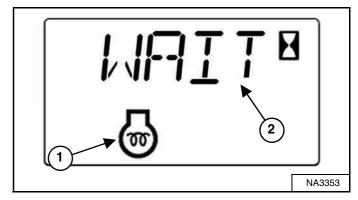
The machine will cycle the glow plugs automatically based on temperature. The engine preheat icon (Item 1) and the cycle time remaining or **[WAIT]** (Item 2) **[Figure 119]** are displayed in the data display.
