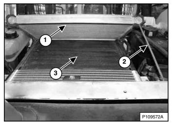
Pivot the air conditioning condenser (Item 1) up and rotate the support bar (Item 2) into position. Use low air pressure or water pressure to clean the top of the hydraulic fluid cooler and radiator assembly (Item 3) **[Figure 223]**.
