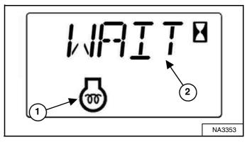
The machine will cycle the glow plugs automatically based on temperature. The engine preheat icon (Item 1) and the cycle time remaining or **[WAIT]** (Item 2) **[Figure 124]** are displayed in the data display.
