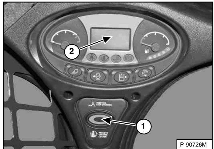
Press the PRESS TO OPERATE LOADER button (Item 1) [Figure 126] to activate the BICST™ and to perform hydraulic and loader functions.
