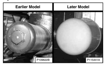
Earlier models use a separate filter housing and filter element. Later models use a spin-on filter **[Figure 266]**. (See Earlier Models on Page 177.) or (See Later Models on Page 178.)
