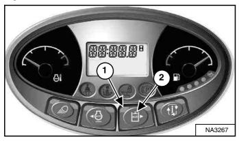
Press the Auxiliary Hydraulics button (Item 2) [Figure 94] once to activate the auxiliary hydraulics.
