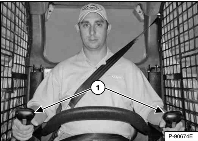
Both joysticks control drive and steering and are located on the left and right side in front of the seat (Item 1) [Figure 64].
