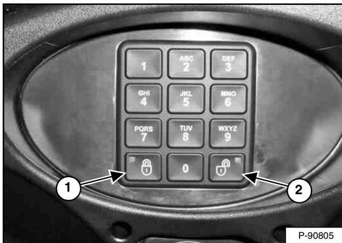
Press and hold the lock (Item 1) and unlock (Item 2) [Figure 319] keys for 2 seconds.
