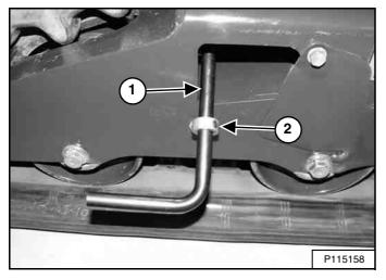
Install the bleed tool (7277225) (Item 1) on the track tension fitting, adjust and tighten the collar (Item 2) **[Figure 283]** to fit behind the edge of the access cover. (Right side shown.)
