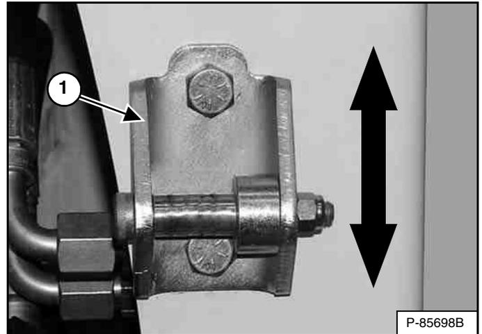
The door latch striker (Item 1) [Figure 192] can be adjusted up or down for alignment with the door latch.
