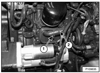
Install the coolant hose (Item 2) onto the engine oil cooler fitting and install the clamp (Item 1) **[Figure 232]**.
