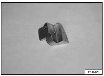
A belt tool **[Figure 290]** is required to install the new air conditioning belt. See your Bobcat dealer.
