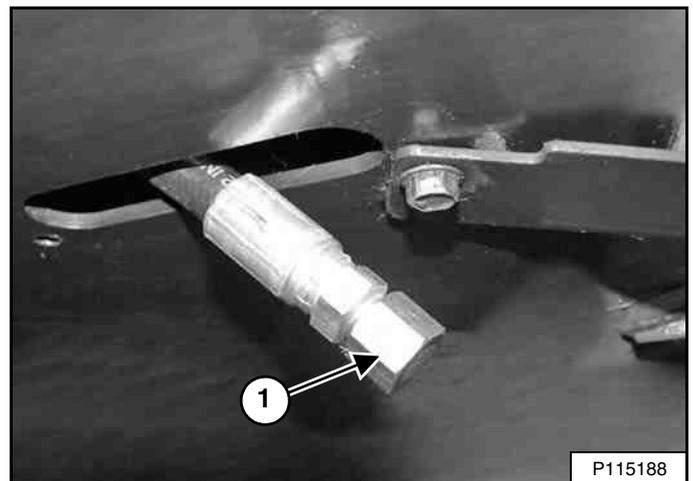
Remove the oil drain cap (Item 1) [Figure 218] from the oil drain hose and drain the oil into a container. Recycle or dispose of used oil in an environmentally safe manner.
