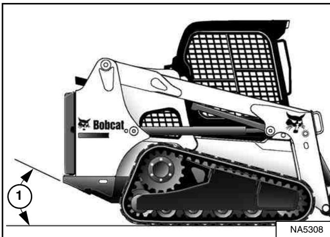
**NOTE:** The loader should be lifted as close to horizontal as possible, but at no time should the angle of the suspended loader exceed the departure angle (Item 1) [Figure 164] provided in the specifications section. (See Machine Dimensions on Page 220.)
