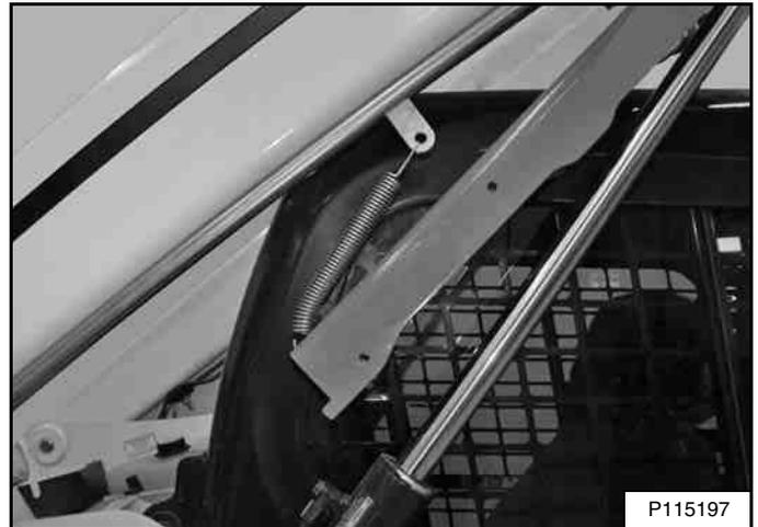
Raise the lift arms a small amount. The spring will lift the lift arm support device off the lift cylinder rod [Figure 177]. Fully lower the lift arms.
