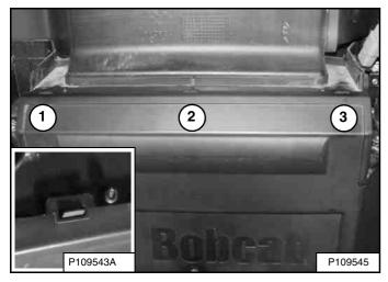
2. Push the cover up in three places (Items 1, 2, and 3) until the slots snap into place on the tabs. This slot (Inset) **[Figure 202]** is correctly fastened.
