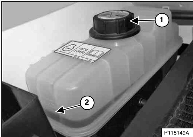
Coolant must be between the top and bottom level markers (Item 2) [Figure 227] when the engine is cold.
