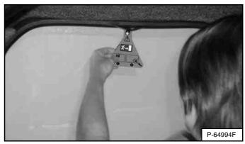
Pull on the tag on the top of the rear window to remove the rubber cord **[Figure 47]**.
