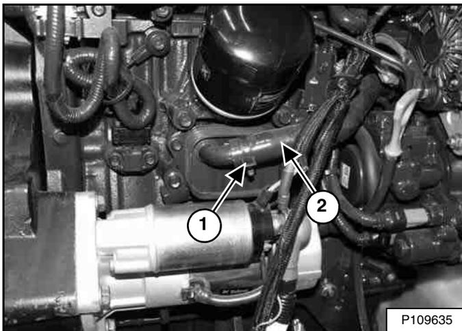
Install the coolant hose (Item 2) onto the engine oil cooler fitting and install the clamp (Item 1) [Figure 232].
