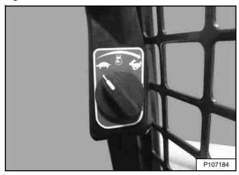
Set the engine speed control to the low idle position [Figure 122].
