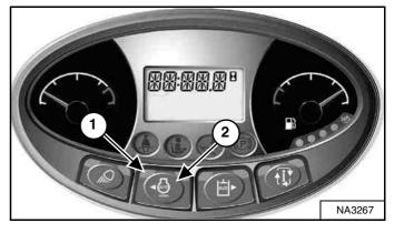
Press the button (Item 2) to engage auto idle. The light (Item 1) **[Figure 42]** is ON.
