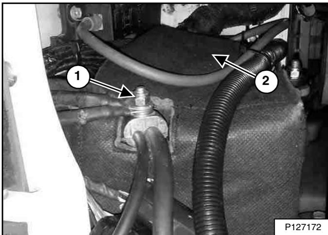
Remove the nut from the top of the negative (-) cable (Item 1) [Figure 250]. Remove the cables.
