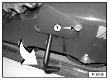
Tighten the access cover bolt (Item 1) [Figure 284] to secure the tool.
