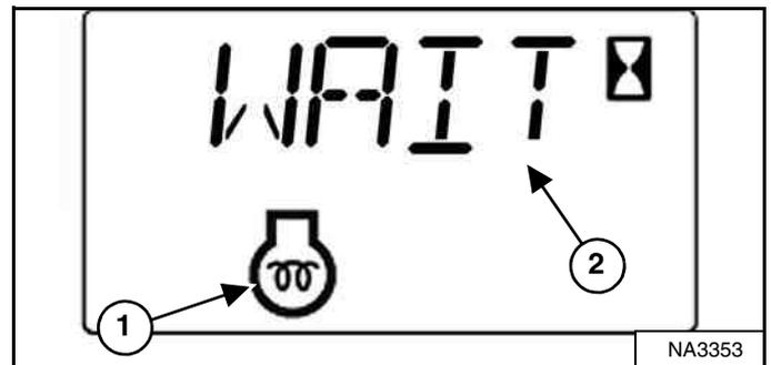
The machine will cycle the glow plugs automatically based on temperature. The engine preheat icon (Item 1) and the cycle time remaining or [WAIT] (Item 2) [Figure 129] are displayed in the data display.
