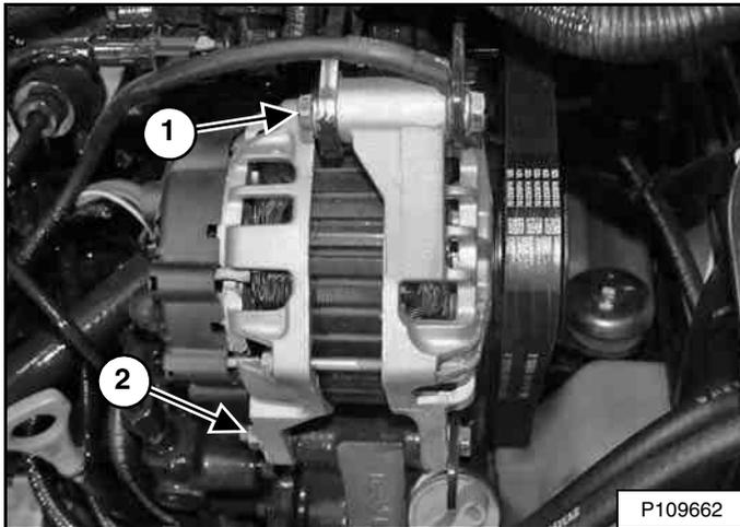
Remove the top alternator mounting bolt (Item 1). Loosen the bottom alternator mounting nut (Item 2) [Figure 288].
