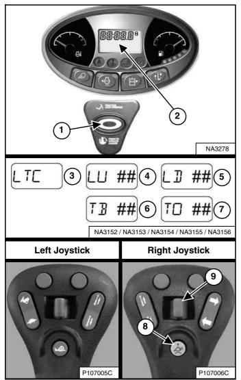
LTC – Lift and Tilt Compensation LU – Lift Up LD – Lift Down TB – Tilt Back TO – Tilt Out
