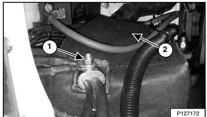
Close and securely fasten the top flap of the battery wrap (Item 2) [Figure 255].
