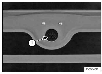
The back-up alarm (Item 1) [Figure 57] is located on the inside of the rear door.
