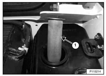
Remove and clean the hydraulic fill screen (Item 1) [Figure 263]. Use low air pressure to dry the screen.
