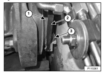
Install the belt on the air conditioning compressor pulley and start the belt (Item 2) and the belt tool (Item 3) on the front side of the hydraulic pump pulley (Item 1) [Figure 295].
