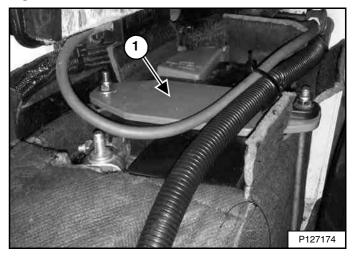
Later models use a bracket (Item 1) **[Figure 243]** over the top of the battery. (See Removing (Later Models) on Page 169.)
