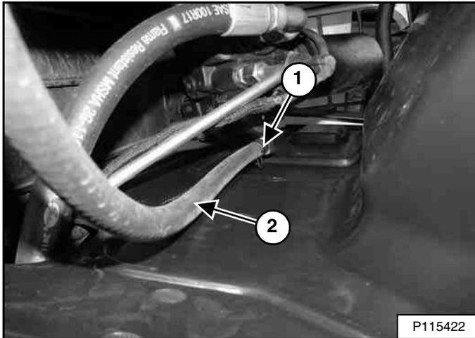
Remove the clamp (Item 1). Pinch off the hose (Item 2) [Figure 260] near the fitting and disconnect hose from the fitting.
