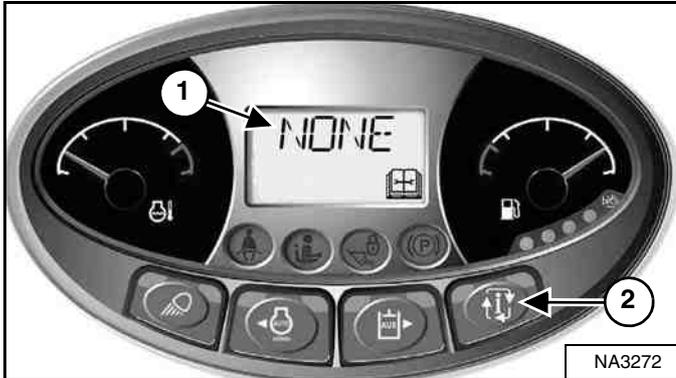
Press the Information button (Item 2) to cycle the data display (Item 1) [Figure 316] until the service code screen is displayed. If more than one service code is present, the codes will scroll on the data display.
