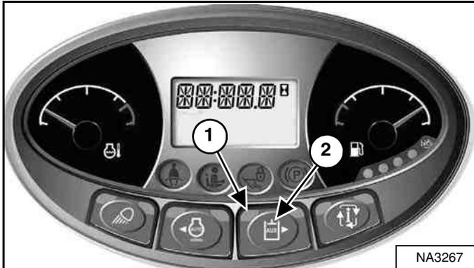
Press the Auxiliary Hydraulics button (Item 2) [Figure 94] once to activate the auxiliary hydraulics.
