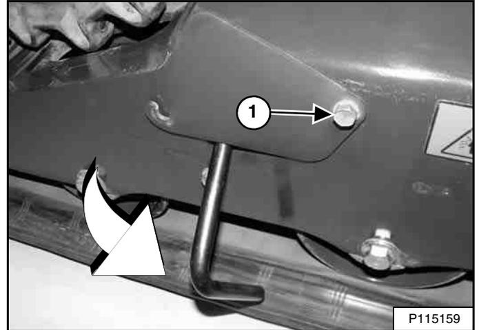
Tighten the access cover bolt (Item 1) [Figure 284] to secure the tool.
