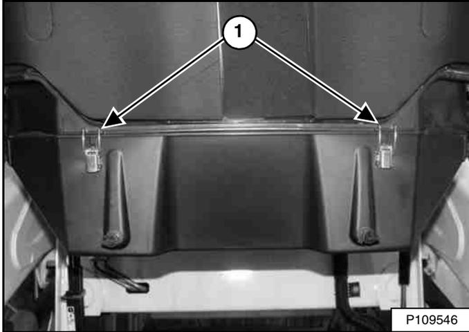
1. Hold the cover in place and fasten two latches (Item 1) [Figure 201].
