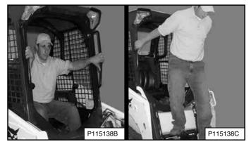
Exit the loader using grab handles, safety tread, and steps (maintaining a three-point contact) [Figure 136].
