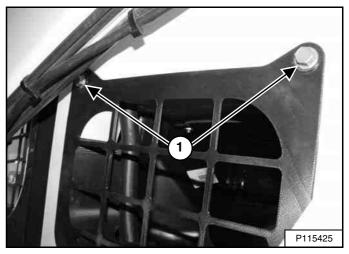
Remove the left side access cover bolts (Item 1) [Figure 292] and remove the access cover.
