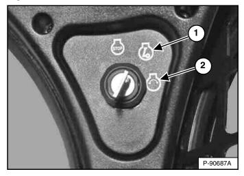
Turn the key switch to RUN (Item 1) [Figure 118]. The indicator lights on the left instrument panel will come ON briefly and the instrument panel / monitoring system will perform a self test.
