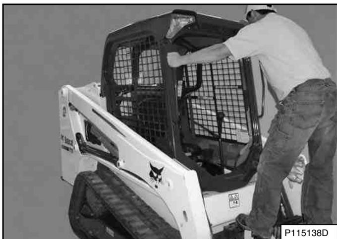
Use the bucket or attachment steps, grab handles, and safety treads (on the loader lift arms and frame) to get on and off the loader, maintaining a three-point contact at all times [Figure 107]. Do not jump.
