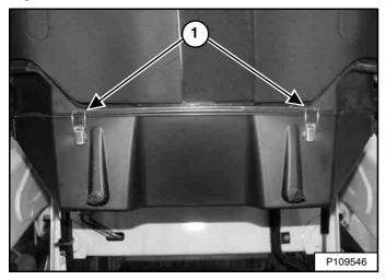
1. Hold the cover in place and fasten two latches (Item 1) [Figure 201].
