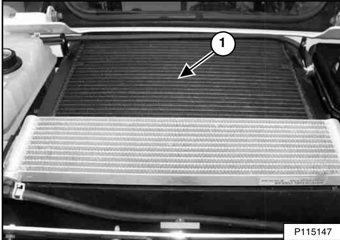
Use low air pressure or water pressure to clean the top of the hydraulic fluid cooler and radiator assembly (Item 1) [Figure 225].
