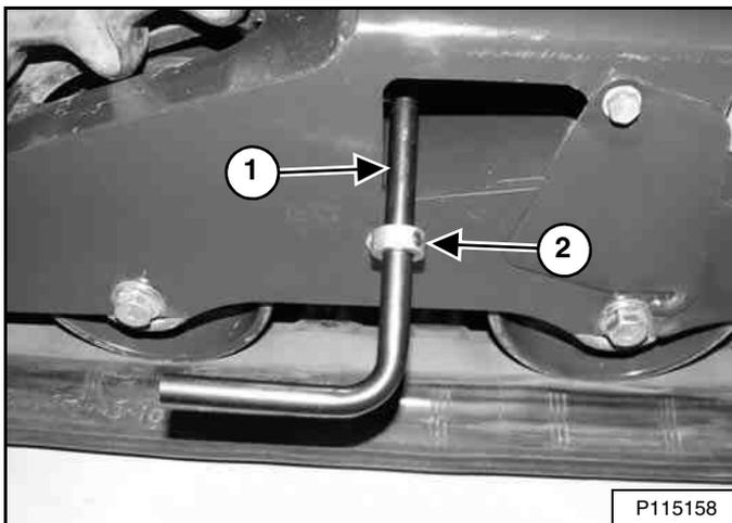
Install the bleed tool (6675936) (Item 1) on the bleed fitting, adjust and tighten the collar (Item 2) [Figure 279] to fit behind the edge of the access cover. (Right side shown.)
