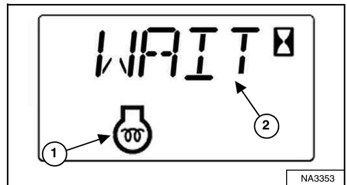
The machine will cycle the glow plugs automatically based on temperature. The engine preheat icon (Item 1) and the cycle time remaining or [WAIT] (Item 2) [Figure 124] are displayed in the data display.
