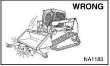
running or with lift arms up. To park, engage parking brake and put attachment flat on the ground.
