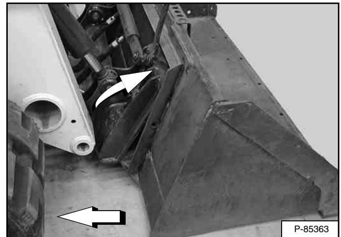
Tilt the Bob-Tach forward and drive the loader backward, away from the bucket or attachment [Figure 153].
