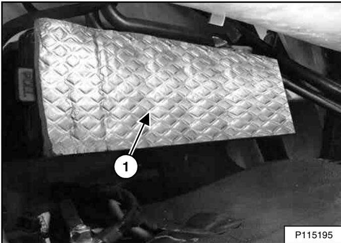
The electrical system is protected from overload by fuses located under the fuse panel cover (Item 1) [Figure 234]. Remove the fuse panel cover by pulling at each end.
