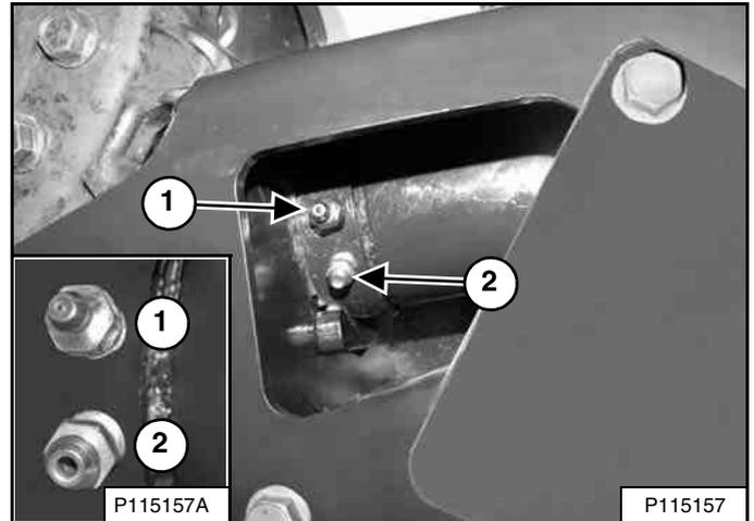
**NOTE:** This view shows the grease fittings on the right side of the loader. The fittings are in the opposite position on the left side of the loader. You **MUST** select the correct fitting for the task required. The grease fitting (Item 1) is used to add grease. The bleed fitting (Item 2) [Figure 278] is used to remove grease.
