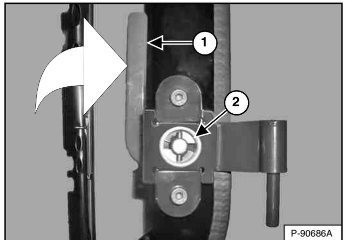
Install cast washers (Item 2) on door hinges taking care to match rectangular surfaces. Hold cast washer firmly against door and rotate latch (Item 1) [Figure 56] up to lock cast washer into position. (Bottom hinge shown.) (Plastic cap shown removed for visual clarity.)
