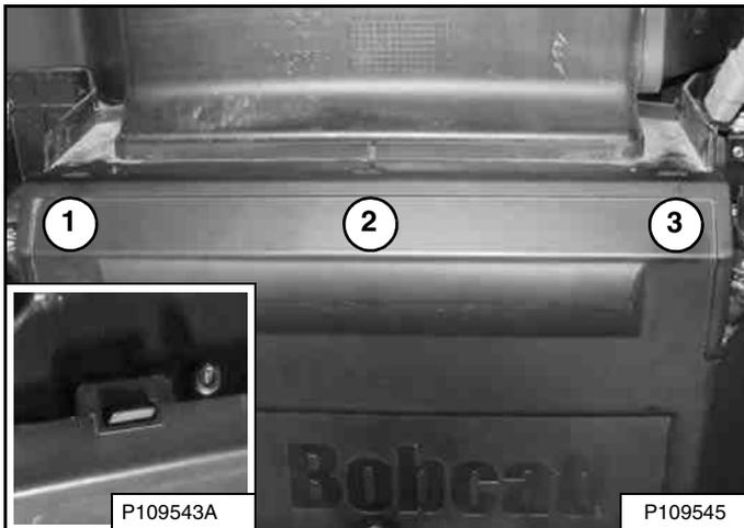
2. Push the cover up in three places (Items 1, 2, and 3) until the slots snap into place on the tabs. This slot (Inset) [Figure 202] is correctly fastened.
