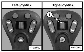
Move the Front Auxiliary Hydraulic switch (Item 1) [Figure 90] or [Figure 91] to the right or left to change direction of the auxiliary hydraulic fluid flow to the front quick couplers. If you move the switch halfway, the auxiliary functions move at approximately one-half speed. (EXAMPLE: Open and close grapple teeth.)
