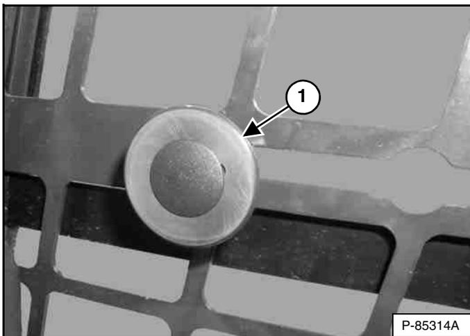
Pull the knob (Item 1) [Figure 29] and slide backward to open window. Release knob at cutout to lock in desired position. Pull the knob and slide forward to close window.
