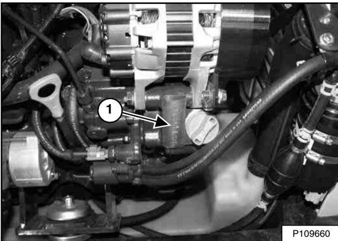
The engine serial number (Item 1) [Figure 2] is located on the side of the engine next to the oil fill cap.
