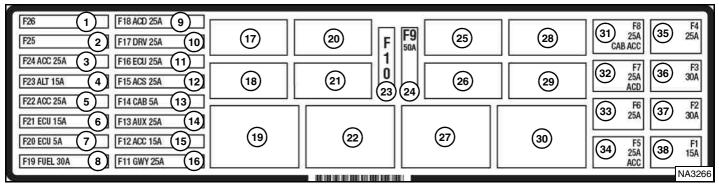
Fuse location and amperage ratings are shown in the table below and on the decal **[Figure 237]**. Relays are identified by the letter "R" in the AMP column.
