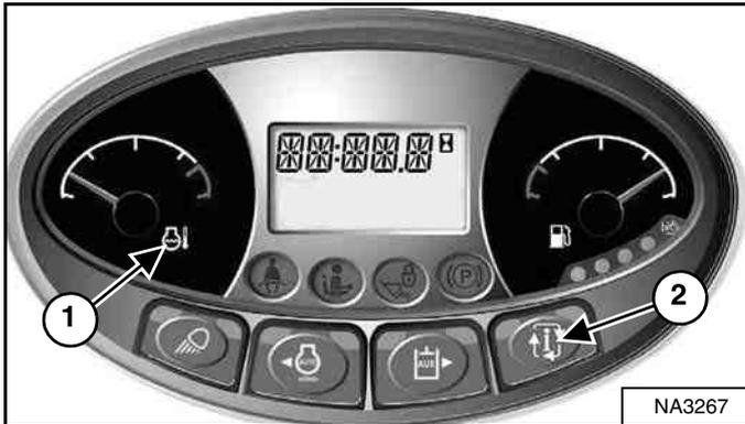
Frequently monitor the temperature and fuel gauges and BICS™ lights (all BICS™ lights must be OFF to operate loader) [Figure 133].
