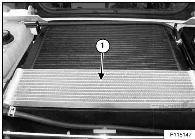
Use low air pressure or water pressure to clean the top of the fuel cooler (Item 1) [Figure 221].
