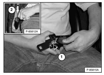
Connect the shoulder belt to the lap belt (Item 1). Pull the lap belt across to the right side of the seat and fasten (Item 2) [Figure 114].
