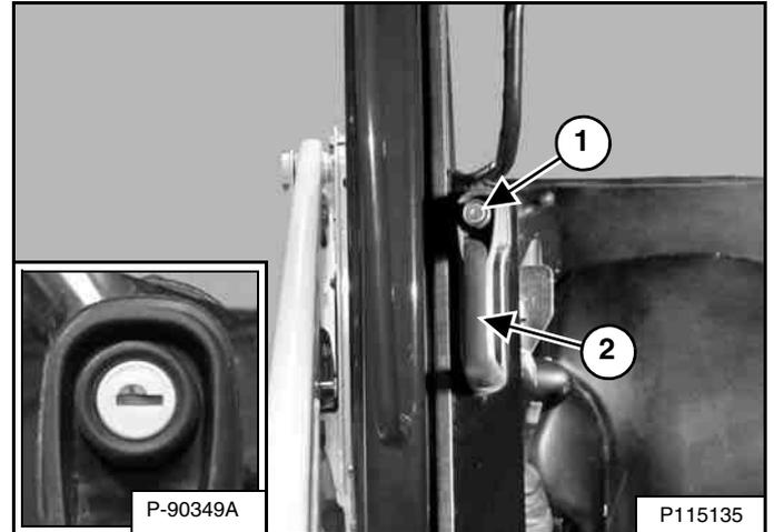
Push the knob (Item 1) and pull the handle (Item 2) to open the front door. A lock is provided in the knob (Inset) [Figure 30] to lock the front door when the loader is not in use.
