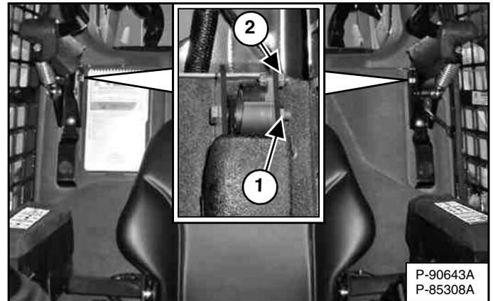
Use compressed air to clean any debris or dirt from the pivot parts. Do not lubricate. Inspect all mounting hardware. The correct hinge nut (both sides) (Item 1) torque is 34 – 38 N•m (25 – 28 ft-lb). The seat bar sensor nut (left side only) (Item 2) [Figure 170] torque is 6 – 8 N•m (50 – 70 in-lb).
