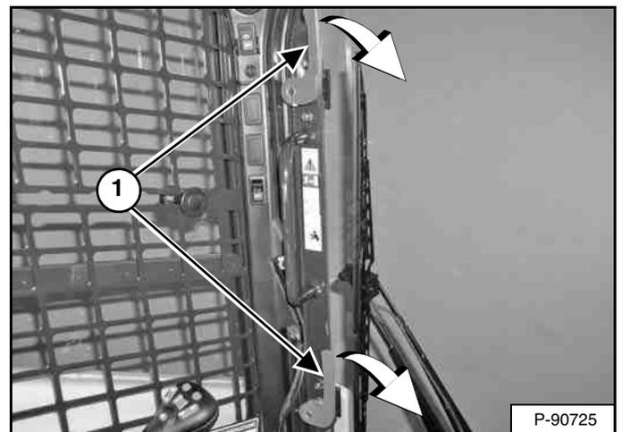
Turn both latches (Item 1) [Figure 52] down until they disengage from the door frame.
