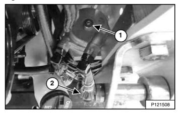
Open the air vent plug (Item 1) **[Figure 213]** on the fuel filter assembly three full turns.
