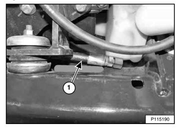
The oil drain hose (Item 1) **[Figure 217]** storage location is near the fuel tank fill. Route the oil drain hose through the opening.
