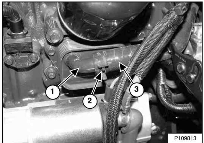
Remove the clamp (Item 2) and disconnect the hose (Item 3) from the engine oil cooler fitting (Item 1) [Figure 230].
