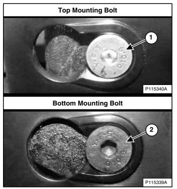
Position the drive belt shield over the drive belt shield mounting bolts. Slide the drive belt shield toward the front of the loader to fully seat the shield onto the top and bottom mounting bolts (Items 1 and 2) [Figure 298].
