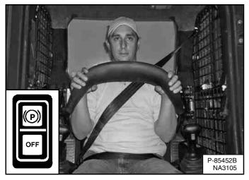
Lower the seat bar and engage the parking brake **[Figure 115]**.
