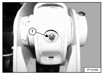
1. Lift Arm Pivot Pin (Both Sides) (2) [Figure 301].
