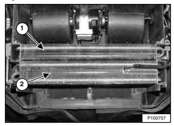
Use low pressure air or water to remove debris from the heater coil (Item 1) and evaporator (Item 2) [Figure 198].
