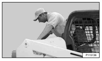
Exit through the rear of the operator cab [Figure 48].
