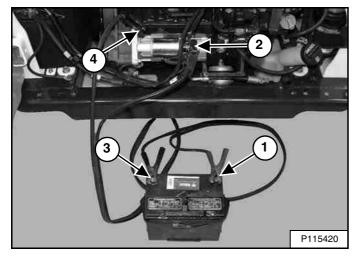
Connect the end of the first cable (Item 1) to the positive (+) terminal of the booster battery. Connect the other end of the same cable (Item 2) **[Figure 241]** to the positive (+) terminal on the engine starter.
