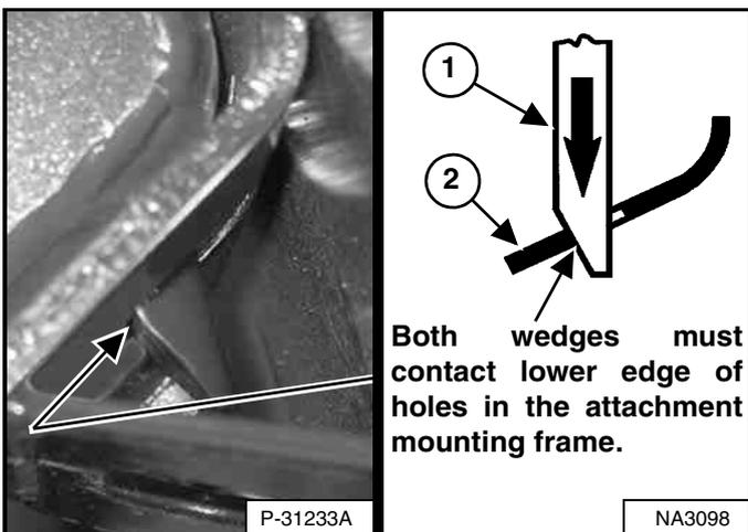
The wedges (Item 1) [Figure 311] must extend through the holes in the attachment mounting frame.
