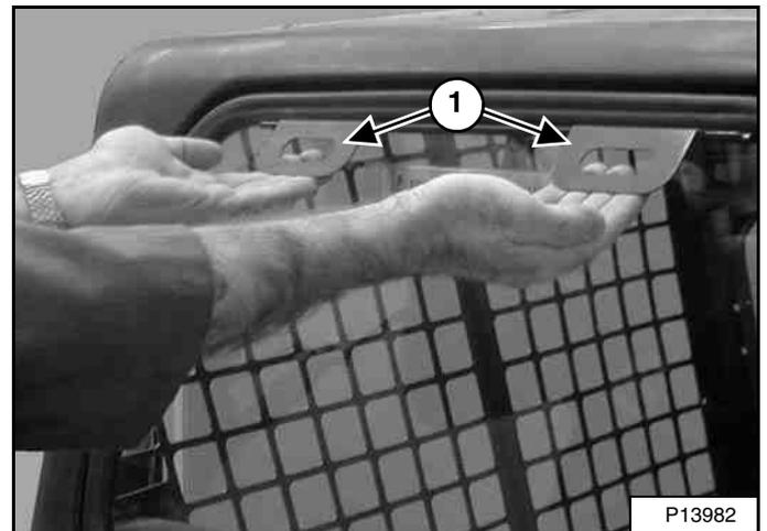
Pull both handles (Item 1) [Figure 51] up and out to remove the rear window.
