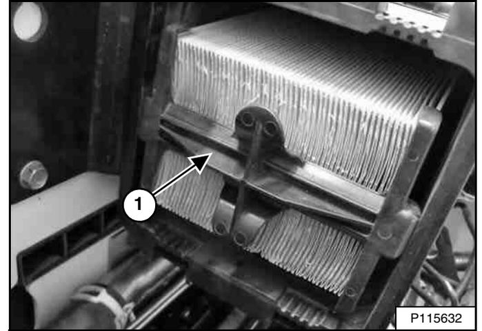
Remove the outer filter (Item 1) [Figure 206] and discard.
