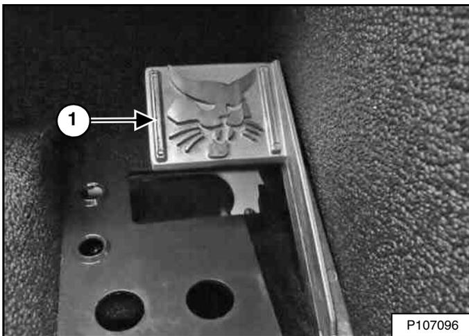
SJC equipped machines have a foot operated engine speed control pedal (Item 1) [Figure 41] in addition to the engine speed control knob. The pedal is located on the right side floor above the footrest.
