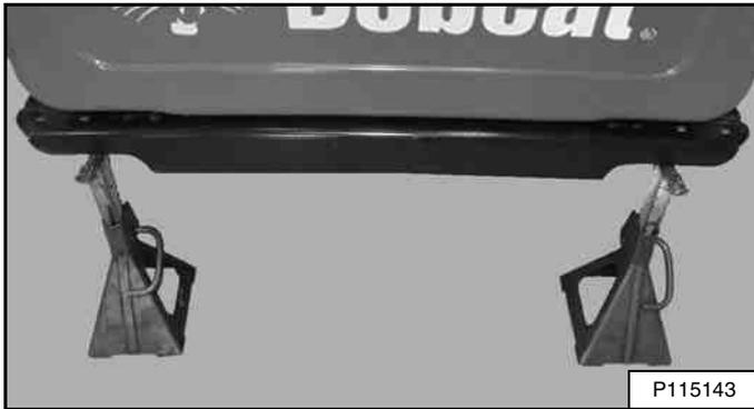
Install jackstands under the rear of the loader frame [Figure 185].
