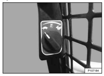
Set the engine speed control to the low idle position [Figure 117].
