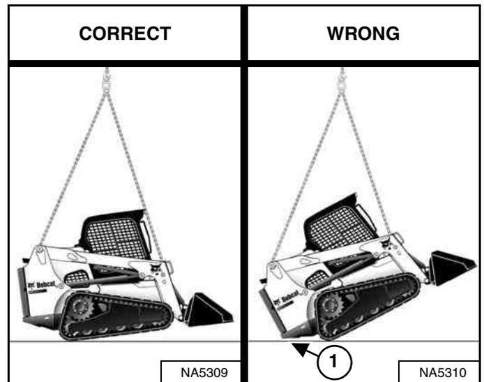
Attach cables or chains to lift eyes [Figure 165].
