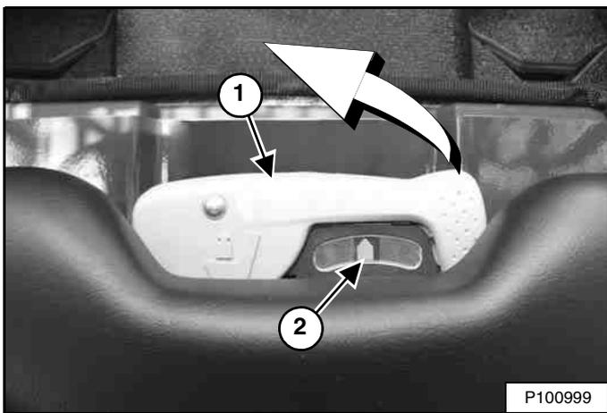
The lever (Item 1) is used to adjust the suspension response of the seat depending on the operator's weight. The optimum setting is achieved with the needle (Item 2) [Figure 110] centred in the gauge with the operator normally seated.
