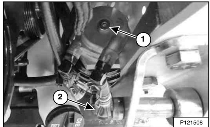
Open the air vent plug (Item 1) [Figure 213] on the fuel filter assembly three full turns.
