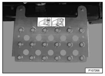
A maintenance platform **[Figure 220]** is available from your Bobcat dealer to facilitate access when cleaning the engine cooling system.
