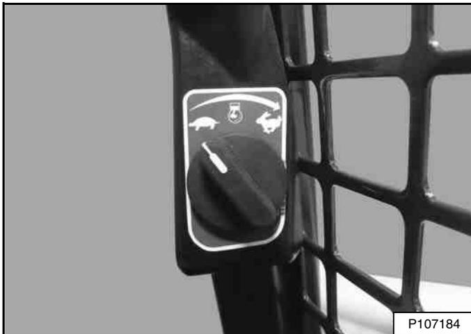
Set the engine speed control to the low idle position [Figure 127].
