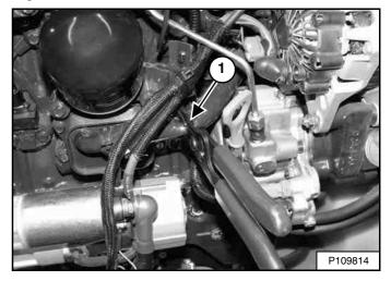
Pinch off the coolant hose attached to the engine oil cooler using a locking hose pinching plier (Item 1) **[Figure 229]** or similar tool.
