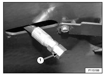
Remove the oil drain cap (Item 1) [Figure 218] from the oil drain hose and drain the oil into a container. Recycle or dispose of used oil in an environmentally safe manner.
