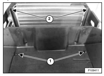
NOTE: The bosses (Item 1) fit inside the core supports (Item 2) [Figure 200] when the cover is installed. Deformity of the cover indicates they are out of position.
