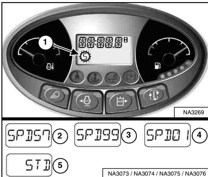
The Speed Management icon (Item 1) [Figure 69] will appear in the display and remain on until the Speed Management button is pressed again or the machine is turned off.
