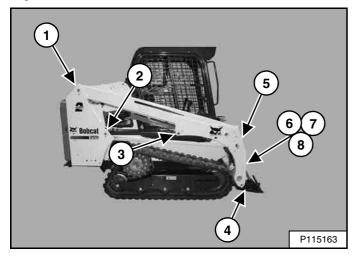
The grease fitting locations **[Figure 300]** are shown in more detail in the following figures.
