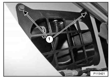
Remove the right side access cover bolts (Item 1) **[Figure 270]** and remove the access cover.
