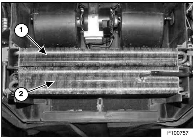
Use low pressure air or water to remove debris from the heater coil (Item 1) and evaporator (Item 2) [Figure 198].
