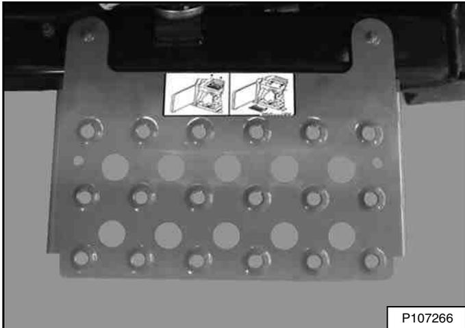
A maintenance platform [Figure 220] is available from your Bobcat dealer to facilitate access when cleaning the engine cooling system.
