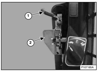
Pull the front door closed using the handle (Item 2) [Figure 31].
