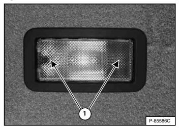
Push either side of the lens (Item 1) [Figure 34] to turn the light ON. Return the lens to the middle position to turn the light OFF.
