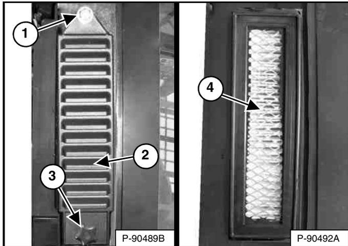
The fresh air filters are located behind the side windows outside the operator cab. (Right side shown) Remove the retaining screw (Item 3) and the filter cover (Item 2) [Figure 195]. (Lift arms shown raised for visual clarity.)
