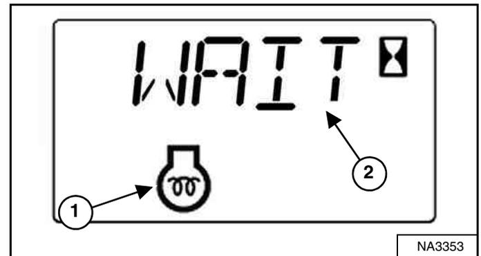
The machine will cycle the glow plugs automatically based on temperature. The engine preheat icon (Item 1) and the cycle time remaining or [WAIT] (Item 2) [Figure 119] are displayed in the data display.
