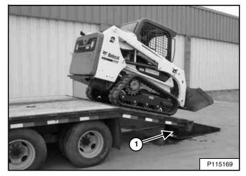
A loader with an empty bucket or no attachment must be loaded backward onto the transport vehicle [Figure 166].
