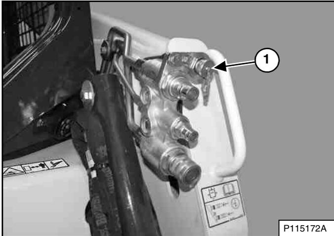
Connect the attachment electrical harness to the attachment control device (Item 1) [Figure 102].
