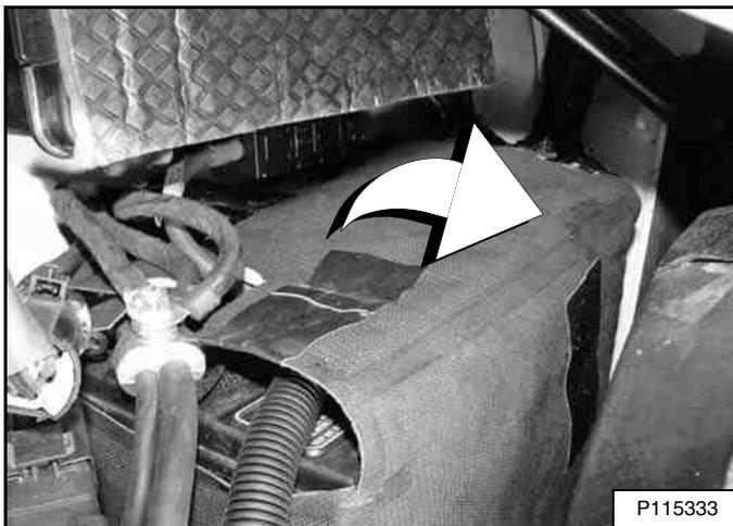
Open the top flap of the battery wrap to gain access to the battery terminals [Figure 244].
