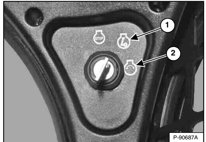
Turn the key switch to RUN (Item 1) [Figure 118]. The indicator lights on the left instrument panel will come ON briefly and the instrument panel / monitoring system will perform a self test.
