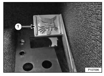
SJC equipped machines have a foot operated engine speed control pedal (Item 1) [Figure 41] in addition to the engine speed control knob. The pedal is located on the right side floor above the footrest.
