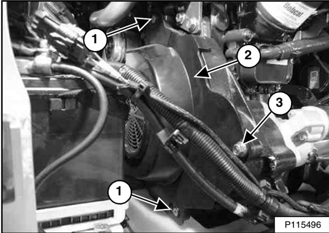
Remove the drive belt shield bolt (Item 3) [Figure 296].
