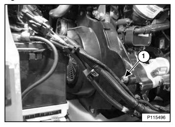
Install the drive belt shield bolt (Item 1) [Figure 299].
