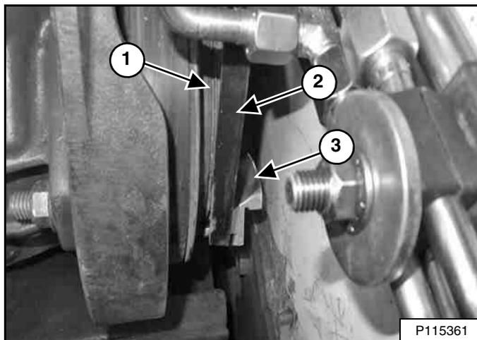
Install the belt on the air conditioning compressor pulley and start the belt (Item 2) and the belt tool (Item 3) on the front side of the hydraulic pump pulley (Item 1) [Figure 295].
