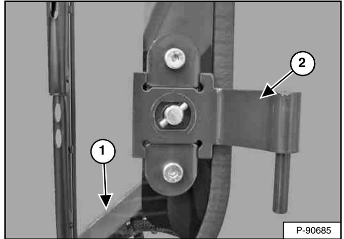
Orient the latches as shown (Item 1) and install the door hinges (Item 2) [Figure 55] on the door. (Bottom hinge shown.)
