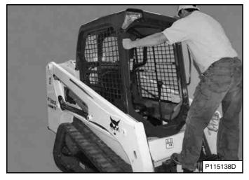
Use the bucket or attachment steps, grab handles, and safety treads (on the loader lift arms and frame) to get on and off the loader, maintaining a three-point contact at all times [Figure 107]. Do not jump.
