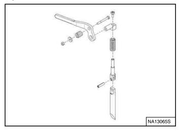
Inspect the mounting frame on the attachment and Bob-Tach, linkages, and wedges for excessive wear or damage **[Figure 315]**. Replace any parts that are damaged, bent, or missing. Keep all fasteners tight.
