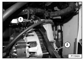
Use a prybar (Item 2) in the location shown to move the alternator until the top alternator mounting bolt (Item 1) **[Figure 289]** can be installed.
