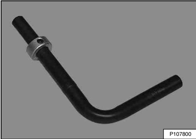
A bleed tool **[Figure 273]** is available and recommended to decrease track tension. The bleed tool will direct the flow of grease to aid in cleanup. See your Bobcat dealer to order a bleed tool.
