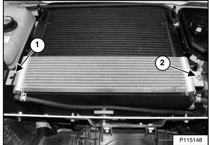
The area between the fuel cooler and the hydraulic fluid cooler and radiator assembly will require occasional cleaning. Remove the bolt (Item 2) and lift the fuel cooler up while sliding out of the bracket (Item 1) [Figure 226].
