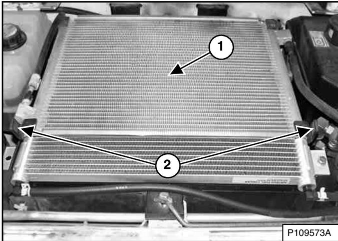
Use low air pressure or water pressure to clean the top of the air conditioning condenser (Item 1) [Figure 222].
