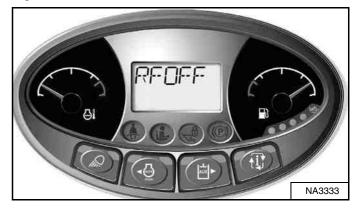
Reversing fan is disabled when the engine coolant or hydraulic fluid temperature is too high or too low.
