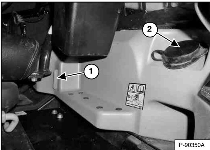
The washer fluid tank is located to the left of the operator seat. Check the fluid level in the sight gauge (Item 1). Remove the cap (Item 2) [Figure 33] to add washer fluid.
