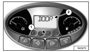
The LIFT AND TILT VALVE light (Item 1) **[Figure 184]** is OFF when the door is <u>closed</u>, the key switch is turned to RUN, the seat bar is lowered, and the PRESS TO OPERATE LOADER button is pressed.
