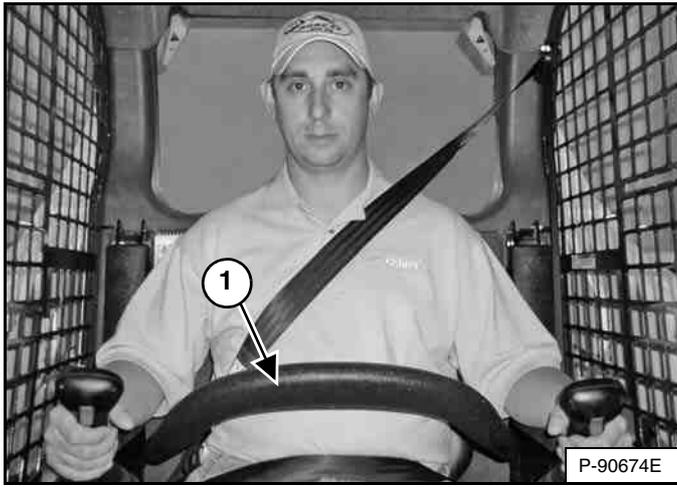
The Bobcat Interlock Control System (BICS™) has a pivoting seat bar with armrests (Item 1) [Figure 35]. The operator controls the use of the seat bar.
