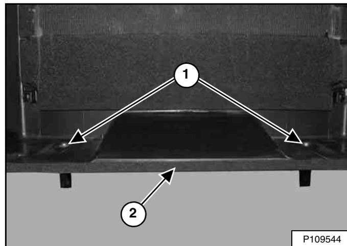
Clean the plenum drains (Item 1) [Figure 199] to ensure they are not plugged by debris.
