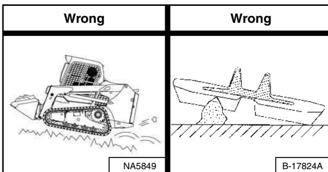
Avoid operating or turning on sharp objects such as jagged rocks, broken concrete, quarry materials, or scrap applications. This can cause cuts on the lug surface of the tracks [Figure 158].
