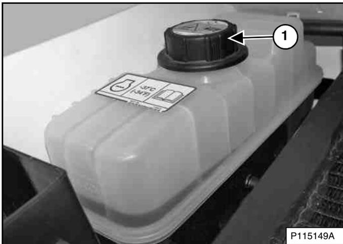
Remove the coolant fill cap (Item 1) [Figure 228].
