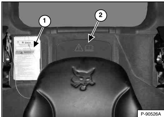
Read and understand the Operation & Maintenance Manual and the Operator's Handbook (Item 1) [Figure 108] before operating the loader.
