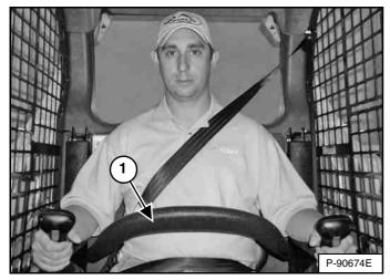
The seat bar restraint system has a pivoting seat bar with armrests (Item 1) [Figure 37].
