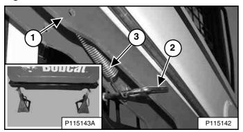
Put jackstands under the rear corners of the loader frame (Inset) [Figure 173].
