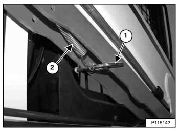
Raise the lift arm support device into the storage position and insert the retaining pin (Item 1) through the lift arm support device and the bracket. Hook the spring (Item 2) [Figure 178] to the retaining pin.
