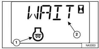
The machine will cycle the glow plugs automatically based on temperature. The engine preheat icon (Item 1) and the cycle time remaining or **[WAIT]** (Item 2) **[Figure 129]** are displayed in the data display.
