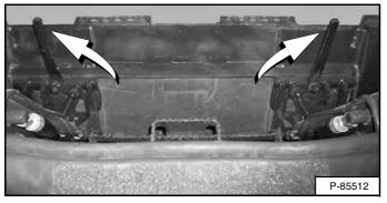
Pull the Bob-Tach levers up **[Figure 143]** until they are fully raised (wedges fully raised).
