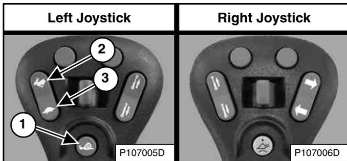
Adjust the speed percentage higher (Item 2) or lower (Item 3) [Figure 70] by pressing the Speed Control switch until the desired default setting is displayed.
