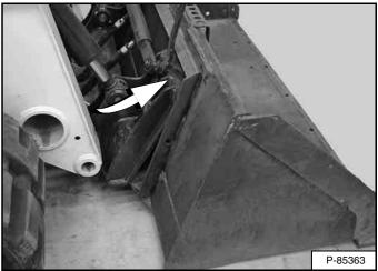
Drive the loader slowly forward until the top edge of the Bob-Tach is completely under the top flange of the bucket mounting frame **[Figure 147]** (or other attachment).
