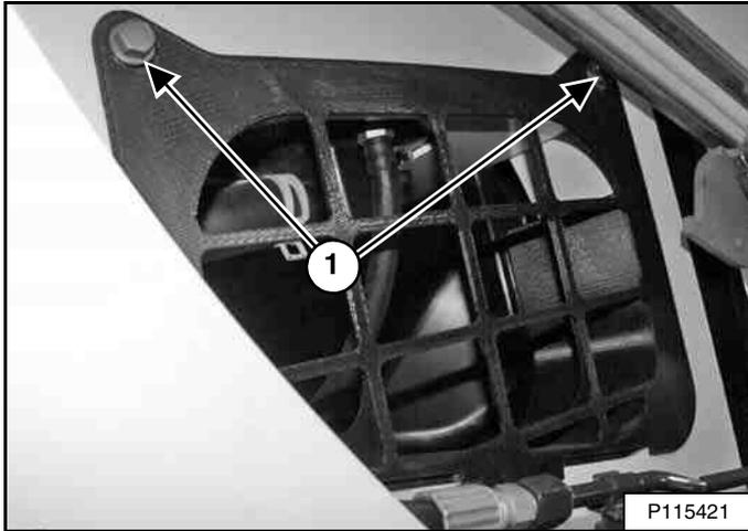
Remove the right side access cover bolts (Item 1) [Figure 270] and remove the access cover.
