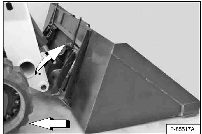
Tilt the Bob-Tach forward and drive the loader backward, away from the bucket or attachment [Figure 144].
