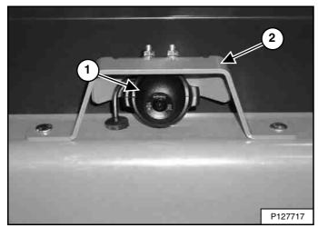
The rear camera (Item 1) is located inside a bracket (Item 2) **[Figure 23]** mounted on top of the rear door.
