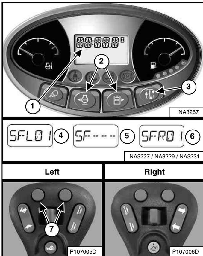
Press the Information button (Item 3) to cycle the data display until the steering drift compensation menu is displayed. The current steering drift compensation setting will appear in the data display (Item 1) [Figure 74].
