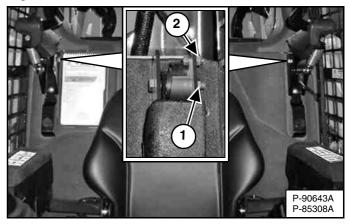
Use compressed air to clean any debris or dirt from the pivot parts. Do not lubricate. Inspect all mounting hardware. The correct hinge nut (both sides) (Item 1) torque is 34 - 38 N•m (25 - 28 ft-lb). The seat bar sensor nut (left side only) (Item 2) [Figure 170] torque is 6 - 8 N•m (50 - 70 in-lb).
