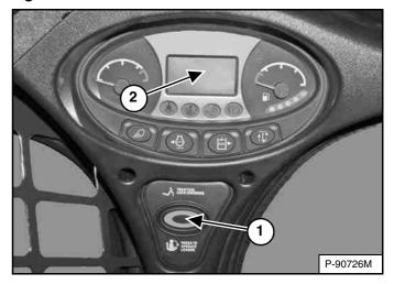
Press the PRESS TO OPERATE LOADER button (Item 1) **[Figure 126]** to activate the BICS<sup>™</sup> and to perform hydraulic and loader functions.
