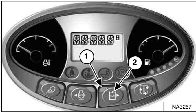
Press the Auxiliary Hydraulics button (Item 2) [Figure 89] once to activate the auxiliary hydraulics.
