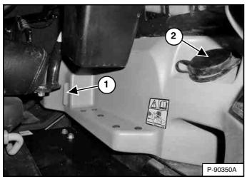
The washer fluid tank is located to the left of the operator seat. Check the fluid level in the sight gauge (Item 1). Remove the cap (Item 2) **[Figure 33]** to add washer fluid.
