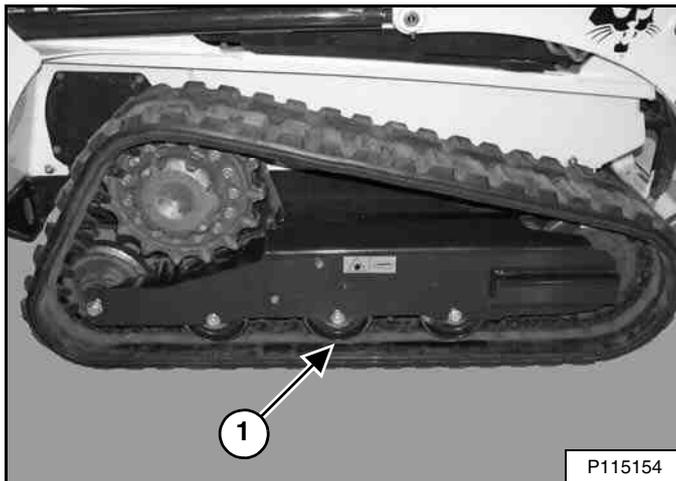
Raise one side of the loader and put jackstands at the front and rear of the loader frame so that the track is about 76 mm (3 in) off the ground [Figure 274]. Lower the loader to the jackstands. Be sure the jackstands do not touch the tracks.
