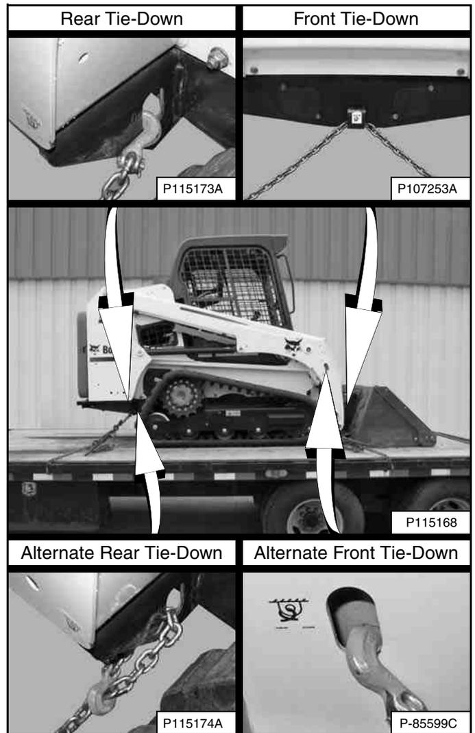
Use the following procedure to fasten the Bobcat loader to the transport vehicle to prevent the loader from moving during sudden stops, or when going up or down slopes [Figure 167].
