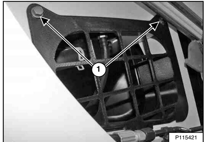
Remove the right side access cover bolts (Item 1) [Figure 259] and remove the access cover.
