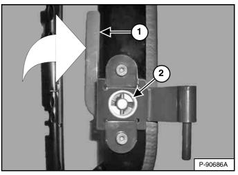
Install cast washers (Item 2) on door hinges taking care to match rectangular surfaces. Hold cast washer firmly against door and rotate latch (Item 1) **[Figure 56]** up to lock cast washer into position. (Bottom hinge shown.) (Plastic cap shown removed for visual clarity.)
