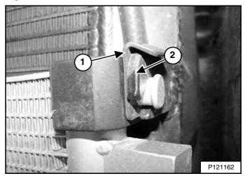
Ensure the air conditioning condenser is installed into the two slotted brackets (Item 2) **[Figure 224]**. (Right side shown.)
