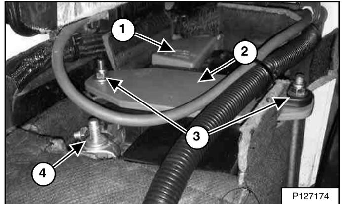
Connect the positive (+) cable (Item 1) [Figure 254]. Tighten the nut to 5,4 - 6,8 N•m (4 - 5 ft-lb) torque.
