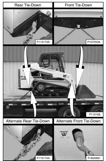
Use the following procedure to fasten the Bobcat loader to the transport vehicle to prevent the loader from moving during sudden stops, or when going up or down slopes [Figure 167].
