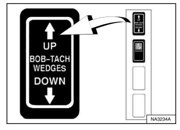
Push and <u>hold</u> BOB-TACH WEDGES "UP" switch (Right Switch Panel) **[Figure 149]** to make sure the levers are fully raised (wedges fully raised).
