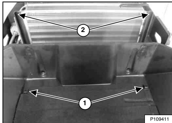
**NOTE:** The bosses (Item 1) fit inside the core supports (Item 2) [Figure 200] when the cover is installed. Deformity of the cover indicates they are out of position.
