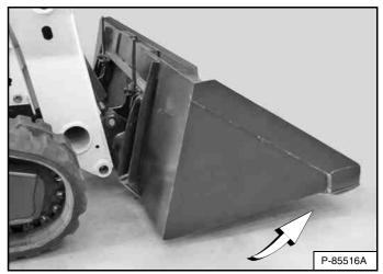
Tilt the Bob-Tach backward until the cutting edge of the bucket (or other attachment) is slightly off the ground **[Figure 140]**. This procedure will cause the bucket mounting frame to fit up against the front of the Bob-Tach.
