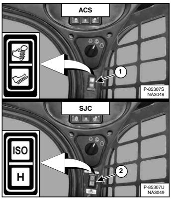
(ACS) Select hand control or foot pedal operation (Item 1) [Figure 125] if equipped with ACS.
