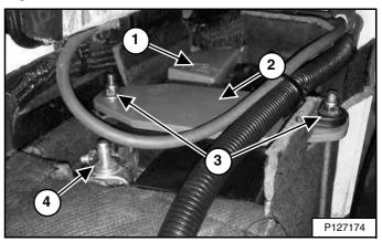
Connect the positive (+) cable (Item 1) [Figure 254]. Tighten the nut to  $5,4 - 6,8 \text{ N} \cdot \text{m} (4 - 5 \text{ ft-lb})$  torque.
