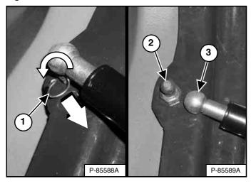
Rotate and pull the clip (Item 1) out of the gas spring socket. Pull the gas spring socket (Item 3) straight off the ball stud fitting (Item 2) [Figure 54].
