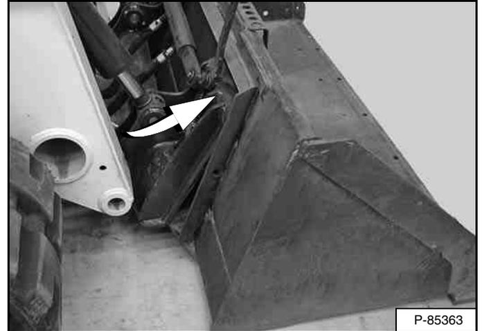
Drive the loader slowly forward until the top edge of the Bob-Tach is completely under the top flange of the bucket mounting frame [Figure 147] (or other attachment).
