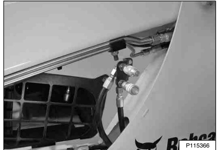
Move the Rear Auxiliary Hydraulic switch (Item 1) [Figure 95] or [Figure 96] to the right or left to change direction of the auxiliary hydraulic fluid flow to the rear quick couplers [Figure 97]. (Left side shown.) (EXAMPLE: Raise and lower rear stabilisers.) Release the switch to stop fluid flow.
