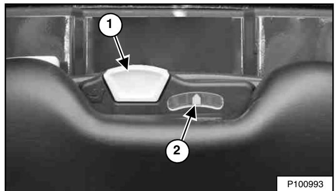
The lever (Item 1) is used to adjust the suspension response of the seat depending on the operator's weight. The optimum setting is achieved with the needle (Item 2) [Figure 112] centred in the gauge with the operator normally seated.
