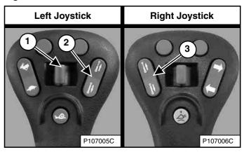
Additional switches (Items 1, 2, and 3) [Figure 104] or [Figure 105] are used to control some attachment functions through the attachment control device.
