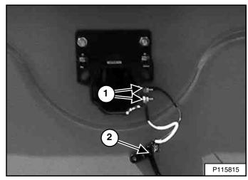
Inspect the back-up alarm electrical connections (Item 1) **[Figure 180]**, wire harness (Item 2) **[Figure 180]**, and back-up alarm switches (if equipped) (Item 1) **[Figure 181]** for tightness and damage. Repair or replace any damaged components.
