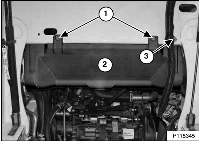
Remove the nut (Item 3) holding the operator cab electrical harness clamp and move the harness toward the front of the loader. Remove the bolts (Item 1) and remove the lower fan duct (Item 2) [Figure 267].
