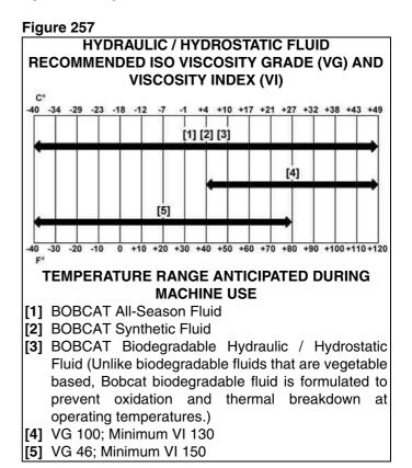
Bobcat hydraulic fluids are recommended for use in this machine. If Bobcat hydraulic fluid is not available, use a good quality hydraulic fluid meeting the viscosity grade and viscosity index shown in the chart [Figure 257].
