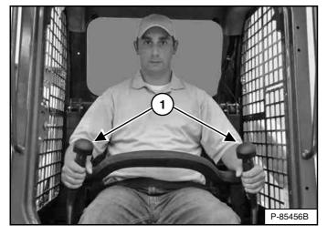
The steering levers (Item 1) **[Figure 58]** are on the left and right side in front of the seat.
