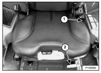
Pull the lever (Item 1) [Figure 109] up to adjust the angle of the seat back.
