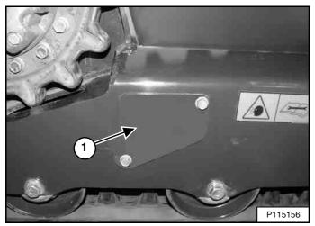
The track tension fittings used to adjust the track tension are located behind access covers (Item 1) [Figure 281]. (Right side shown.)
