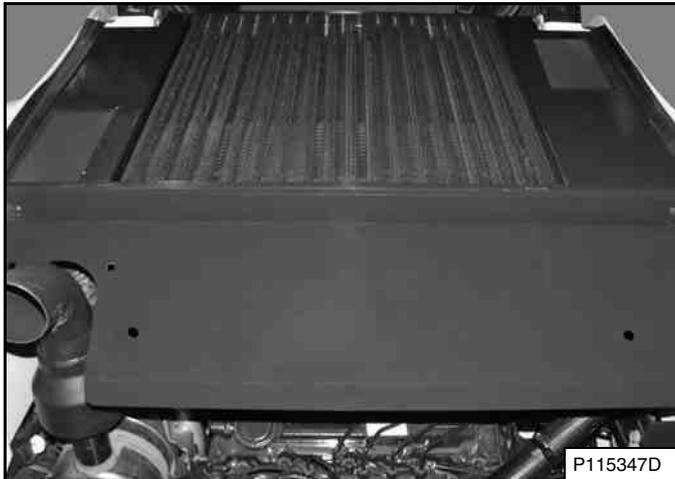
Lift and pull the rear grille backward to remove from the loader [**Figure 193**].
