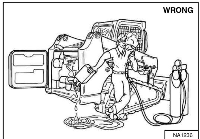
Use a clean, approved safety container to add fuel of the correct specification. Add fuel only in an area that has free movement of air and no open flames or sparks. **NO SMOKING** [Figure 210].
