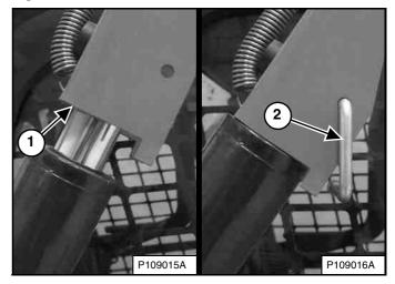
Raise the lift arms until the lift arm support device drops onto the lift cylinder rod (Item 1) [Figure 175].
