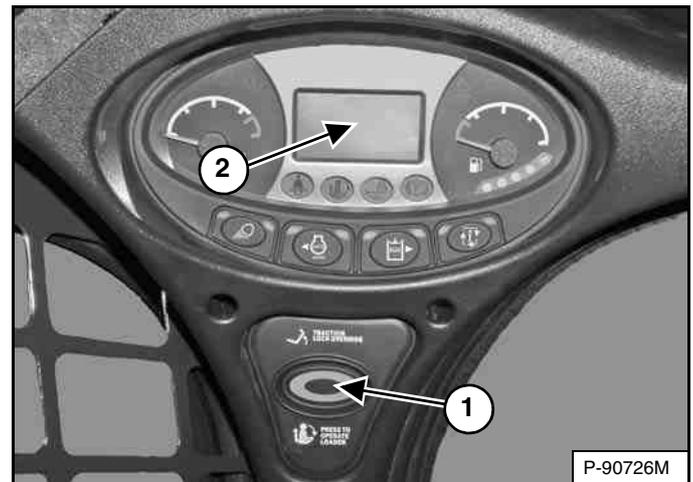
Press the PRESS TO OPERATE LOADER button (Item 1) [Figure 121] to activate the BICS™ and to perform hydraulic and loader functions.
