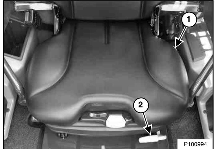
Pull the lever (Item 1) [Figure 111] up to adjust the angle of the seat back.
