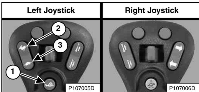
Press the button (Item 1) [Figure 68] on the left joystick once to engage Speed Management.
