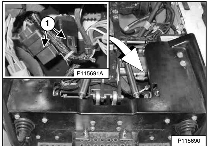
Two relays (Item 1) [Figure 236] for the loader lights are located under the operator cab on the left side of the loader. Stop the engine and raise the operator cab to access the relays. (See Raising on Page 138.)
