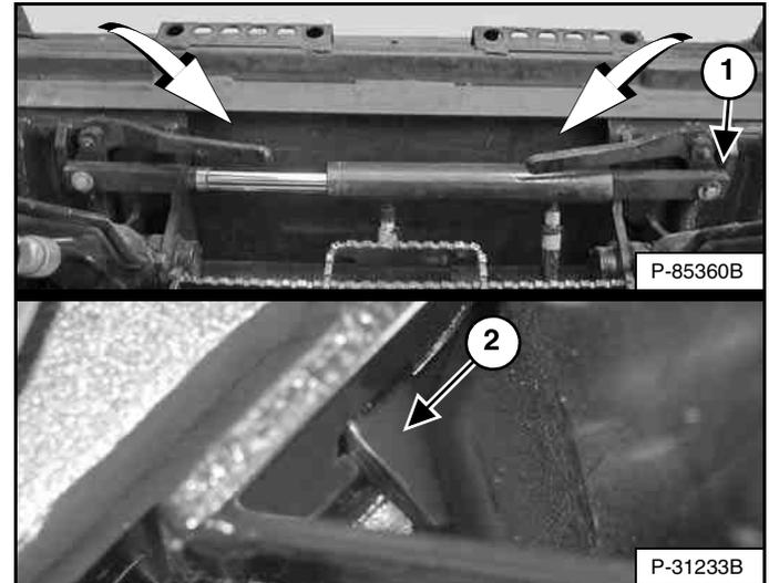
Push and hold BOB-TACH WEDGES “DOWN” switch (Right Switch Panel) [Figure 150] until levers are fully engaged in the locked position [Figure 151] (wedges fully extended through the attachment mounting frame holes).
