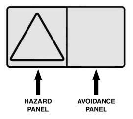
The format consists of the hazard panel(s) and the avoidance panel(s):
