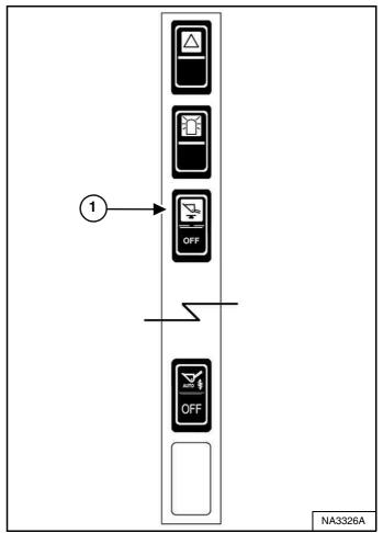
Press the top of the Bucket Positioning switch (Item 1) **[Figure 85]** on the left switch panel to engage the bucket positioning function. The amber light in the switch will turn ON.
