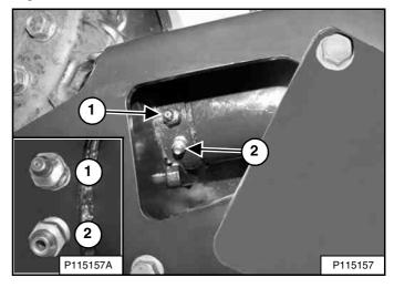
NOTE: This view shows the grease fittings on the right side of the loader. The fittings are in the opposite position on the left side of the loader. You MUST select the correct fitting for the task required. The grease fitting (Item 1) is used to add grease. The bleed fitting (Item 2) [Figure 278] is used to remove grease.
