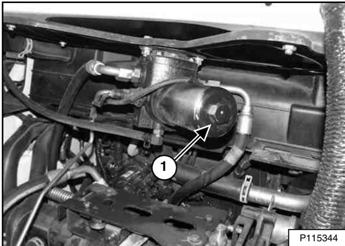
Put a suitable container below the filter housing and remove the filter housing (Item 1) [Figure 268].
