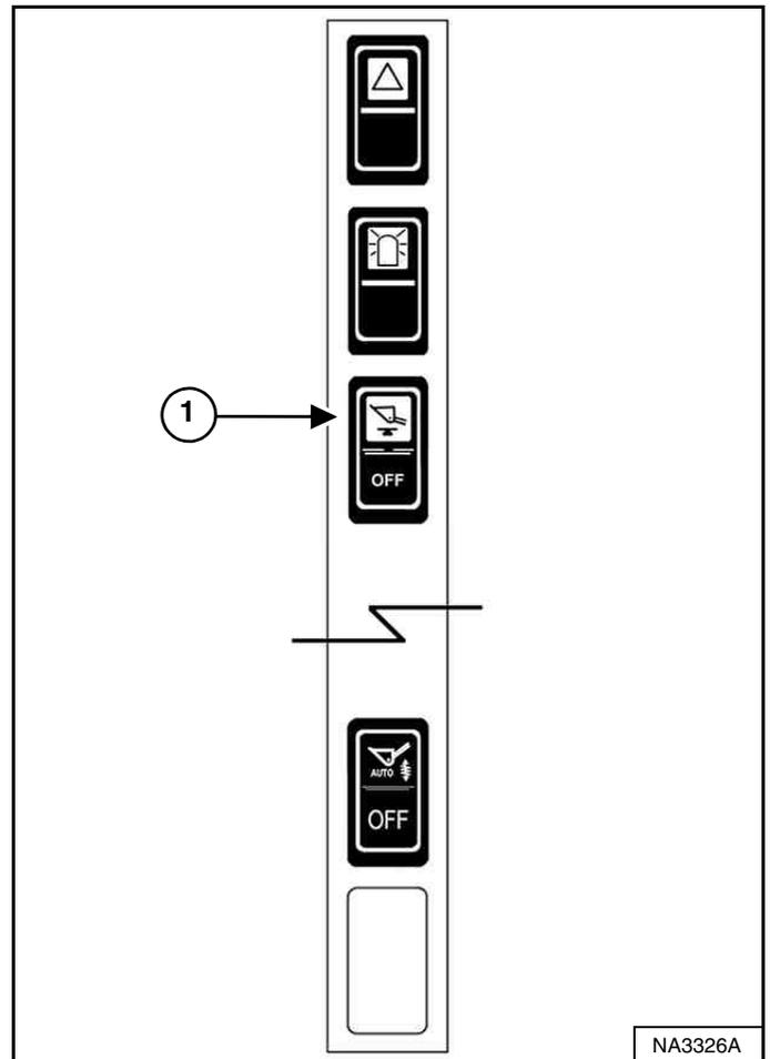
Press the top of the Bucket Positioning switch (Item 1) [Figure 85] on the left switch panel to engage the bucket positioning function. The amber light in the switch will turn ON.
