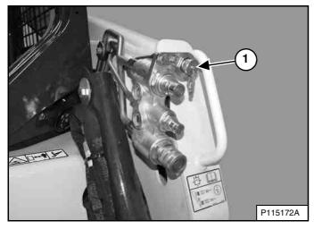
Connect the attachment electrical harness to the attachment control device (Item 1) [Figure 102].
