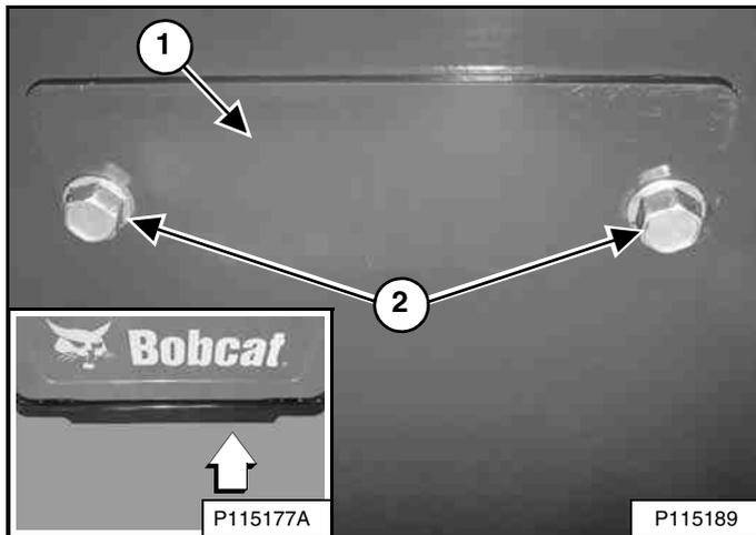
The oil drain hose is located behind a cover (Item 1) under the rear of the loader (Inset) [Figure 216].
