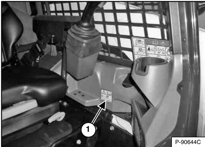
Inspect for damaged or missing back-up alarm decal (Item 1) [Figure 179]. Replace if required.
