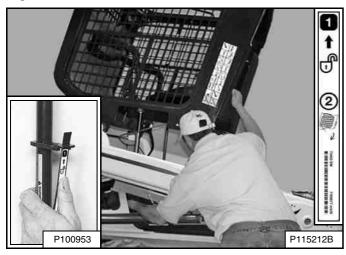
Pull down on the bottom of the operator cab until stopped by the latching mechanism **[Figure 188]**.
