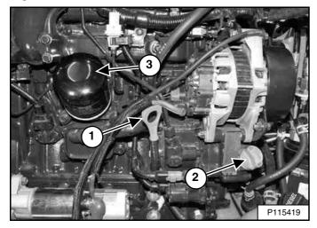
Remove the oil filter (Item 3) [Figure 219] and clean the filter base.
