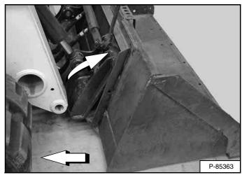
Tilt the Bob-Tach forward and drive the loader backward, away from the bucket or attachment [Figure 153].
