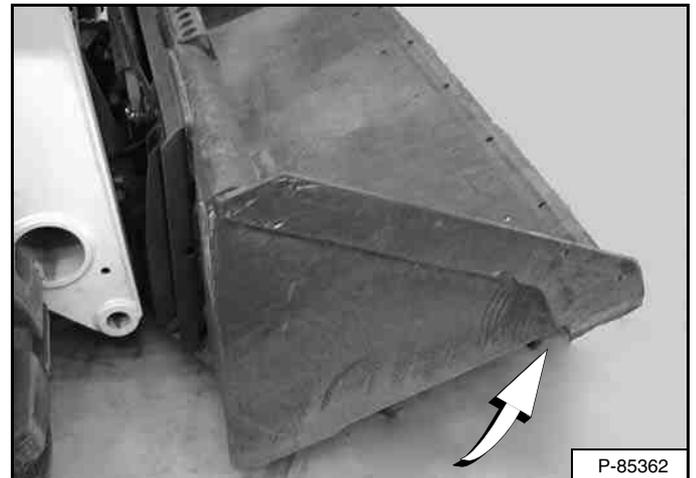
Tilt the Bob-Tach backward until the cutting edge of the bucket (or other attachment) is slightly off the ground [Figure 148]. This procedure will cause the bucket mounting frame to fit up against the front of the Bob-Tach.
