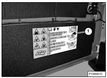
The Service Checklist And Schedule (Item 1) [Figure 106] is located inside the rear door of the loader.
