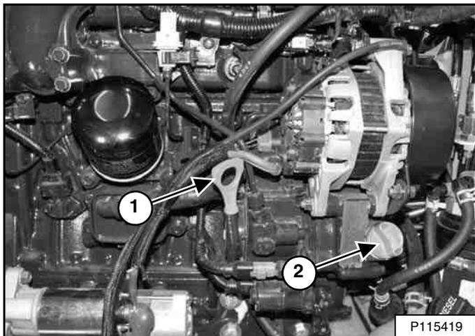
Park the loader on a level surface. Stop the engine. Open the rear door and remove the dipstick (Item 1) [Figure 214].
