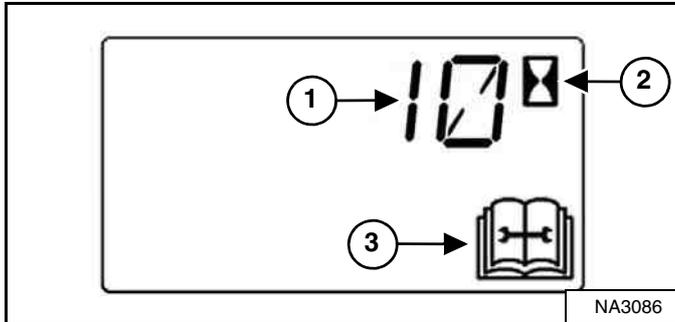
During machine operation, a 2 beep alarm will sound when there are less than 10 hours until the next planned maintenance.
