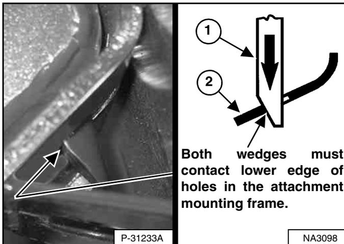
The wedges (Item 1) [Figure 314] must extend through the holes in the attachment mounting frame.
