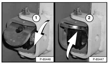
Move the door stop into the engaged position (Item 1) to hold the door open. Move the door stop up (Item 2) **[Figure 191]** to allow the door to close.
