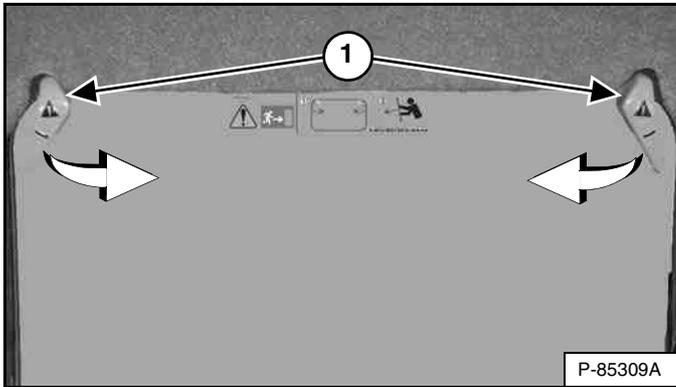
Turn both latches (Item 1) [Figure 45] in until they disengage from the window frame.
