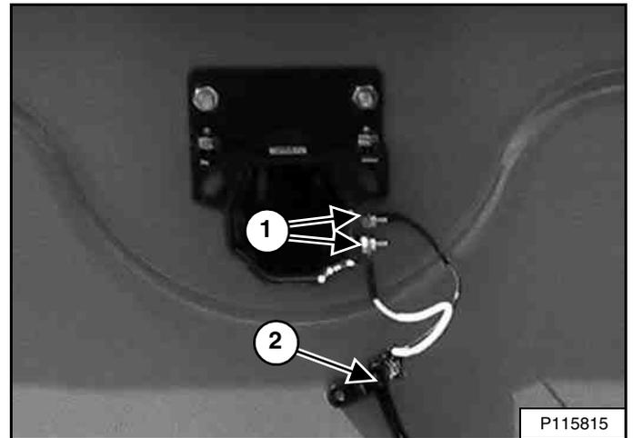
Inspect the back-up alarm electrical connections (Item 1) [Figure 180], wire harness (Item 2) [Figure 180], and back-up alarm switches (if equipped) (Item 1) [Figure 181] for tightness and damage. Repair or replace any damaged components.
