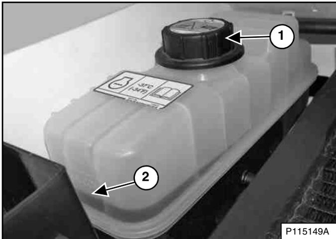
Remove the coolant fill cap (Item 1) [Figure 231] to drain the coolant faster.
