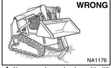
Never work on loader with lift arms up unless lift arms are held by an approved lift arm support device. Replace if damaged. Never modify equipment or add attachments not approved by Bobcat Company.
