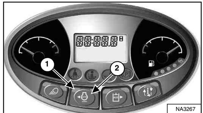
Press the button (Item 2) to engage auto idle. The light (Item 1) [Figure 42] is ON.
