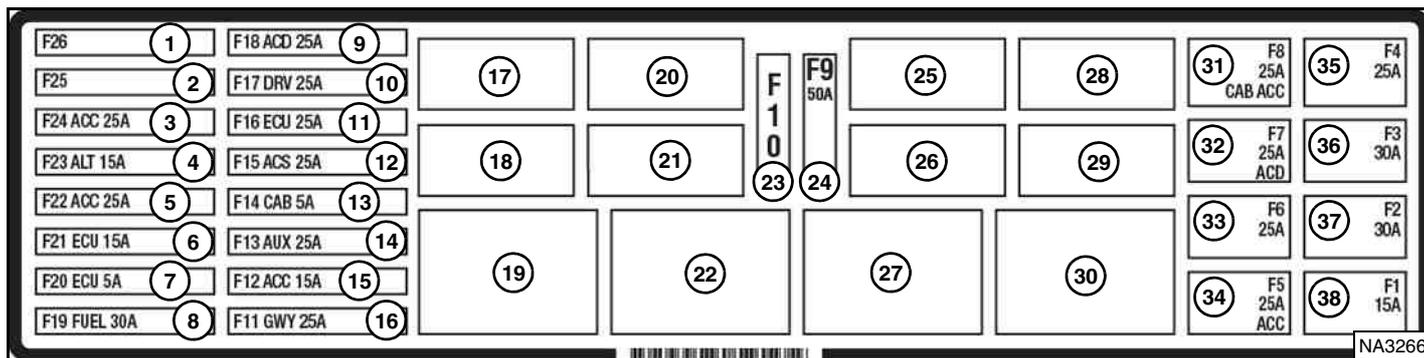
Fuse location and amperage ratings are shown in the table below and on the decal [Figure 237]. Relays are identified by the letter “R” in the AMP column.
