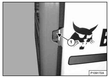
Reach into the slot on the right side of the rear door and pull the latch handle (Item 1) **[Figure 190]**. Pull the rear door open.
