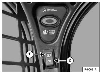
Press the top of the switch (Item 1) **[Figure 38]** to engage the parking brake. The red light in the switch will turn ON. The traction drive system is locked.
