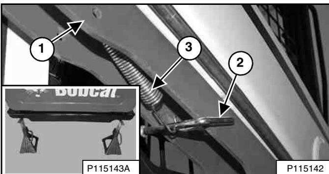
Put jackstands under the rear corners of the loader frame (Inset) [Figure 173].
