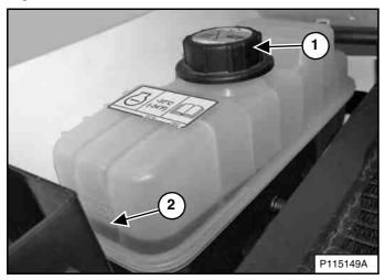
Coolant must be between the top and bottom level markers (Item 2) **[Figure 227]** when the engine is cold.
