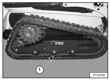
Raise one side of the loader and put jackstands at the front and rear of the loader frame so that the track is about 76 mm (3 in) off the ground **[Figure 274]**. Lower the loader to the jackstands. Be sure the jackstands do not touch the tracks.
