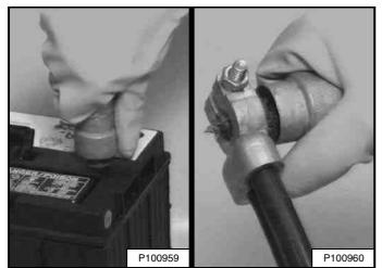
Always clean the battery terminals and cable ends when installing a new or used battery [Figure 253].
