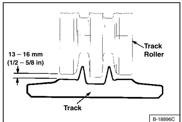
DO NOT put your fingers into the pinch points between the track and the roller. Use a 13 – 16 mm (1/2 – 5/8 in) bolt, dowel or block to check the gap [Figure 275] and [Figure 276].
