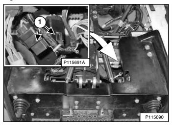
Two relays (Item 1) **[Figure 236]** for the loader lights are located under the operator cab on the left side of the loader. Stop the engine and raise the operator cab to access the relays. (See Raising on Page 138.)
