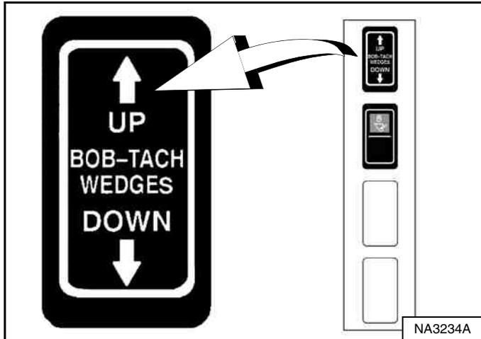
Push and hold BOB-TACH WEDGES “UP” switch (Right Switch Panel) [Figure 149] to make sure the levers are fully raised (wedges fully raised).
