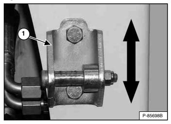
The door latch striker (Item 1) **[Figure 192]** can be adjusted up or down for alignment with the door latch.
