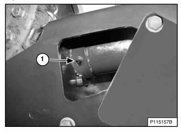
Add grease to the track tension fitting (Item 1) [Figure 282] until the track adjustment is correct [Figure 275] and [Figure 276].
