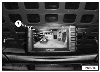
The camera display is located above the front door [Figure 21].
