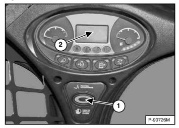
Press the PRESS TO OPERATE LOADER button (Item 1) **[Figure 131]** to activate the BICS<sup>™</sup> and to perform hydraulic and loader functions.
