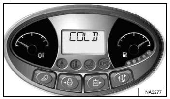
The engine controller will not allow full engine speed and torque when the engine temperature is too low. The following indications and actions are performed automatically by the engine controller:
