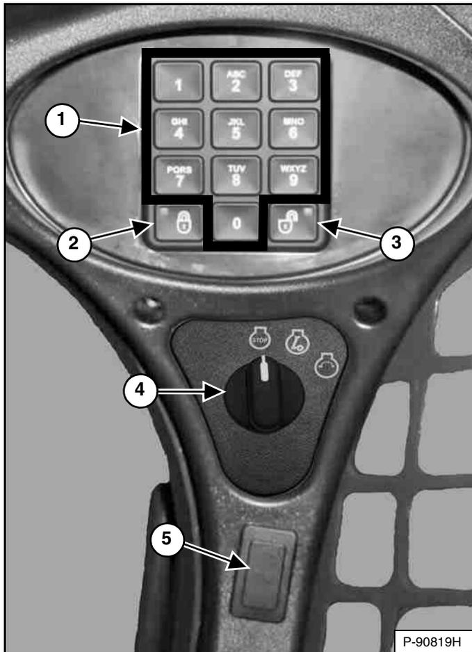
This machine may be equipped with a Keyless Start Panel [Figure 14].
