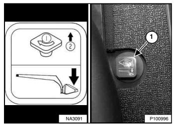
The lift arm bypass control (Item 1) **[Figure 43]**, located to the right of the operator's seat, is used to lower the lift arms if the lift arms cannot be lowered during normal operations.
