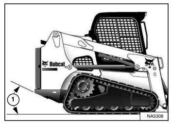
NOTE: The loader should be lifted as close to horizontal as possible, but at no time should the angle of the suspended loader exceed the departure angle (Item 1) [Figure 164] provided in the specifications section. (See Machine Dimensions on Page 220.) Figure 165
