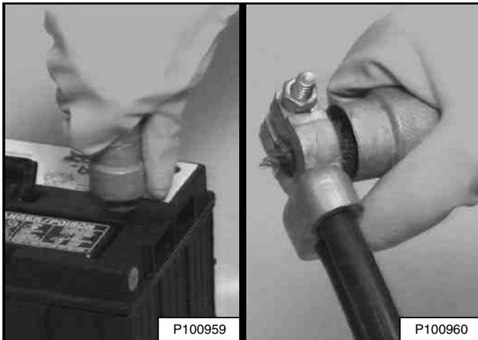
Always clean the battery terminals and cable ends when installing a new or used battery [Figure 247].
