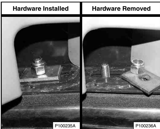
Remove the nuts and washers [Figure 186] (both sides) at the front corners of the operator cab.
