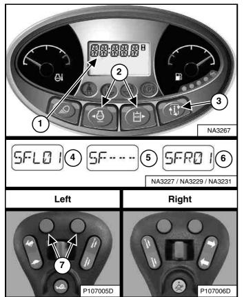
Press the Information button (Item 3) to cycle the data display until the steering drift compensation menu is displayed. The current steering drift compensation setting will appear in the data display (Item 1) [Figure 74].
