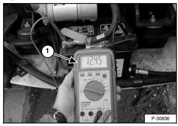
The simplest and most common check to determine battery state of charge is to use a digital multimeter or voltmeter (Item 1) [Figure 240].
