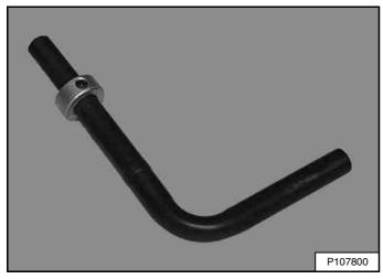
A bleed tool **[Figure 273]** is available and recommended to decrease track tension. The bleed tool will direct the flow of grease to aid in cleanup. See your Bobcat dealer to order a bleed tool.
