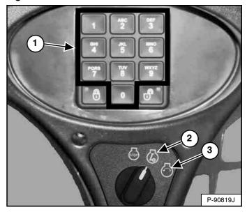
Turn the key switch to RUN (Item 2). The indicator lights on the left instrument panel will come ON briefly and the instrument panel / monitoring system will perform a self test. Use the numeric keypad (Item 1) [Figure 123] to enter the password.
