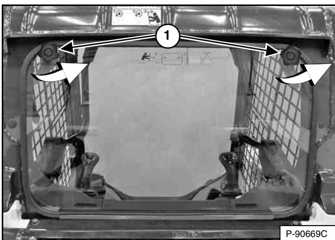
A kit is available to allow removal of the latch equipped rear window from outside the machine without tools. See your Bobcat dealer for availability.
