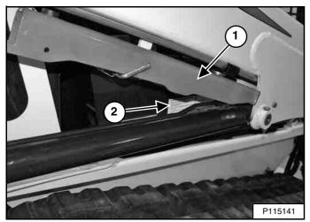
The lift arm support device (Item 1) **[Figure 172]** is used to support the lift arms while working on a machine with the lift arms up.
