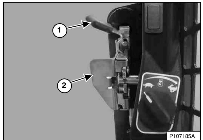
Pull the front door closed using the handle (Item 2) [Figure 31].
