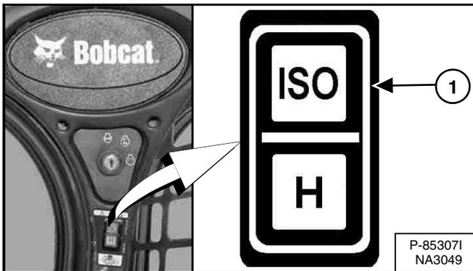
Select the 'ISO' control pattern by pressing the top of the switch (Item 1) [Figure 60].
