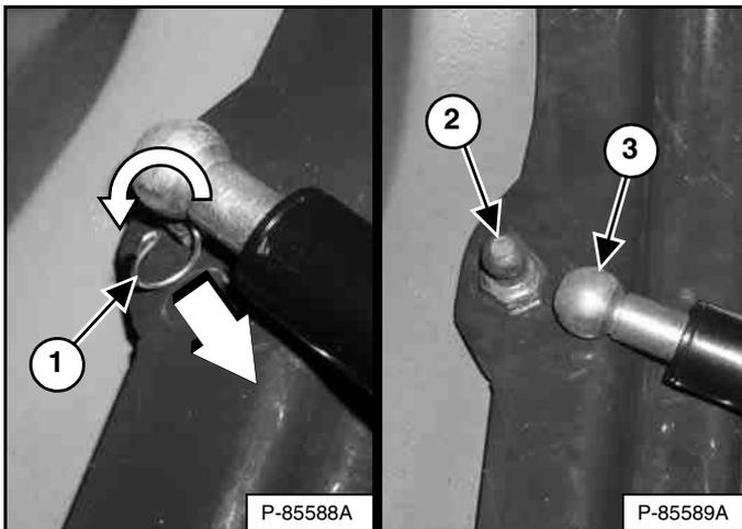
Rotate and pull the clip (Item 1) out of the gas spring socket. Pull the gas spring socket (Item 3) straight off the ball stud fitting (Item 2) [Figure 54].
