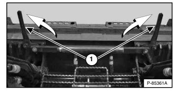
Push and <u>hold</u> BOB-TACH WEDGES "UP" switch (Right Switch Panel) [Figure 145] until levers (Item 1) [Figure 146] are fully raised (wedges fully raised).
