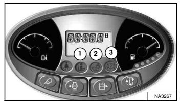
There are three display lights (Items 1, 2, and 3) **[Figure 36]** located on the left instrument panel that must be OFF to fully operate the machine.
