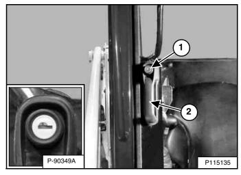
Push the knob (Item 1) and pull the handle (Item 2) to open the front door. A lock is provided in the knob (Inset) [Figure 30] to lock the front door when the loader is not in use.
