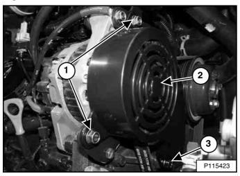
Remove the alternator belt shield mounting nuts and bolts (Item 1). Remove the mounting bolt (Item 3) **[Figure 287]**.
