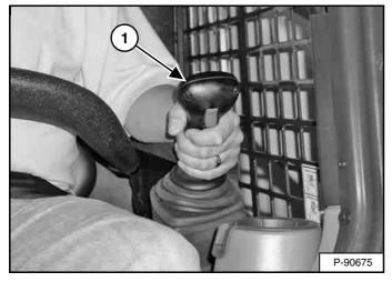
The joystick that controls drive and steering is on the left side in front of the seat (Item 1) **[Figure 61]**.
