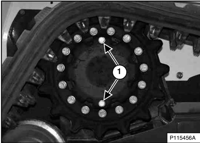
Park the loader so that the plugs (Item 1) [Figure 285] in the hydrostatic drive motor are at the top and the bottom.
