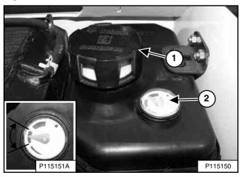
Check the fluid level in the sight gauge (Item 2). Keep the fluid level within the operating range (Inset) [Figure 256].
