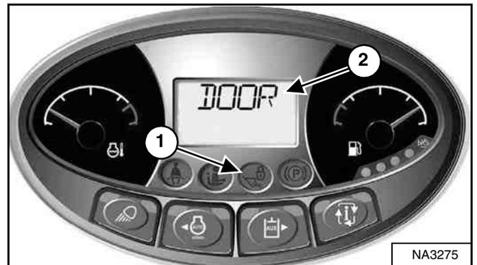
The LIFT AND TILT VALVE light (Item 1) [Figure 184] is OFF when the door is closed, the key switch is turned to RUN, the seat bar is lowered, and the PRESS TO OPERATE LOADER button is pressed.
