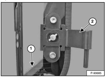
Orient the latches as shown (Item 1) and install the door hinges (Item 2) **[Figure 55]** on the door. (Bottom hinge shown.)
