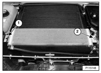
The area between the fuel cooler and the hydraulic fluid cooler and radiator assembly will require occasional cleaning. Remove the bolt (Item 2) and lift the fuel cooler up while sliding out of the bracket (Item 1) [Figure 226].
