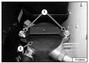
Loosen the bolts (Item 1) and rotate the filter cap (Item 2) **[Figure 264]** anticlockwise until the cap clears the bolts.
