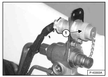
You will need the 14-Pin Attachment Control Device kit (Item 1) **[Figure 103]** to operate early model attachments. See your Bobcat loader dealer.
