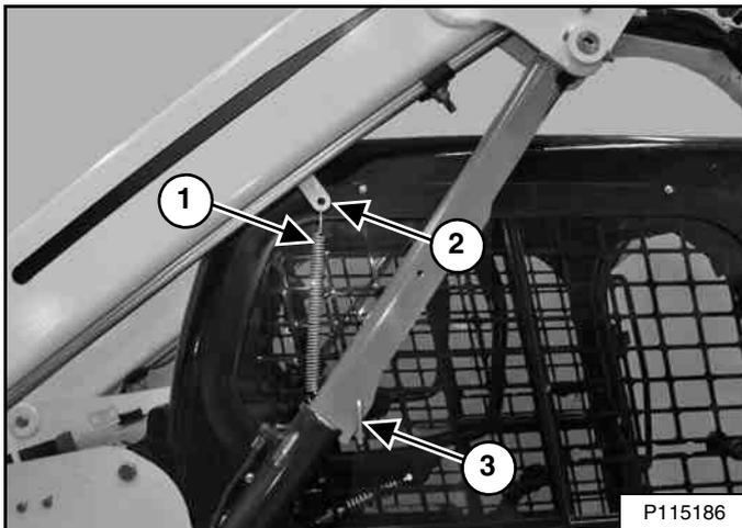
Remove the retaining pin (Item 3) [Figure 176] from the lift arm support device.
