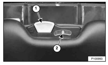
The lever (Item 1) is used to adjust the suspension response of the seat depending on the operator's weight. The optimum setting is achieved with the needle (Item 2) **[Figure 112]** centred in the gauge with the operator normally seated.
