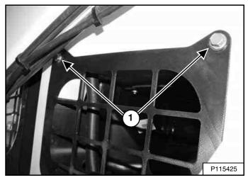
Remove the left side access cover bolts (Item 1) [Figure 261] and remove the access cover.
