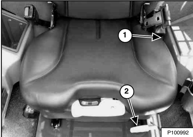
Pull the lever (Item 1) [Figure 109] up to adjust the angle of the seat back.
