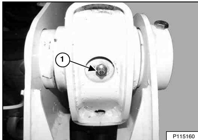
1. Lift Arm Pivot Pin (Both Sides) (2) [Figure 301].
