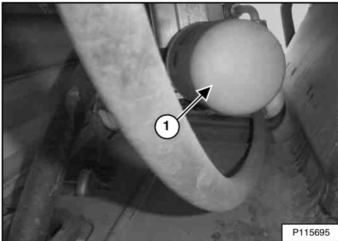
Put a suitable container below the filter, remove the filter (Item 1) [Figure 271], and clean the filter base.
