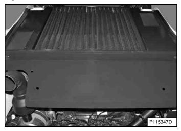
Lift and pull the rear grille backward to remove from the loader [Figure 193].
