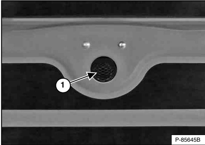
The back-up alarm (Item 1) [Figure 57] is located on the inside of the rear door.
