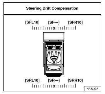
Steering drift compensation contains a total of 21 settings. Steering drift compensation can be set to any point from NEUTRAL to [SFL10] or [SRL10] left, and from NEUTRAL to [SFR10] or [SRR10] right. [SF---] or [SR---] is displayed when set for NEUTRAL [Figure 73].
