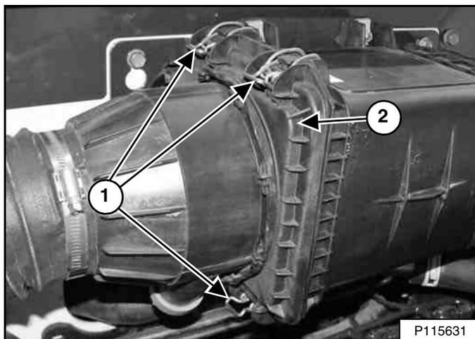
Open four latches (Item 1) and move the cover (Item 2) [Figure 205] out of the way. (One latch is not visible in the photo.)
