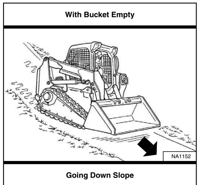
With a full bucket, go up or down the slope with the heavy end toward the top of the slope [Figure 159] and [Figure 160].
