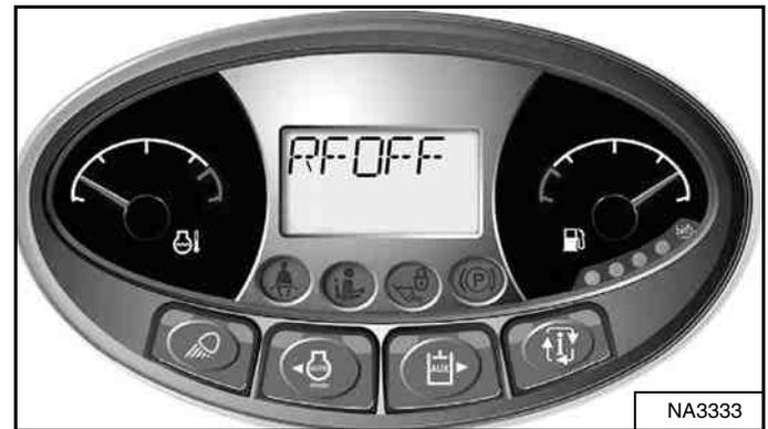
Reversing fan is disabled when the engine coolant or hydraulic fluid temperature is too high or too low.
