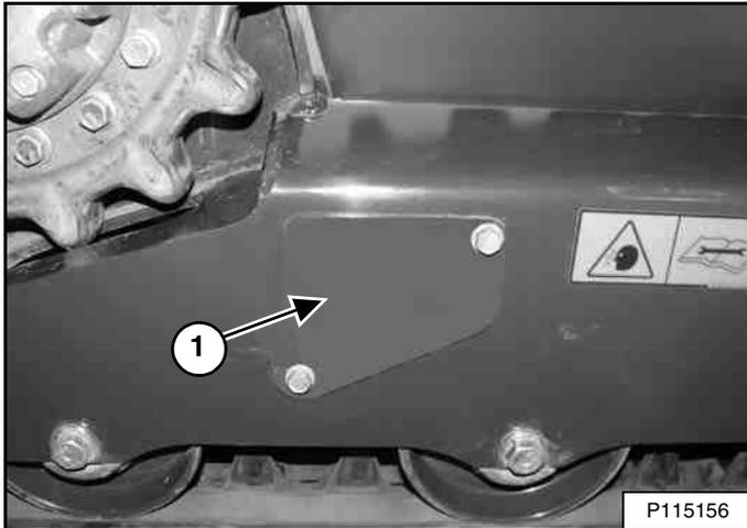
The grease fittings used to adjust the track tension are located behind access covers (Item 1) [Figure 277]. (Right side shown.)
