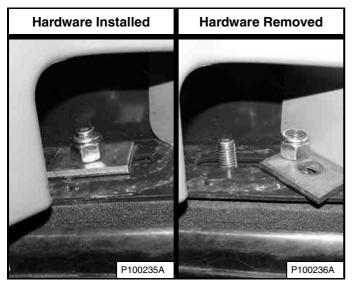
Remove the nuts and washers [Figure 186] (both sides) at the front corners of the operator cab.
