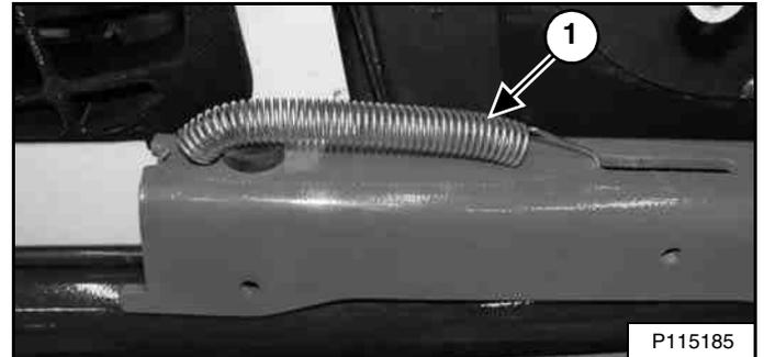
Lower the lift arm support device to the top of the lift cylinder. Hook the free end of the spring (Item 1) [Figure 174] to the lift arm support device to prevent interference with lift arm support device engagement.
