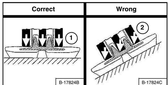
The track carriage components will wear faster when operated on a slope. When the machine is operated on a level surface, the weight of the machine is distributed throughout the entire surface of the rollers to the tracks (Item 1). When operated on a slope, the weight is directed to the edge of the rollers and against the lugs of the track (Item 2) [Figure 156] which causes increased wear.
