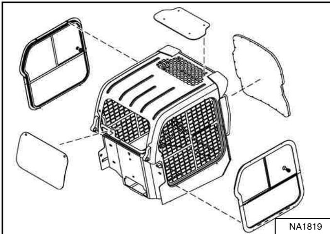
Available for special applications to prevent flying debris and objects from entering the cab. Kit includes 19,1 mm (0.75 in) thick laminated polycarbonate front door, polycarbonate side windows, and polycarbonate rear window [Figure 5].
