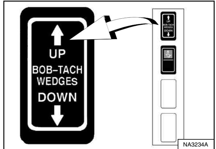
Push and hold BOB-TACH WEDGES "UP" switch (Right Switch Panel) [Figure 152] until levers are fully raised (wedges fully raised).
