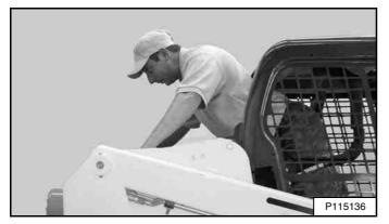
Exit through the rear of the operator cab [Figure 46].
