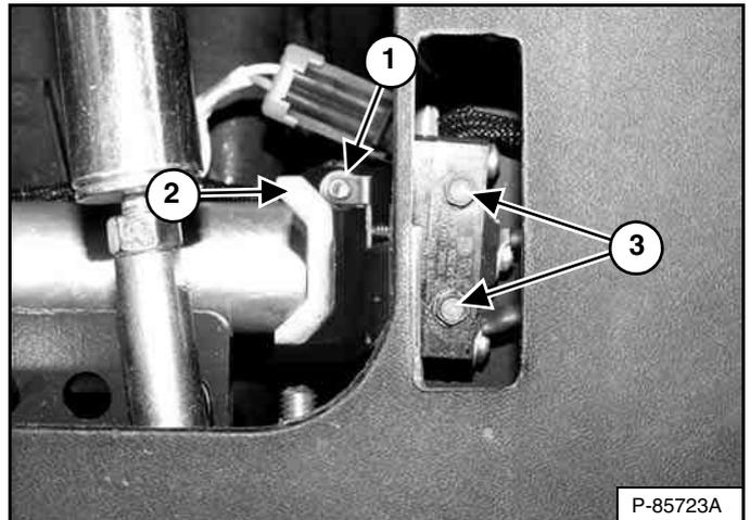
Loosen the screws (Item 3) [Figure 182] securing the back-up alarm switch. (Left side shown)
