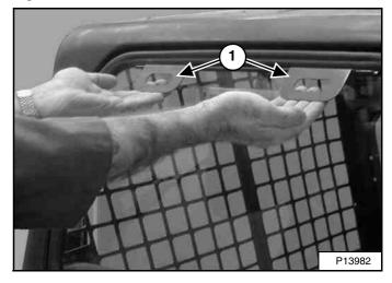
Pull both handles (Item 1) [Figure 51] up and out to remove the rear window.
