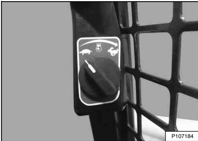
Set the engine speed control to the low idle position [Figure 122].
