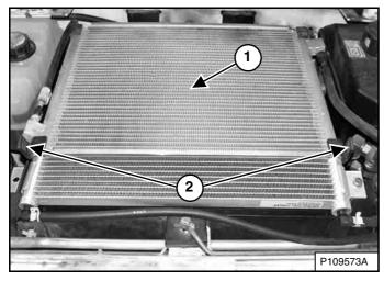
Use low air pressure or water pressure to clean the top of the air conditioning condenser (Item 1) [Figure 222].
