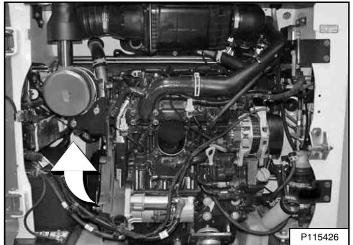
The air conditioning compressor is located behind the engine on the left side of the loader [Figure 293].
