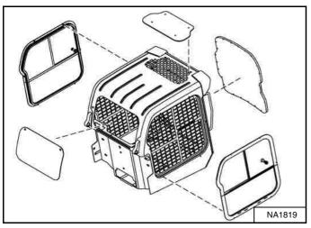
Available for special applications to prevent flying debris and objects from entering the cab. Kit includes 19,1 mm (0.75 in) thick <u>laminated</u> polycarbonate front door, polycarbonate side windows, and polycarbonate rear window **[Figure 5]**.
