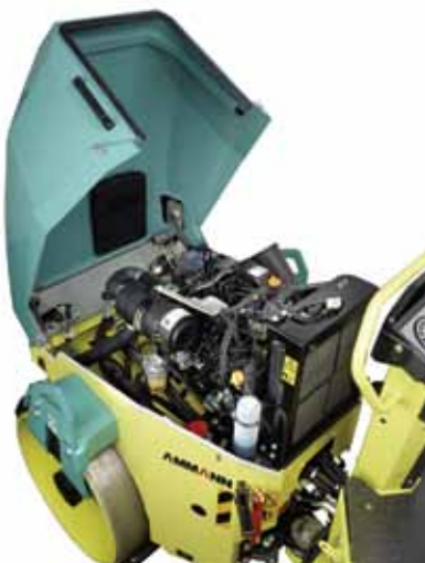
Best service access due to large engine hood
