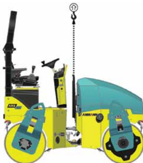
Central lifting point on ARX1(standard) ARX2(option)
