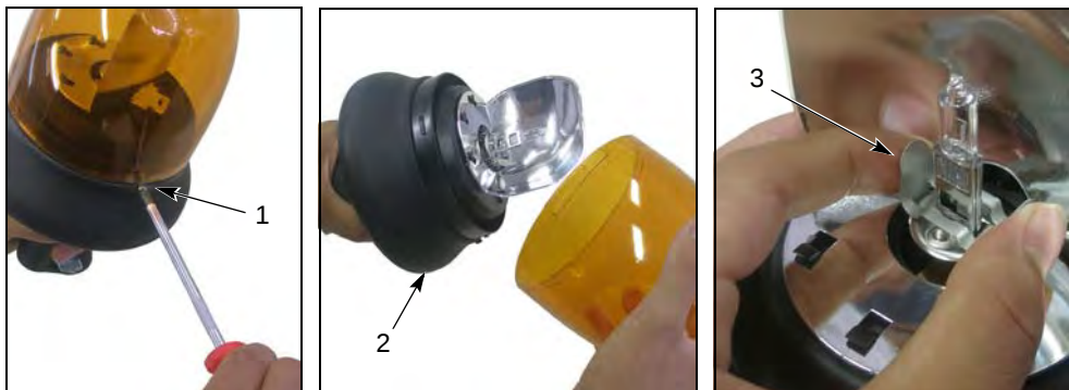
Fig. 8-5 Replacing the bulb
