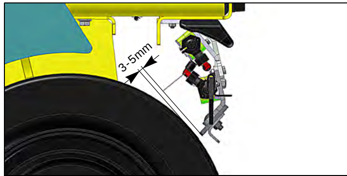
Fig. 9-26 Clearance of scraper to pneumatic wheels
