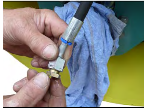
Fig. 9-31 Remove the brake hose and seal it so that it can be pressurized.
