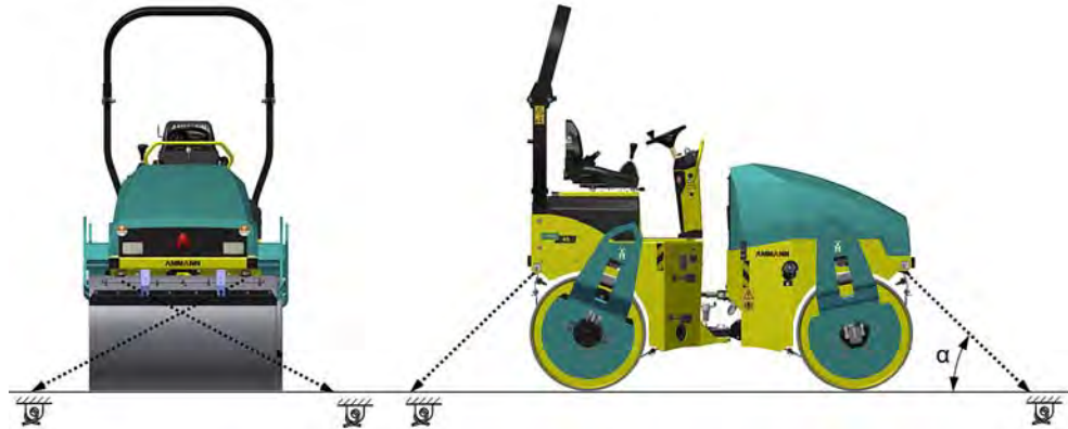
Fig. 12-3 Lashing the roller / side view
