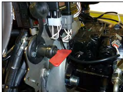
Fig. 8-7 Switching on the power
