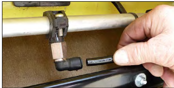
Fig. 11-1 Draining sprinkling water
