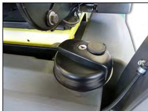
Fig. 7-6 Water tank cover rear right
