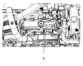
Fig. Engine 1. Type plate
