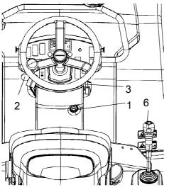
Figure. Instrument panel 1. Starter switch 2. Throttle control 3. Emergency stop 6. Forward/reverse lever
