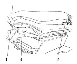
Fig. Driver seat 1. Handle - Length adjustment 2. Handle - Backrest angle 3. Handle - Weight adjustment
