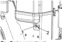
Fig. Engine compartment 1. Battery disconnector 2. Power socket, 12 V
