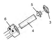
Fig. Hydraulic oil filter 3. Cap 4. Filter insert 5. Handle
