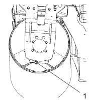
Fig. Drum, vibration side 1. Drain plug
