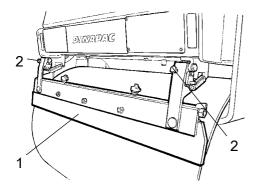
Scrapers, spring-action (Optional) Checking - Adjustment
