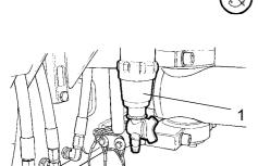
Fig. Pump system 1. Water filter
