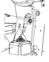
Fig. Driver seat 1. Forward/Reverse lever 2. Attachment screws
