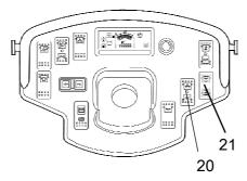
Fig. Instrument panel 20. Man/Auto switch 21. Switch, Vibration selector
