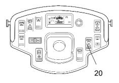
Fig. Instrument panel 20. Vibration switch
