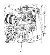
Fig. Left frame side 1. Drain plug
