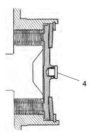
Fig. Brake housing 4. Center plug
