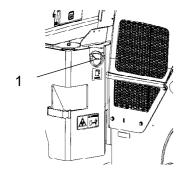
Fig. Fuel tank 1. Filler cap
