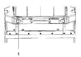
Fig. PIN Front frame 1. Serial number
