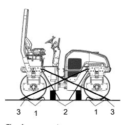
Fig. Arrangement 1. Chocks 2. Wooden blocks 3. Lashing straps
