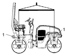
Fig. Lifting the roller 1. Lifting plate
