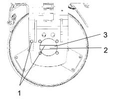
Fig. Left side of drum 1. Brake tool 2. Fastening screw 3. Disengagement nut
