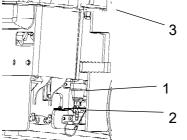
Fig. Pump system 1. Water filter 2. Stop cock 3. Water pump
