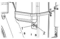
Fig. Battery bay 1. Battery disconnector 2. Power socket, 12 V
