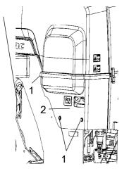
Fig. Engine compartment 1. Retaining screws 2. Protective cover
