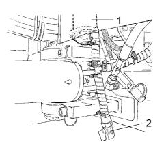
Fig. Pump system 1. Water pump 2. Drain cock
