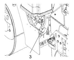
Loosen the red cap (3) and pull up the filter insert (4).
