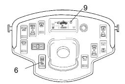
Fig. Instrument panel 6. Parking brake 9. Brake warning lamp Parking brake - Check
