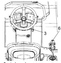
Fig. Control panel 3. Emergency stop 6. Forward/Reverse lever
