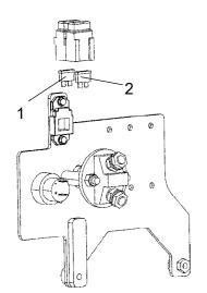
Fig. Battery disconnector
