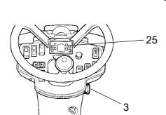
Figure. Instrument panel 3. Emergency stop 25. Parking brake lamp
