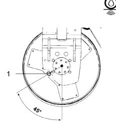
Fig. Drum, drive side 1. Oil plug
