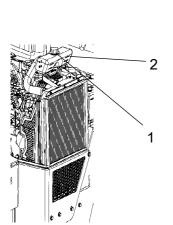
Figure. Cooling water container 1. Filler cap 2. Level marking
