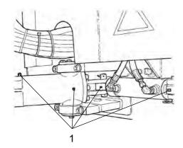
Fig. Main filter 1. Grease nipples
