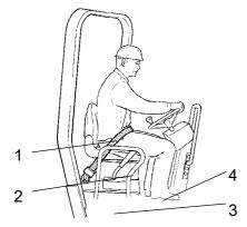
Fig. Driver seat 1. Seat belt 2. Safety rails 3. Rubber element 4. Anti-slip
