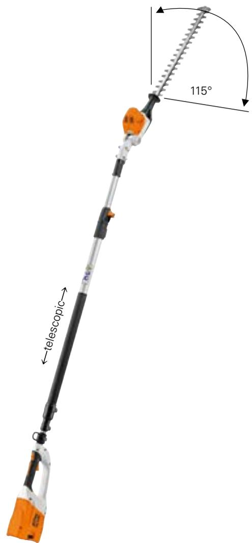
**2 HLA 85 // Battery long-reach hedge trimmer with high cutting performance for particularly high hedges.** Telescopic shaft with tool-free, quick-release tensioner (total length of 260 to 330 cm), double-sided cutting blades, cutter bar adjustable through 115°, ideal adjustment for overhead, vertical and floor cutting.
