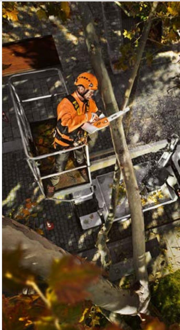
1 MSA 160 T // Very lightweight battery arborist saw for professional work in noise-sensitive areas. Captive nut on the sprocket cover, side chain tensioning, PM3 1/4" saw chain as standard for a clean cut and good cutting performance.
