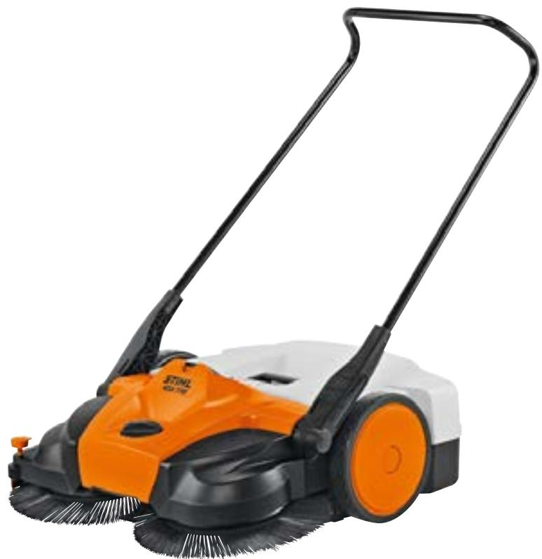
**KGA 770 // Battery sweeping machine for working on large areas both indoors and outdoors.** STIHL MultiClean PLUS sweeping system, 8-level central height adjustment, ergonomically shaped push bar, side guide roller, transport handle, can be stored upright to save space, 4-year warranty on the low-wear nylon bristles. (Battery operation only applies for circular brushes and power sweep.)
