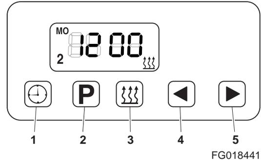
**Figure 12** Engine Coolant Heater Digital Switch
