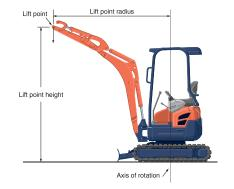
Machine with ROPS canopy and rubber crawler, without bucket
