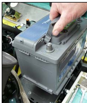
Fig. 10-2 Replacing the battery
